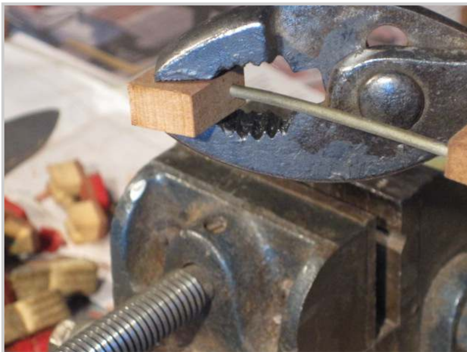
Photo 501: A pair of pliers is used to pop the damper block off cleanly from the damper head. Ordinarily, no steaming is required for this step.
