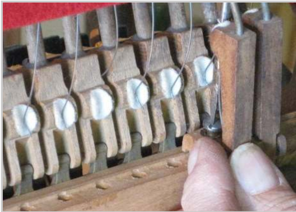
Photo 507: Once new felt is in place, damper levers are screwed back onto the main action rail.
