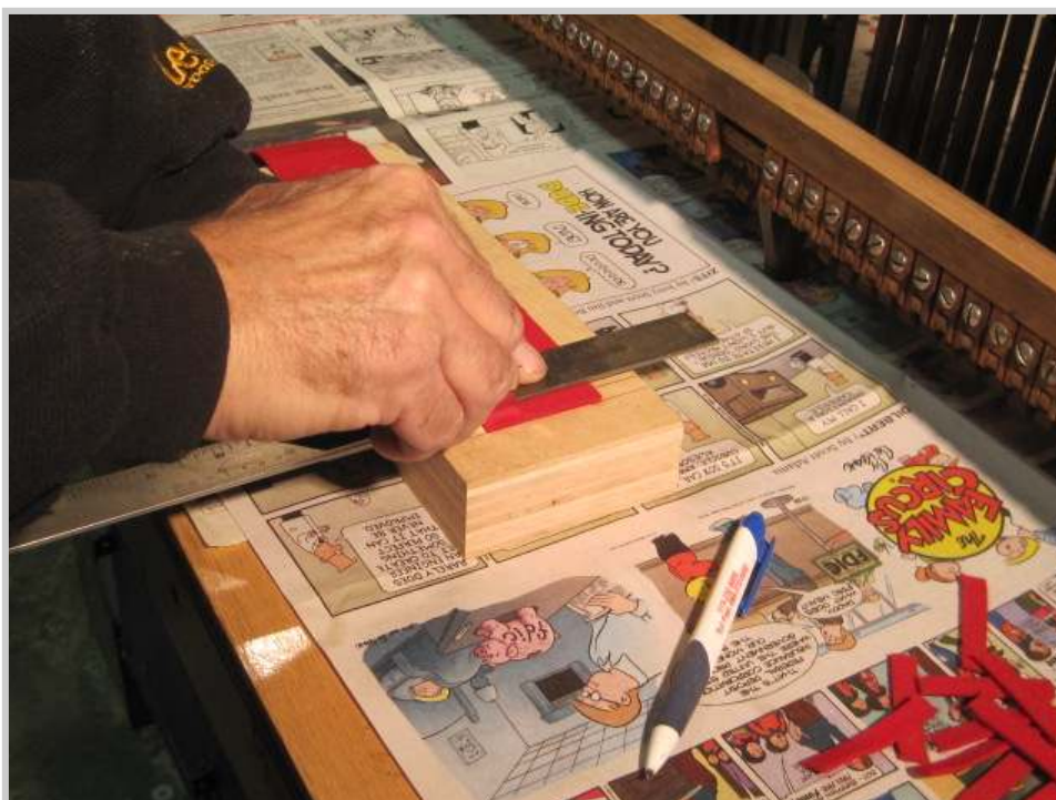
Photo 504: New felt for the damper levers is cut from a strip of felt with the same thickness as the original.
