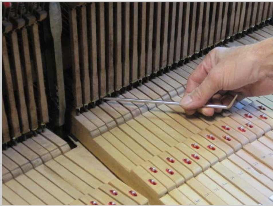
Photo 513: With the action complete, the regulation process is completed. In this step, lost motion is taken up to prevent a sloppy feel.
