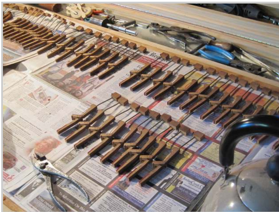
Photo 502: The damper assemblies minus the actual damper felts and damper heads are lined up in order. Because of variations in the bends of the damper wires, each assembly is returned to its original position, reducing the amount of adjustment that will need to be made upon the installation of the action back into the piano.
