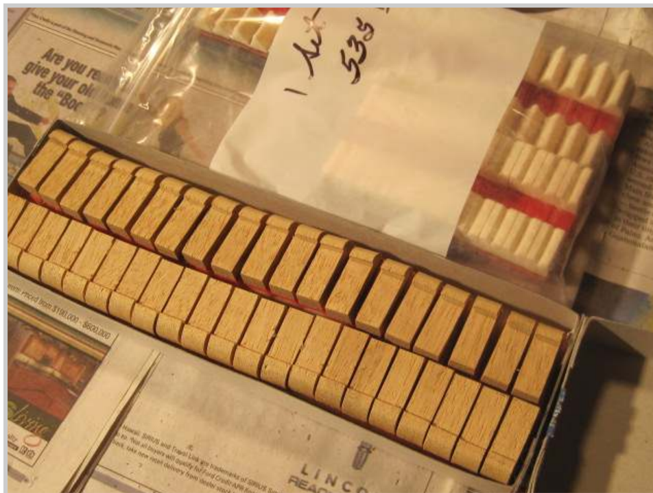
Photo 509: New sets of treble and bass dampers, ready for installation. The treble damper heads, with damper felts attached, are graduated in size, with the largest damper to be placed on the left side of the treble dampers.
