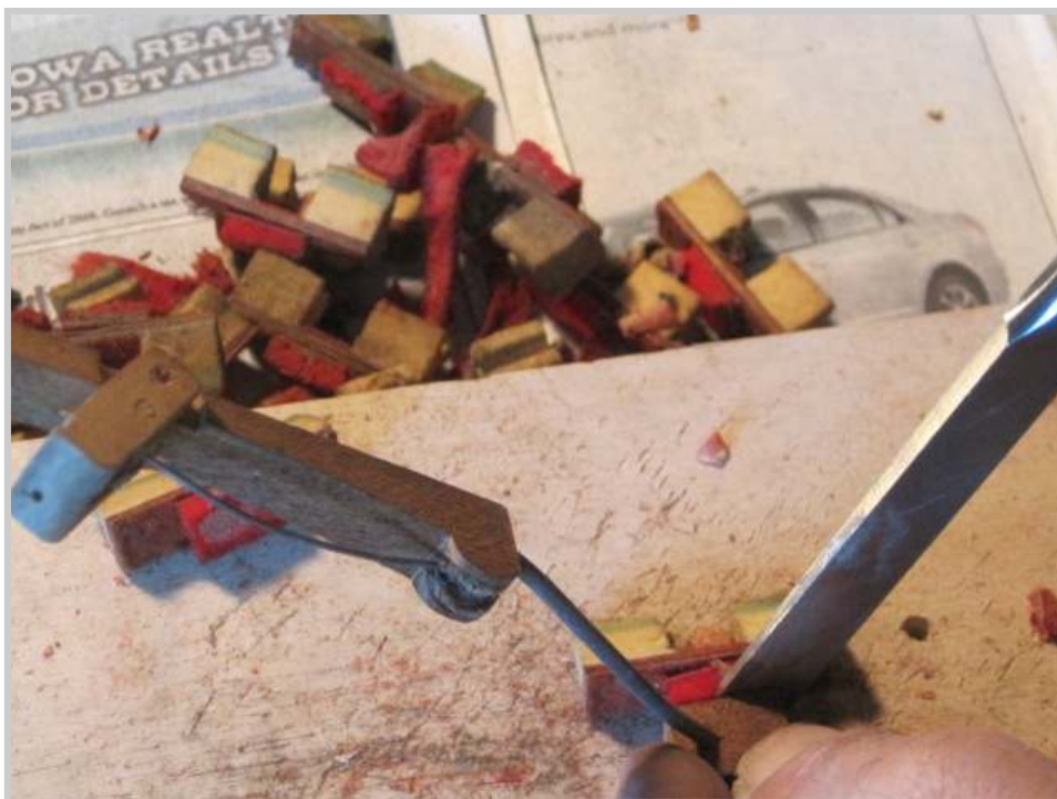
Photo 499: The dampers and damper levers are now due to be worked on. The first step is the removal of the old dampers from their damper blocks. Bass dampers are removed with a chisel and discarded. The original wooden damper blocks will be retained.
