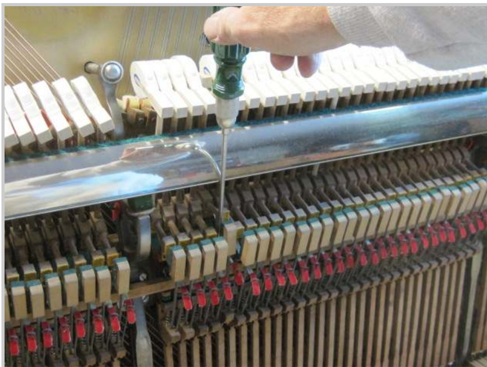
Photo 514: Let off is adjusted so that hammers escape at approximately 1/8th of an inch from the strings.
