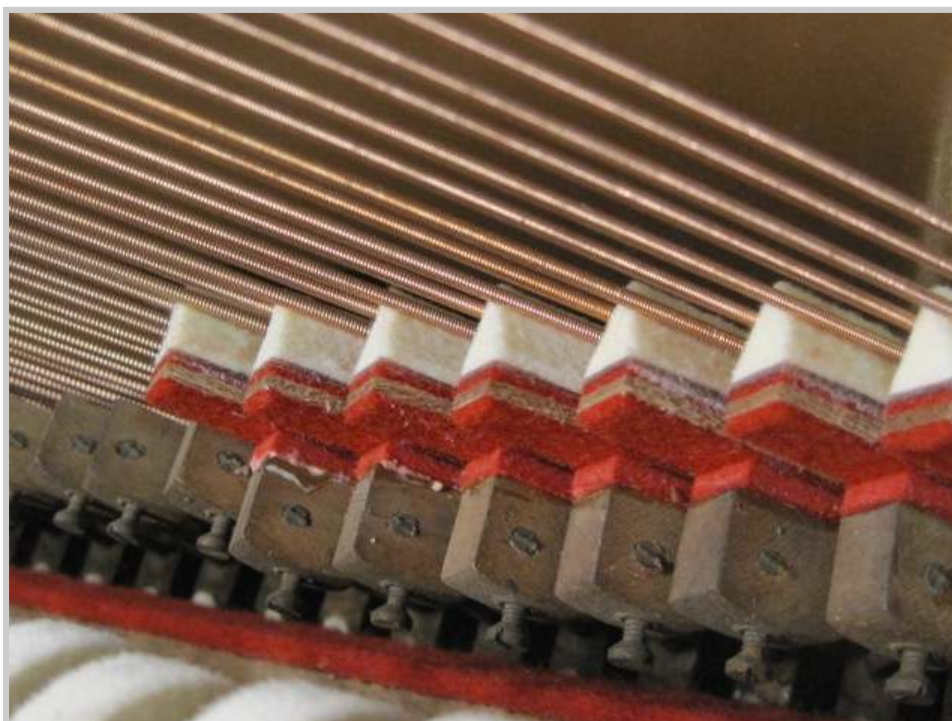
Photo 512: The process of fitting and gluing the bass dampers is begun. The double string wedges are adjusted to make contact with both strings at exactly the same moment.
