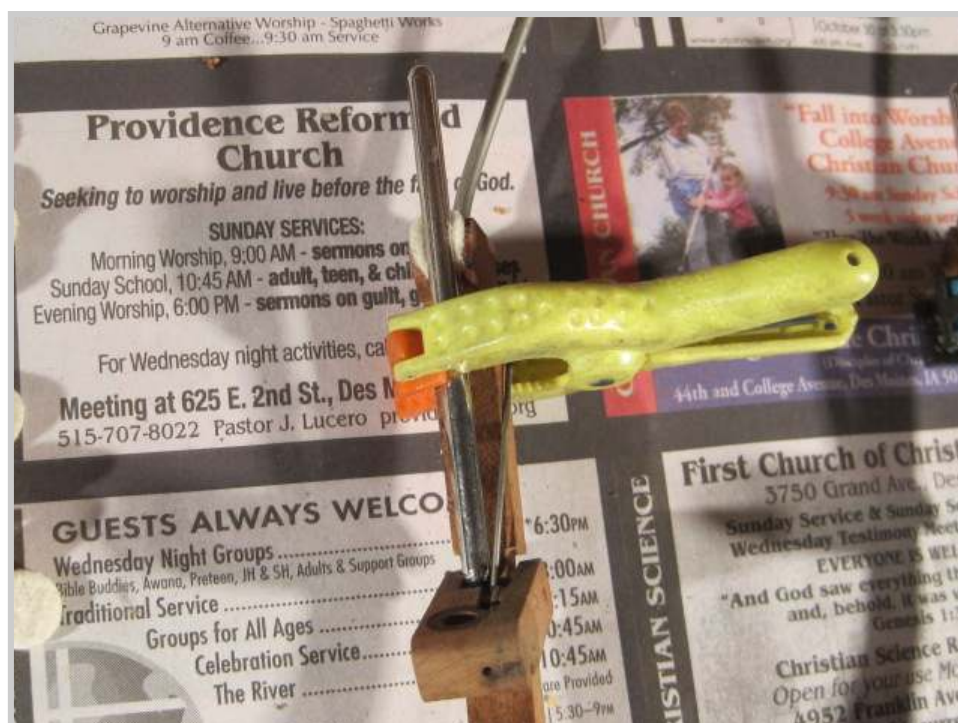
Photo 506: Spring punchings are glued with hot glue. A balance rail pin is of the right diameter to be used as a form while the glue cures.
