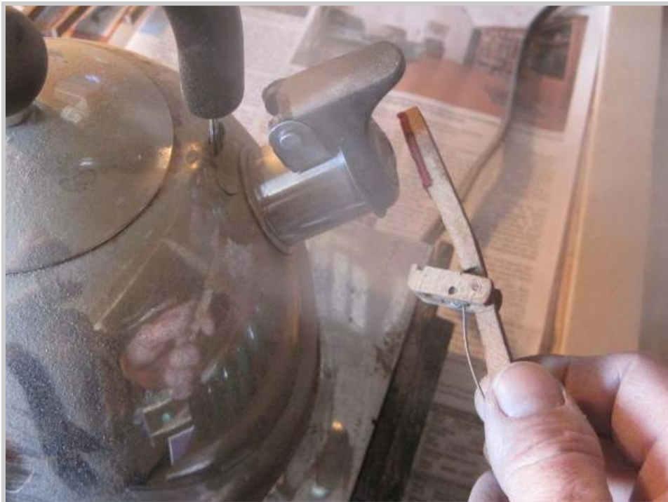
Photo 503: The damper lever felt and spring punchings are next removed from each assembly. The felt is first steamed, then chiseled off.
