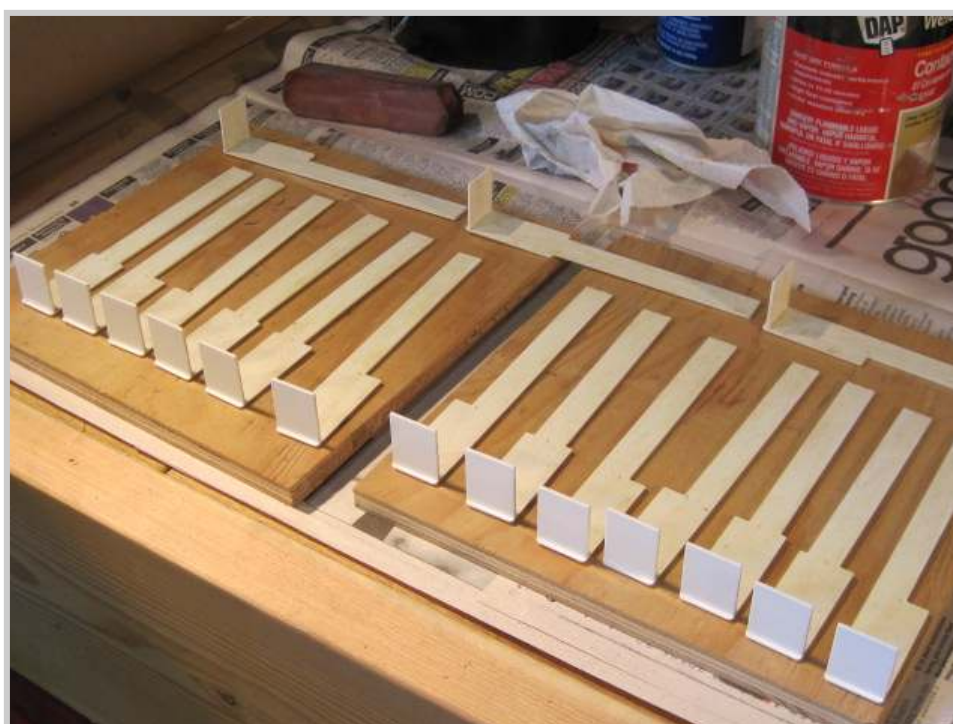
Photo 474: Molded keytops with fronts are placed in order on a drying rack to dry until tacky to the touch.
