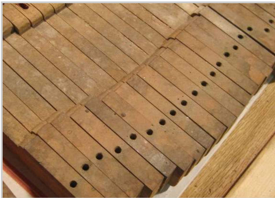
Photo 444: Without the capstans in place, the riser at the backs of the keysticks may now be sanded to eliminate the final reminders of the mouse colony.
