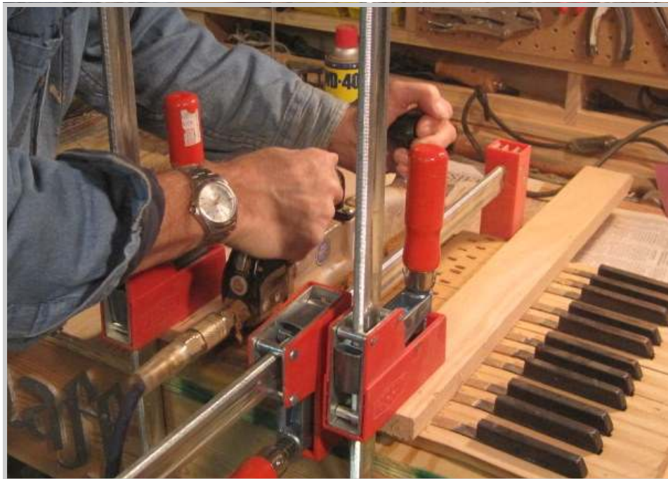
Photo 447: With the keys clamped firmly in place on the bench, the area of the keysticks in between the key buttons and the back riser are initially prepped with an inline pneumatic sander.
