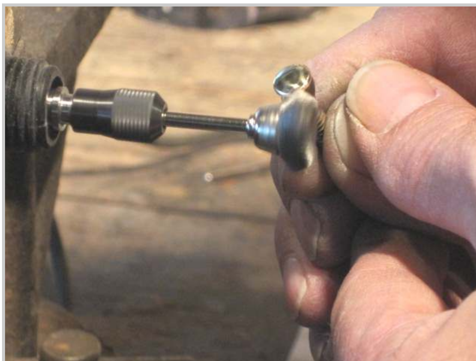
Photo 468: The wings of the capstan are cleaned on a micro wire wheel used on a Dremel tool. Again, the speed of the wheel is set on the lowest possible setting
