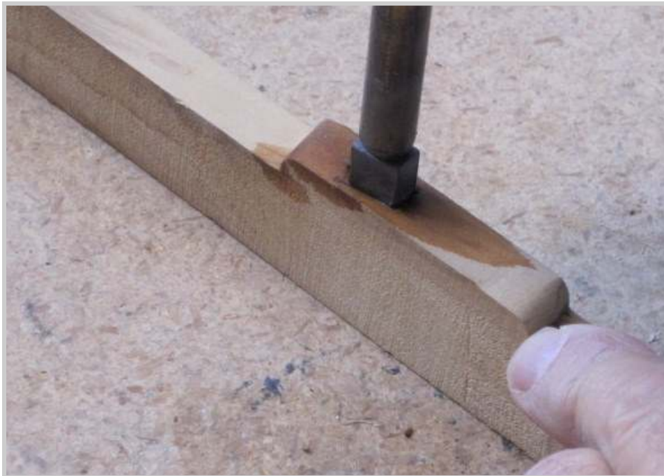
Photo 451: If the old bushing felt does not readily come out after moistening, an electric key bushing removal tool is inserted into the mortise to further loosen the glue holding the felt in place.
