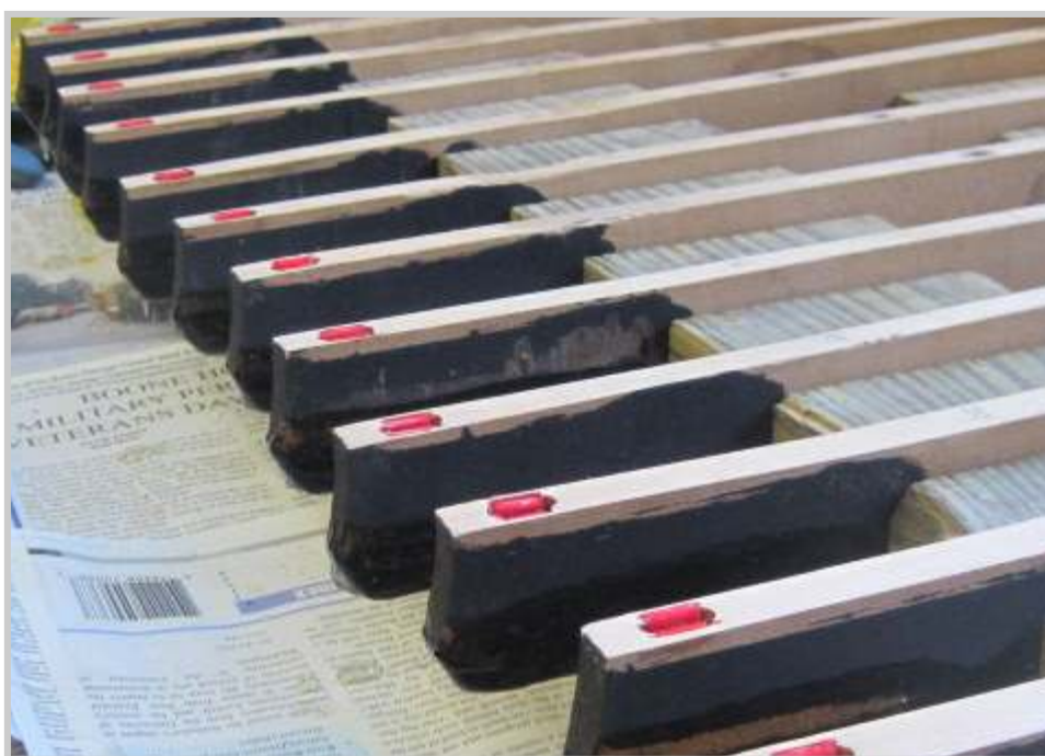
Photo 487: Removing the old lacquer is the first step, no matter what course of action is taken in refinishing the sharps. Here, a thick coat of stripper is applied.
