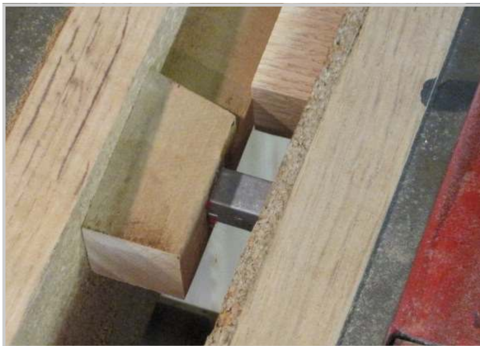
Photo 457: Once the caul is inserted and the bushing felt is trimmed, the key is placed in the vise for a short time to insure that the felt adheres to the shoulder of the mortise.
