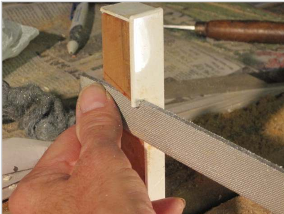
Photo 481: The first cut for the notches are made with a coarse file used on edge. The cut is stopped just short of the line.
