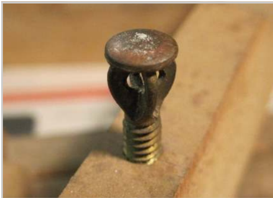
Photo 442: The effects of time on brass are seen clearly in this photo. The problem with this is that the upper surface of the capstan should be slippery smooth to eliminate friction. These capstans will in short order be polished to a mirror finish.
