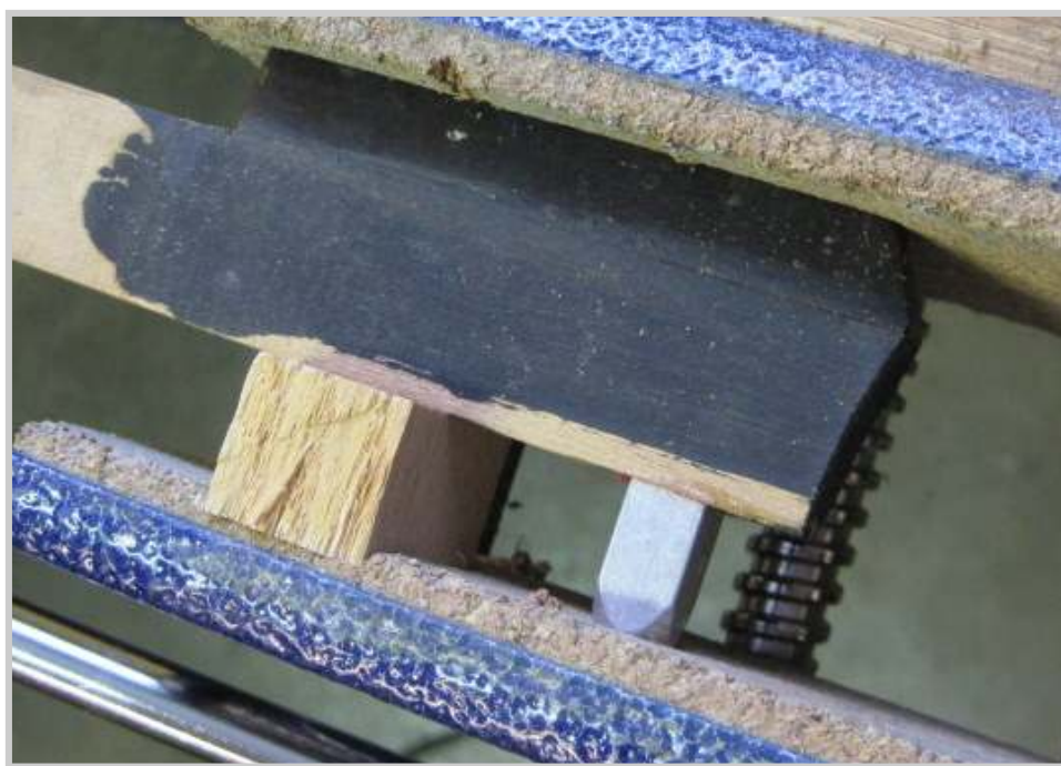
Photo 458: The wooden block on the left keeps the caul at a 90 degree angle.
