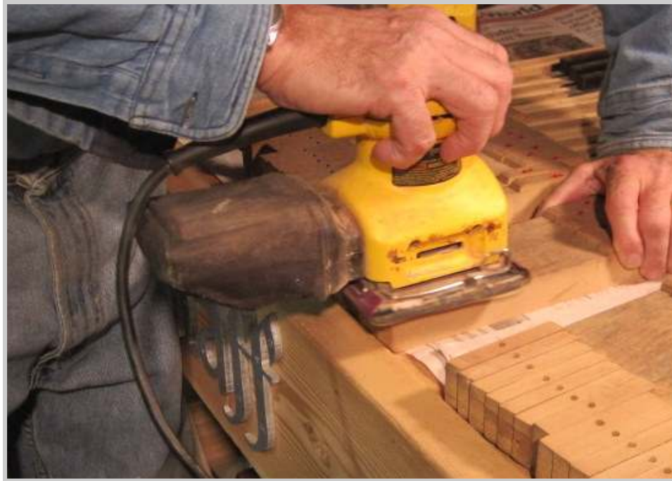
Photo 445: A small sander equipped with 150 grit paper, followed by 220 grit, does the job nicely.
