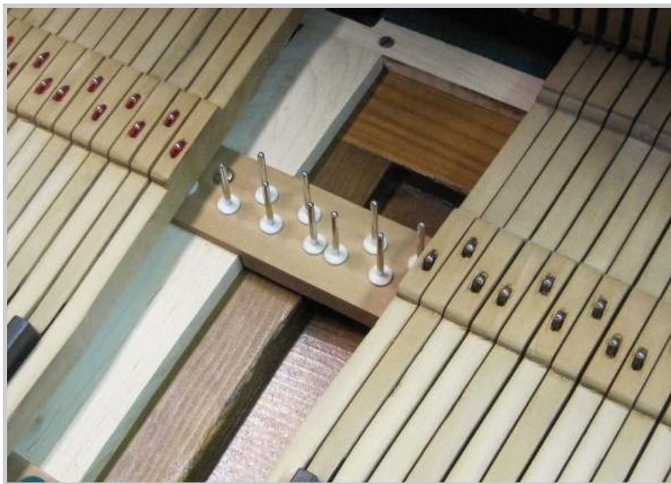
Photo 464: Work progresses from left to right. Keys on the left have new bushings installed. Missing keys in the center are being worked on. Keys on right are waiting their turn.
