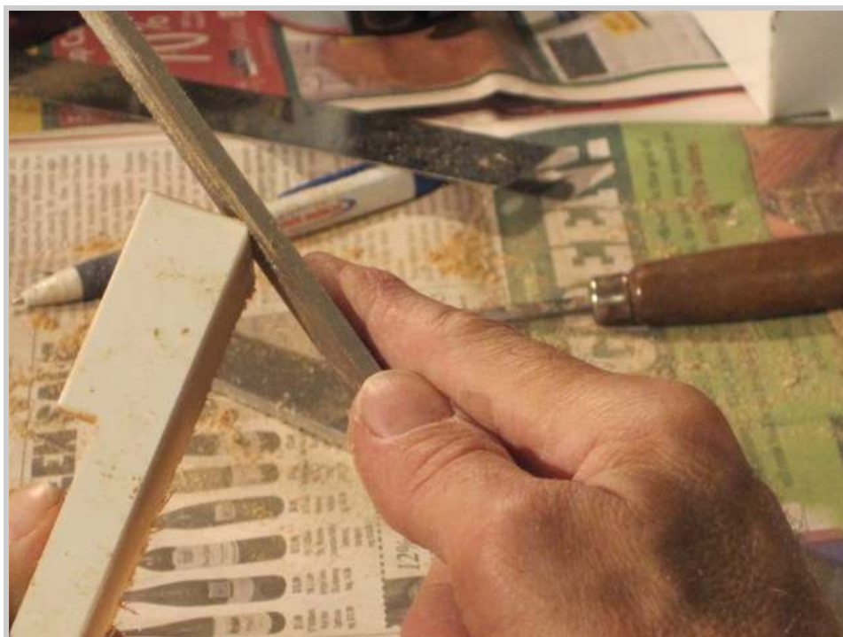
Photo 484: The corners of the overhang of each key are given a slight curve, and the sides of the keytop are slightly rounded to give softer edges which are easier on the fingers of the pianist.
