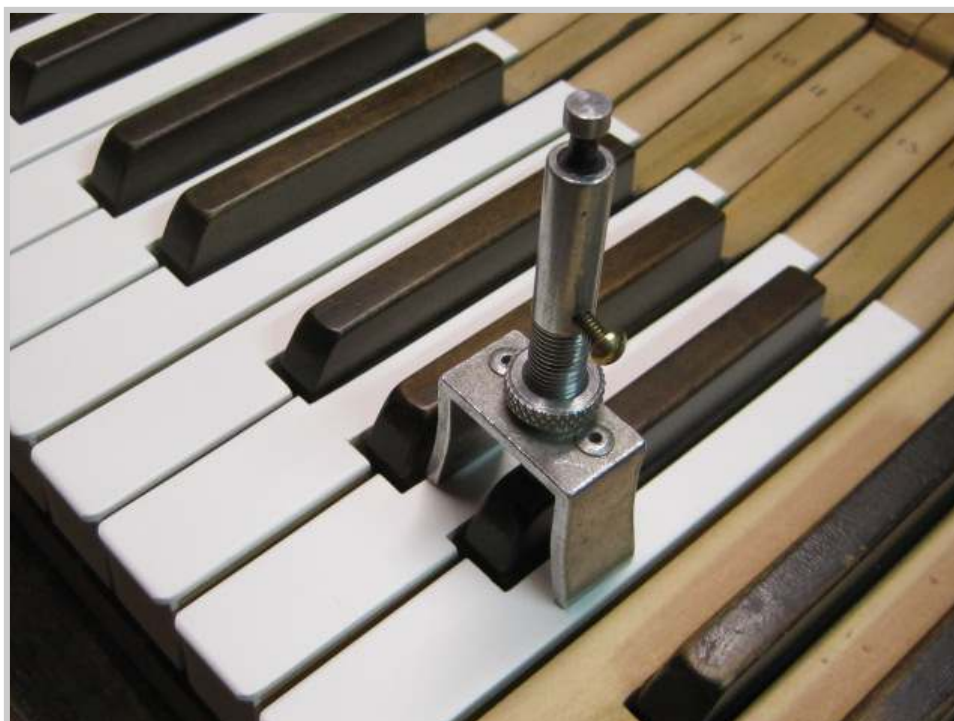
Photo 496: The sharp keys are leveled 1/2" above the naturals.
