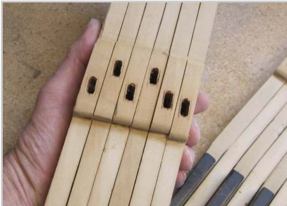
Photo 453: The key buttons, without bushings, having now been dried out over-night. The mortise for the front rail bushings have also been cleaned of the old felt and allowed to dry.
