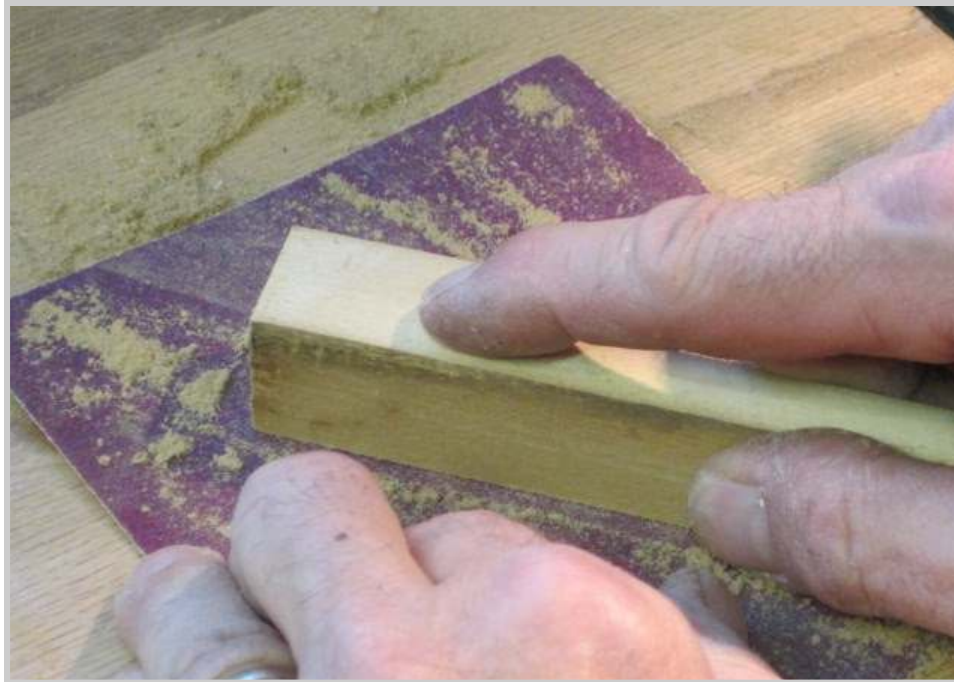
Photo 459: Once the glue has been allowed to cure, the bottoms of the keys, and the tops of the key buttons, are sanded to remove any wayward glue.
