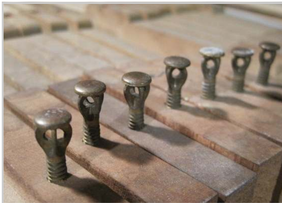
Photo 441: The first order of business concerns the brass capstans at the back of each keystick. These are especially important in that they serve as the point of contact between the key and the lower part of the action.
