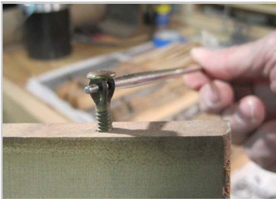
Photo 443: For the time being, the complete set of capstans are removed by backing them out with a regulating tool. They will be set aside and returned to the key after several intervening steps have been accomplished.
