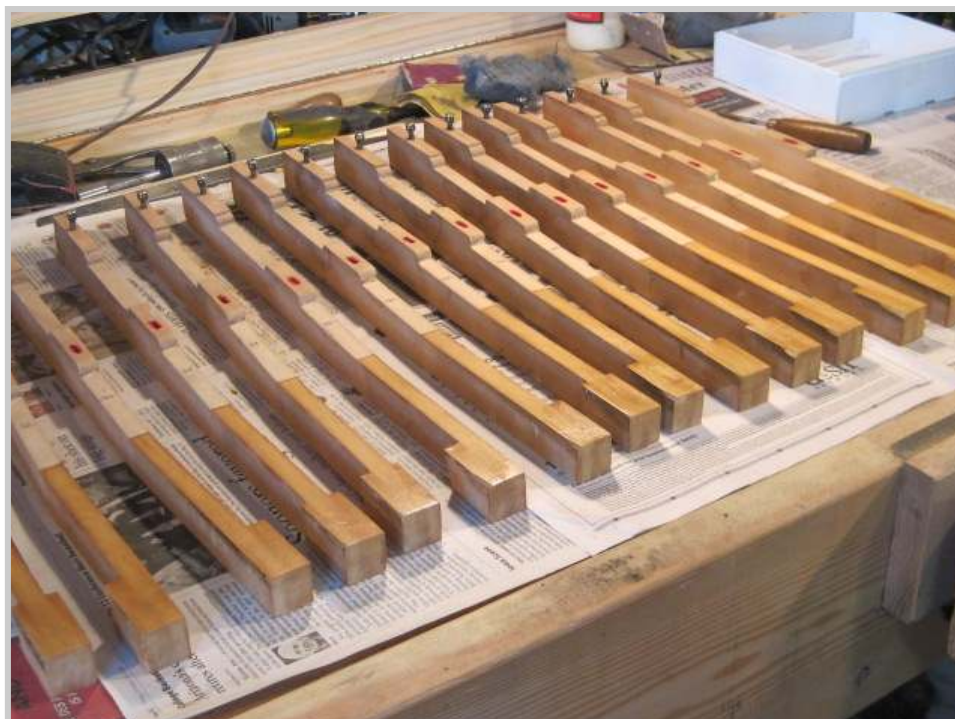
Photo 471: Recovering the naturals is the next step. Opinion is divided over the best adhesive to use. My glue of choice is contact cement. I coat the wood, let it dry, then coat it a second time.
