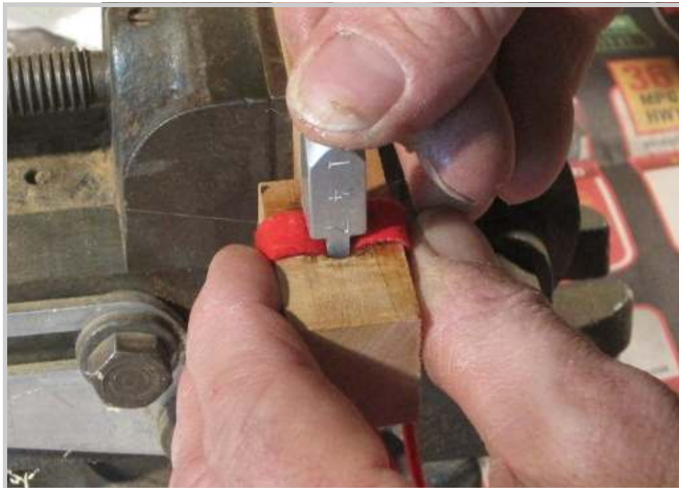
Photo 455: The proper thickness of felt and the proper caul size have been selected. Hot glue is applied to the inside of the mortises, and the correct length of felt inserted. The heated caul is then pushed into place.
