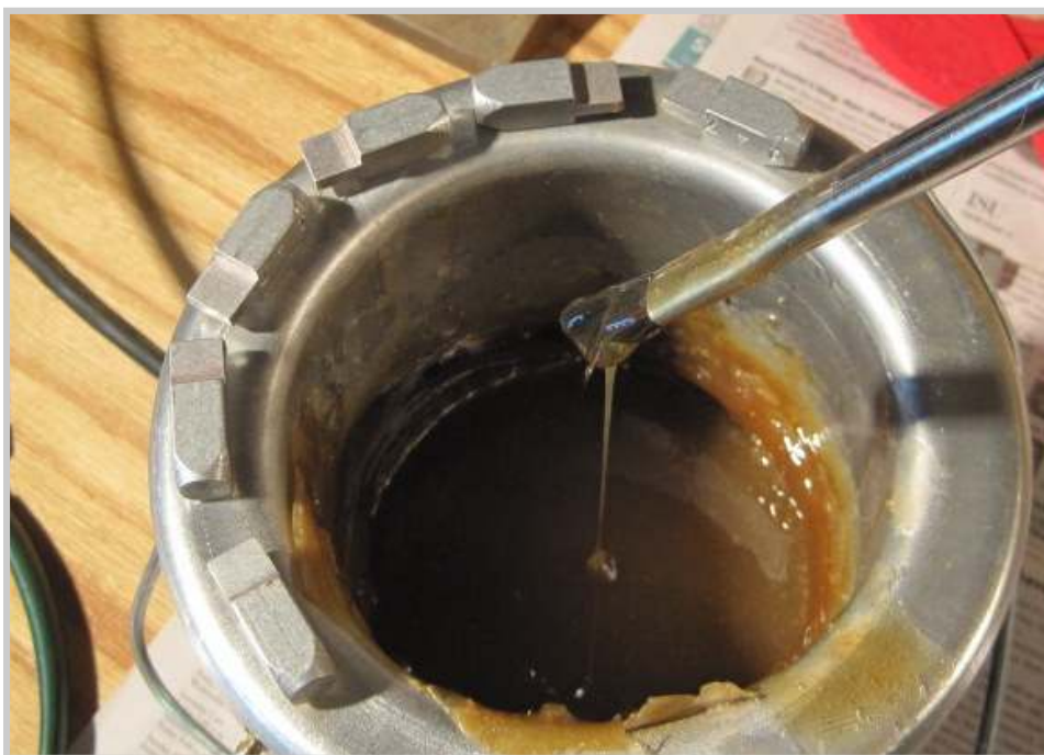
Photo 454: Hot hide glue is again the glue of choice. Aluminum bushing cauls are heated on the side of the glue pot in readiness for insertion.
