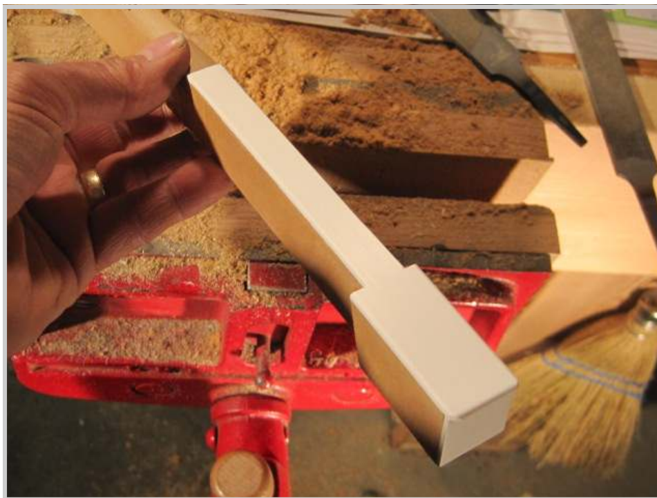
Photo 485: A completed keytop. The final optional step of buffing with 0000 steel wool gives it a texture more like ivory, less slippery than plastic.
