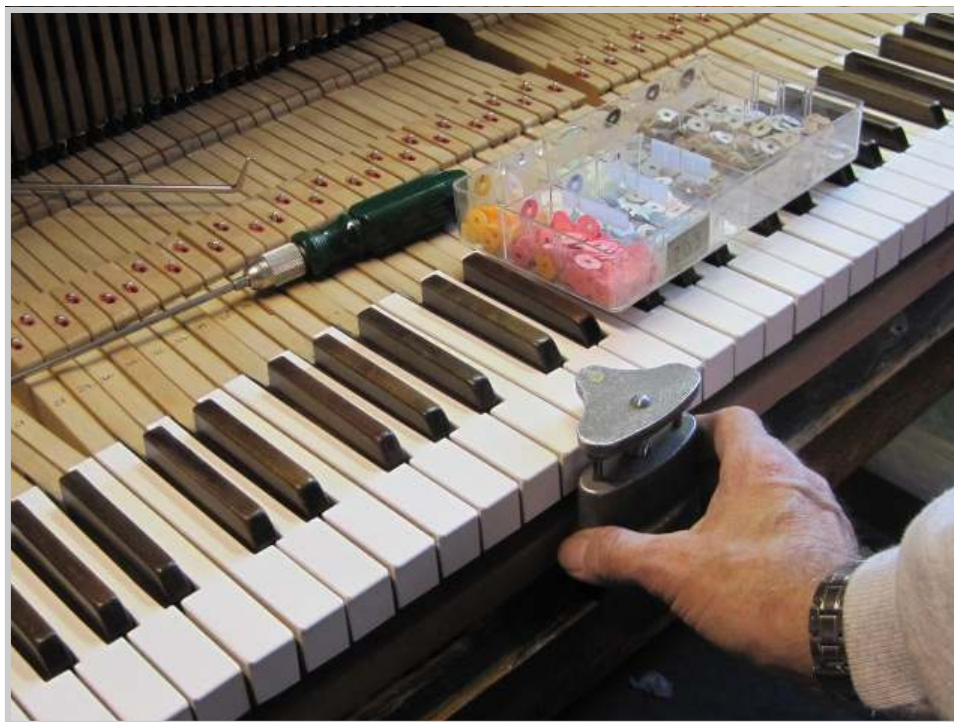
Photo 495: With a key leveling device, the naturals are brought up to the level of the highest key. Leveling papers as fine as .001" are used to produce a perfectly level set of keys.
