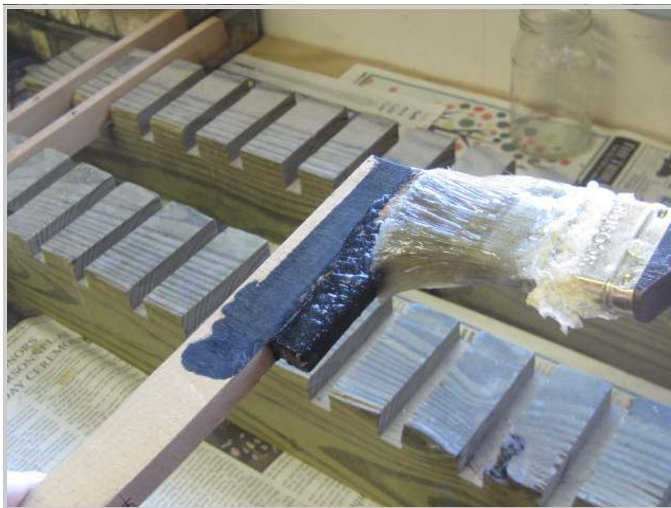
Photo 487: Removing the old lacquer is the first step, no matter what course of action is taken in refinishing the sharps. Here, a thick coat of stripper is applied.
