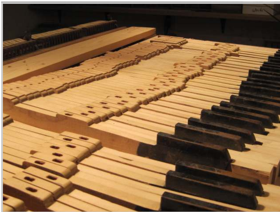
Photo 449: The set of keysticks with top surfaces sanded. Remaining staining on the sides of the keysticks will be dealt with in a later stage.
