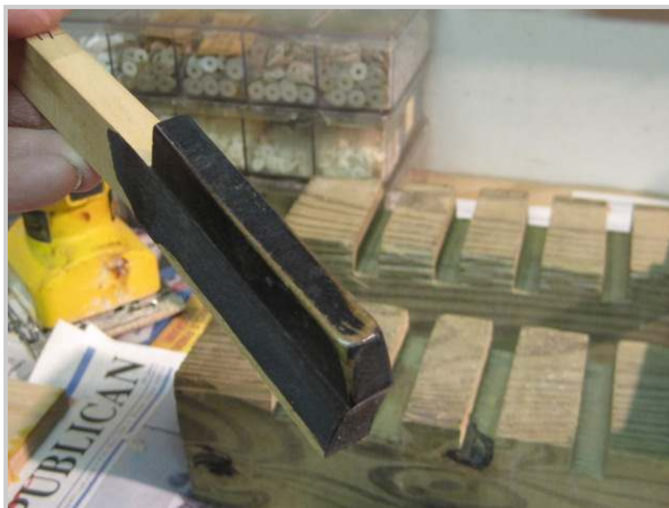
Photo 486: An unfinished sharp. These sharps are made from ebony wood which was painted originally with a black lacquer. The ebony itself is a beautiful wood, and oftentimes looks more attractive without an opaque coating. Again, there are optional approaches to the refinishing of the sharps.
