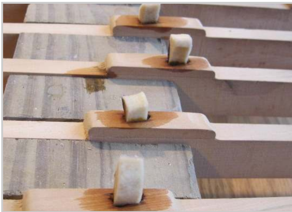
Photo 450: Old key bushings are now removed. The first step is to dampen the old felt with wedges of hammer felt.
