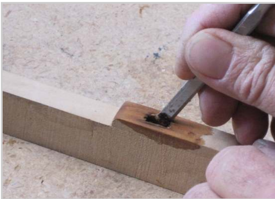
Photo 452: In a few cases, reluctant bushings must be scrapped away with a small chisel.
