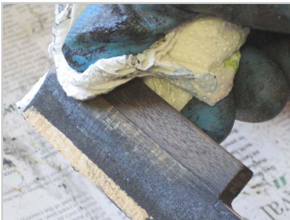
Photo 489: Once the lacquer has been softened by the stripper it is scrubbed with #3 steel wool. If a second treatment seems necessary, more stripper is brushed on and the key is returned to the rack for a short time.
