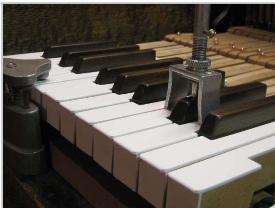
Photo 440: As the naturals and sharps are completed, they are returned a final time to the keyframe to be leveled.
