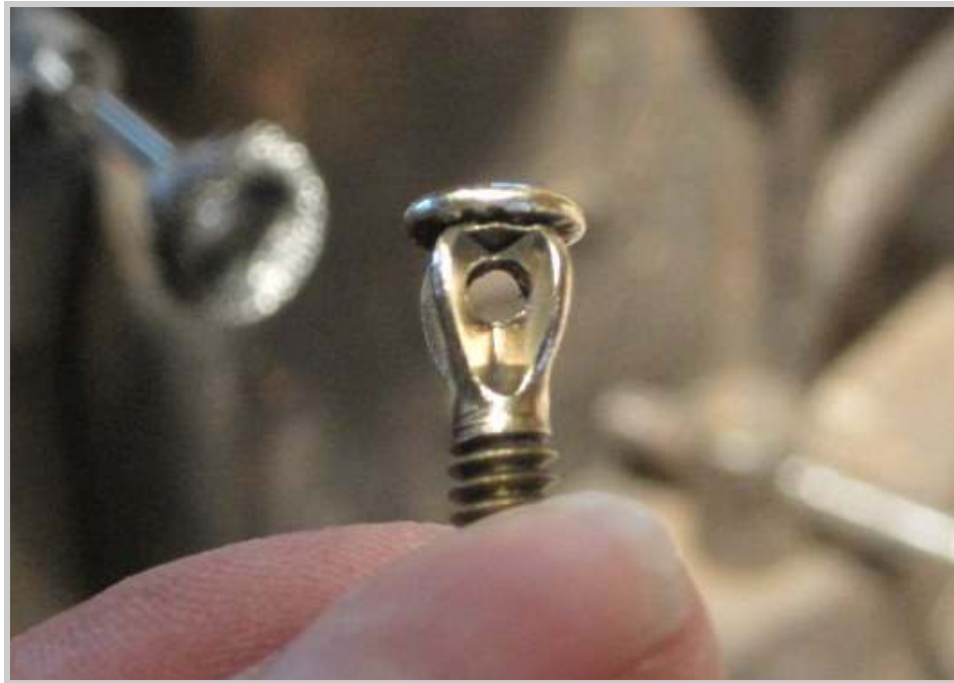
Photo 469: The capstan thus cleaned is ready to be replaced into the riser at the back of the keystick.
