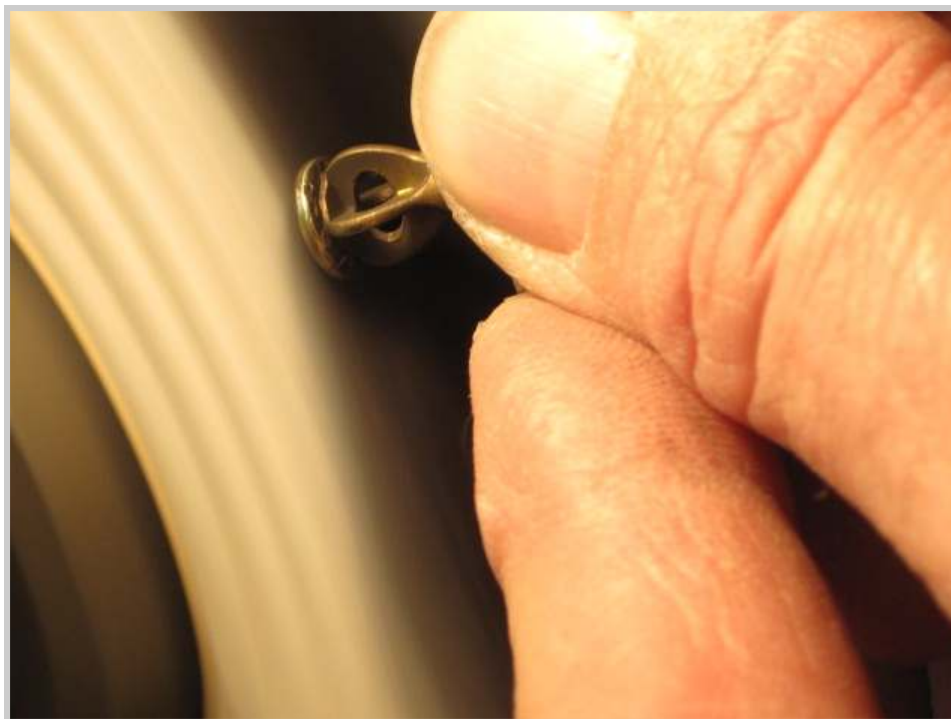
Photo 467: With the wheel turning at its lowest speed, the head of each capstan is polished. The effects of nearly a century of exposure to the air melt away.
