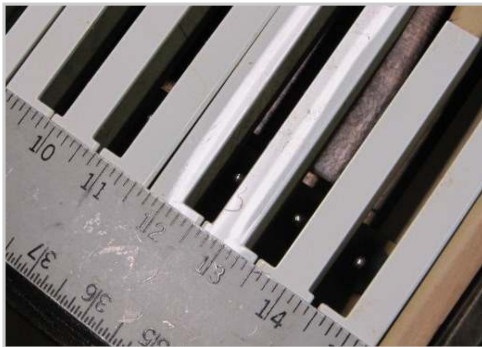
Photo 477: The overlong front of the key is ground down on a grindstone set at a slow rotational rate.
