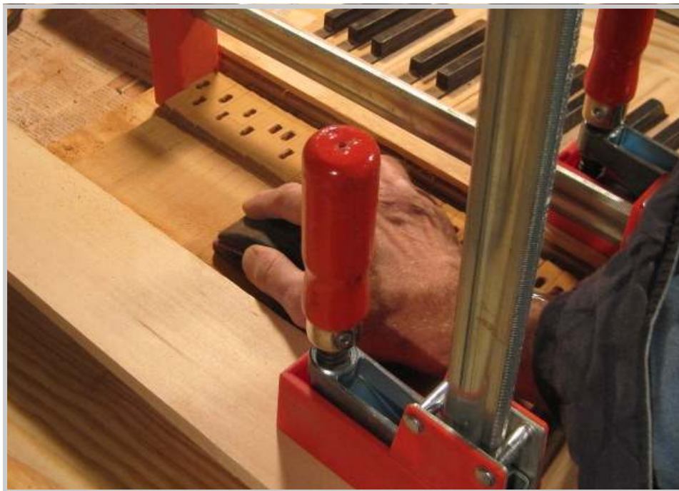
Photo 448: To eliminate side-to-side sanding marks left by the air tool, each section is hand sanded with grades progressing down to 600 grit paper.
