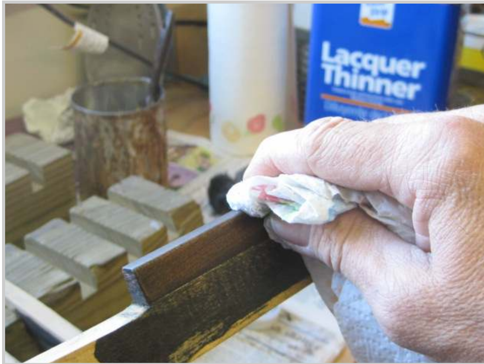
Photo 491: Final cleaning is done with a paper towel dowsed in lacquer thinner. The sharp is then allowed to dry.
