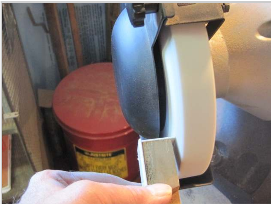
Photo 477: The overlong front of the key is ground down on a grindstone set at a slow rotational rate.
