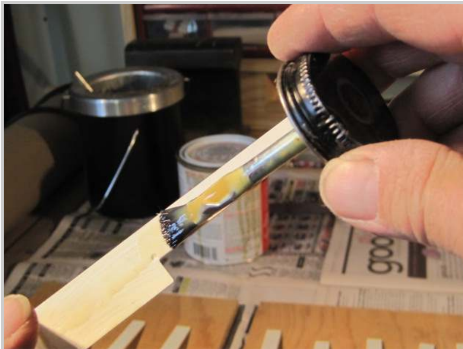
Photo 473: Coating the inside of the molded keytops is the only tricky part in the process. The glue must not be allowed to touch the playing surface of the keytop.
