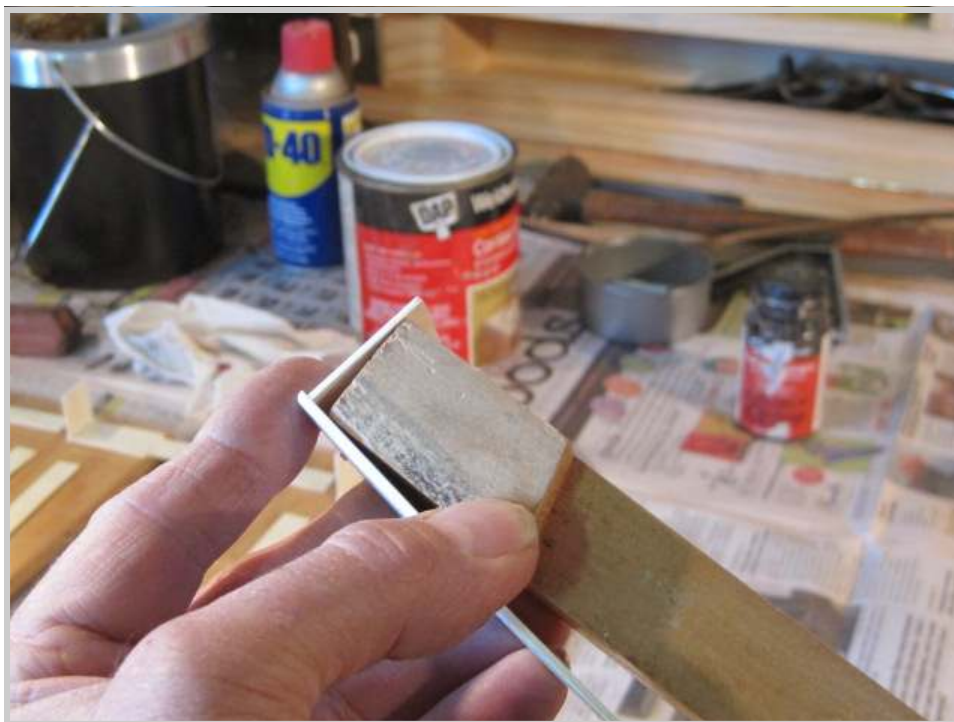
Photo 475: The keystick and keytop are carefully joined together by folding the keytop down over the wooden keystick.
