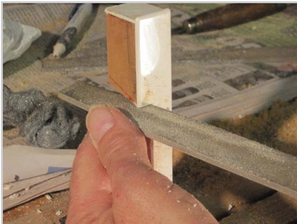
Photo 482: The notch is finished with a fine file, using the wide, flat side of the file to carefully cut out the rest of the unneeded material. A perfect 90 degree cut-out is the goal.
