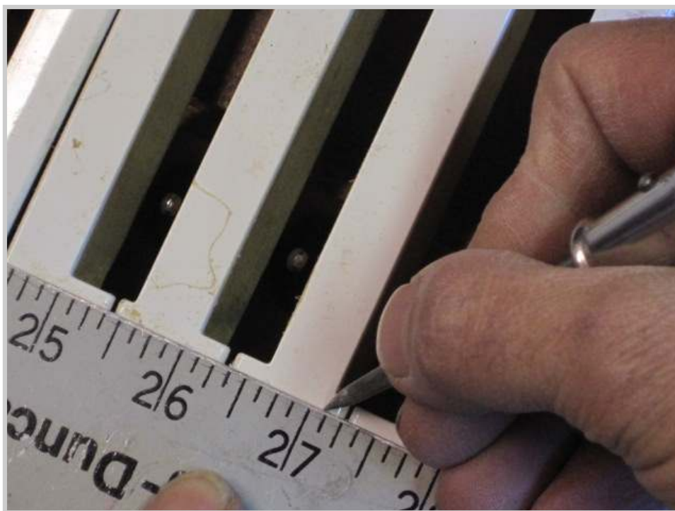
Photo 480: With the straightedge clamped down on either side of the keybed, the keys are pushed up from underneath against the ruler firmly with the fingers of one hand, while a sharp scratch awl is used with the other hand to scribe the keys for notching. Care is taken only to scribe the portion of each key actually to be notched.
