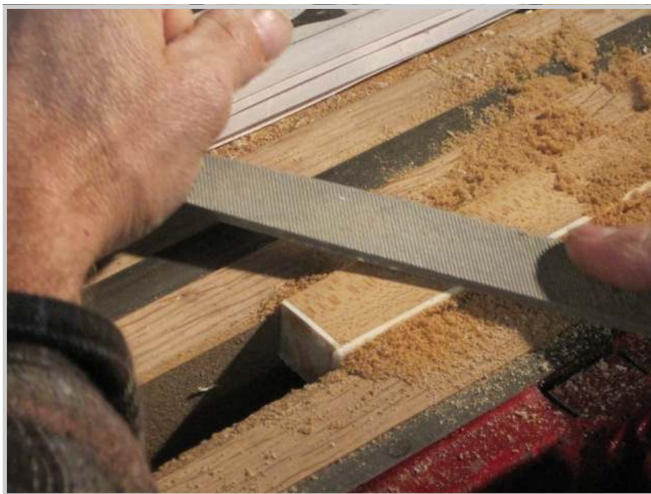
Photo 483: Using first the coarse file, and then the fine one, each key is filed flush with the keystick on either side.
