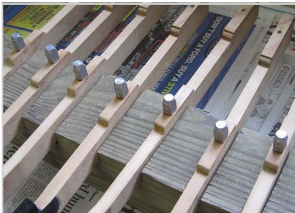
Photo 462: With the cauls for the balance rail bushings in place, the keysticks are placed in the holder for the hide glue to cure.
