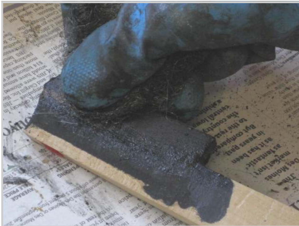
Photo 489: Once the lacquer has been softened by the stripper it is scrubbed with #3 steel wool. If a second treatment seems necessary, more stripper is brushed on and the key is returned to the rack for a short time.
