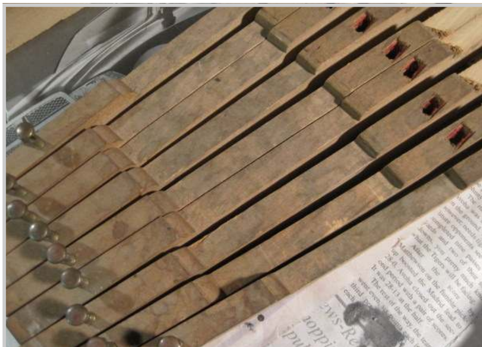
Photo 439: At last, I'm ready to turn my attention to the keys. Apart from trimming the keysticks on the table saw in preparation for new molded keytops, and burying the entire set of keys for weeks in baking soda to eliminate mouse odor, they have not been touched. Obviously, from the looks of them.
