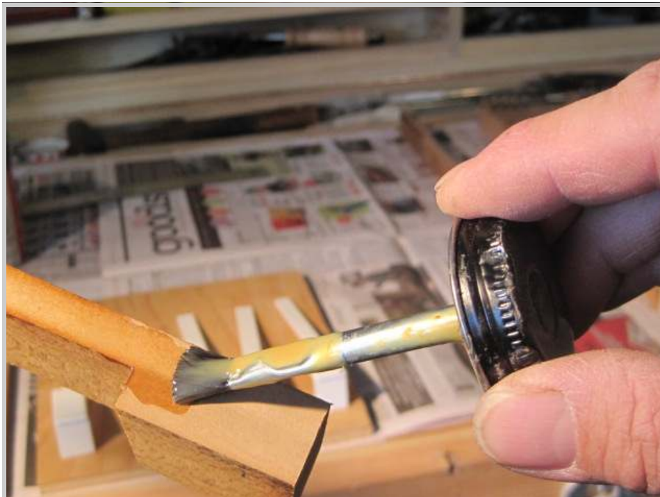
Photo 471: Recovering the naturals is the next step. Opinion is divided over the best adhesive to use. My glue of choice is contact cement. I coat the wood, let it dry, then coat it a second time.
