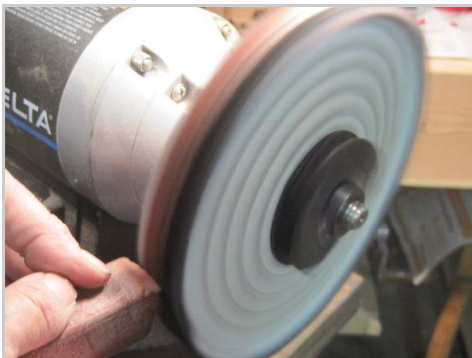
Photo 466: The buffing wheel is loaded with Red Tripoli polish.
