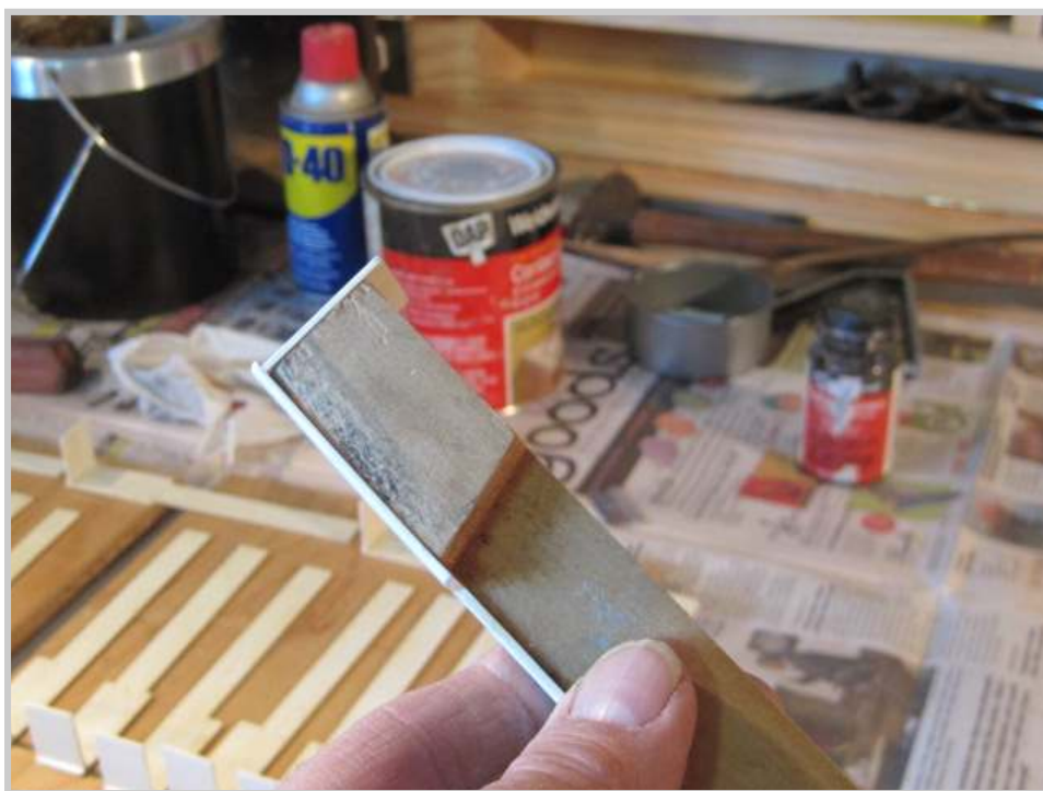
Photo 476: The bond between the two components of the key is formed immediately upon contact. Any adjustment at this point is very difficult. Each key is clamped down in a vise with cork facings for a few moments to strengthen the bond.
