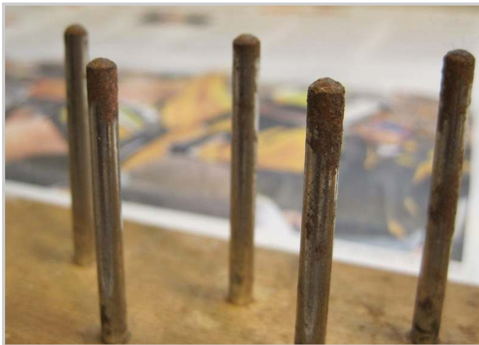
Photo 323: Examination of the balance rail pins reveals corrosion too deep to simply polish out. Removal of the old pins and replacement with new is necessary.
