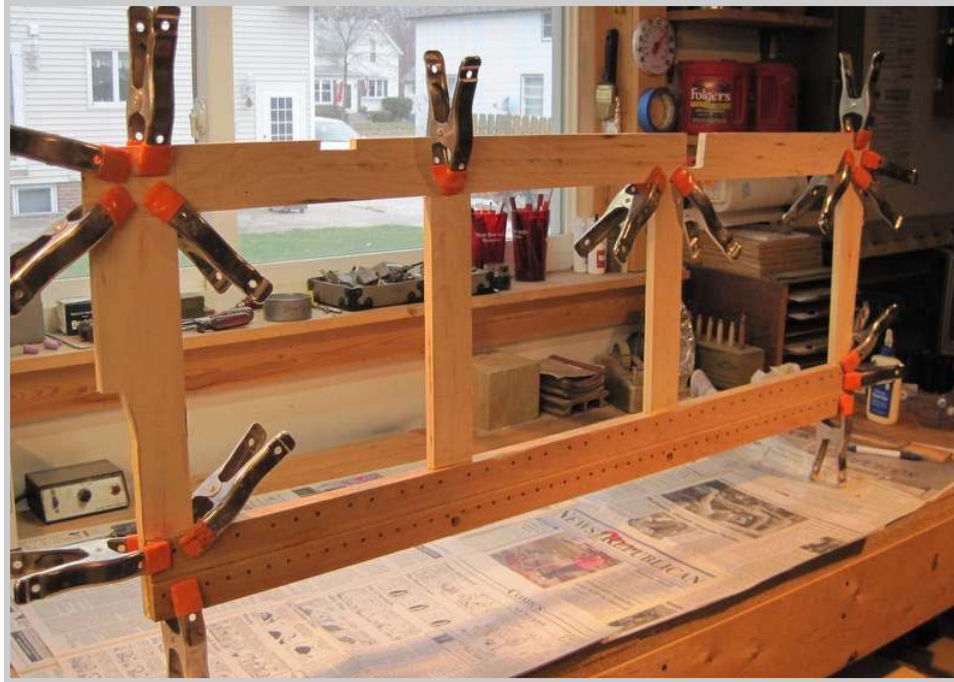
Photo 341: With all the joints fitted and glued, the keyframe is clamped together and allowed to dry overnight.
