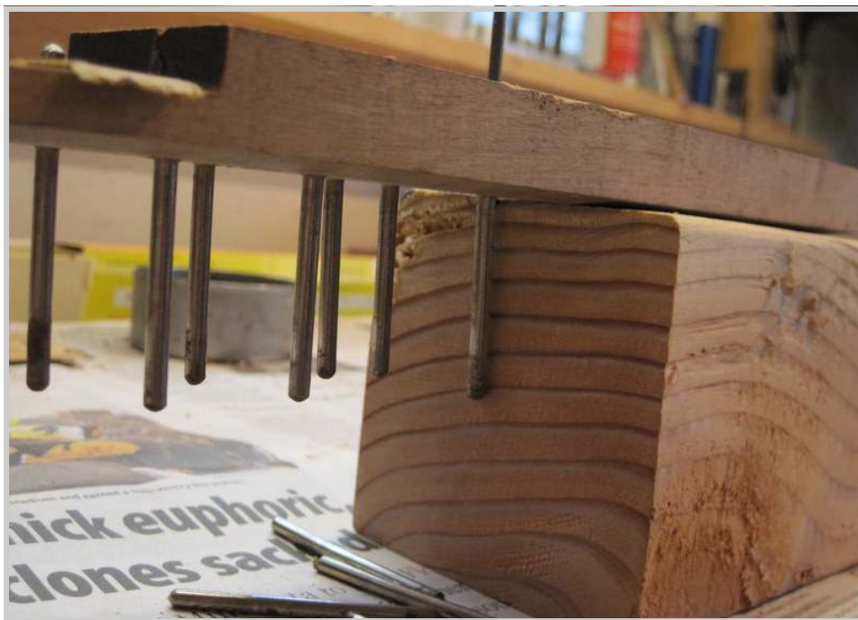
Photo 325: The 4 X 4 block holds the balance rail far enough off of the surface of the bench that the pins are free to drop out below once they are punched through.
