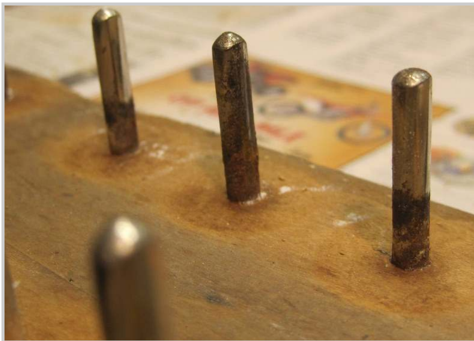
Photo 329: The front rail pins are unfortunately in no better condition than the balance rail pins, and must be replaced as well.
