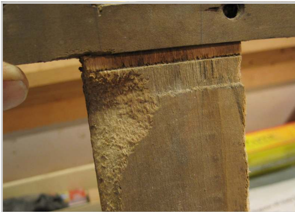
Photo 332: The front to back members of the keyframe, as well as the back rail, have severe damage courtesy of the factory mice. These parts, being of a softer wood than the front and balance rails, suffered from much more abuse. Replacement of these parts of the keyframe, at this stage of the project, seems desirable. If there's one thing I hate, is to finish a job and wish I had done this or done that. "Do it right the first time," was my dad's motto. I've tried to make it mine as well.
