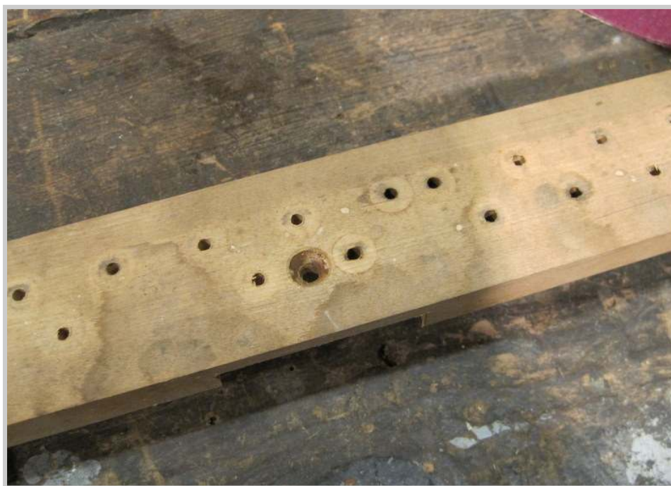
Photo 326: With all the pins removed, the balance rail itself needs attention to remove stains and odors.
