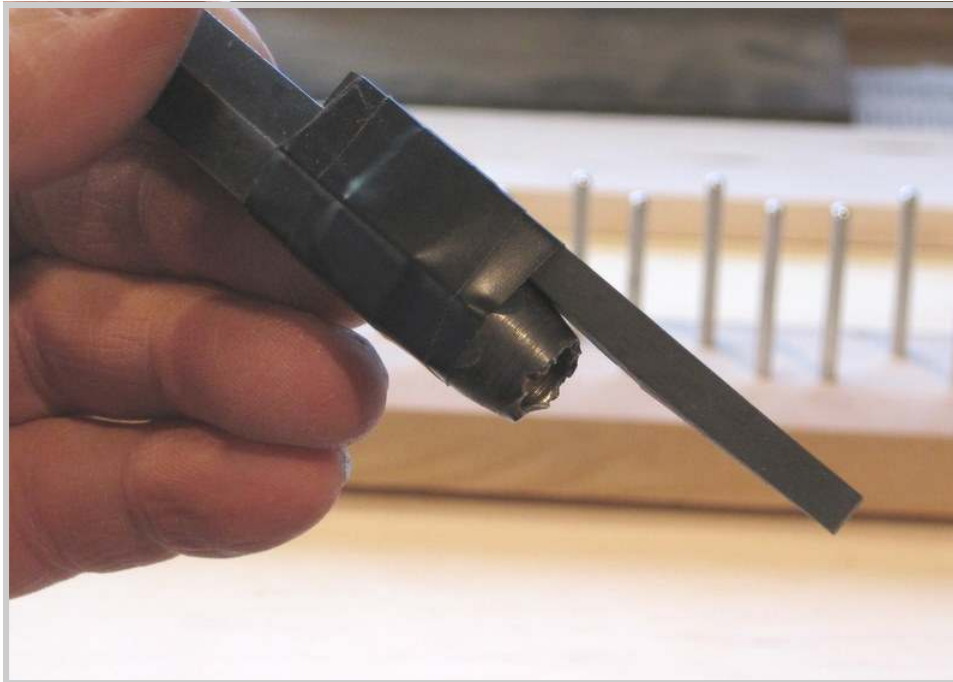
Photo 347: A depth gauge, much like the one used for pounding tuning pins, is made from a piece of rubber wedge attached to the pin punch with electrical tape.
