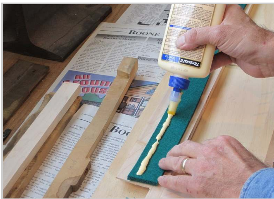
Photo 352: Each piece of felt is flipped upside down and a bead of glue is applied to the back half of each strip.
