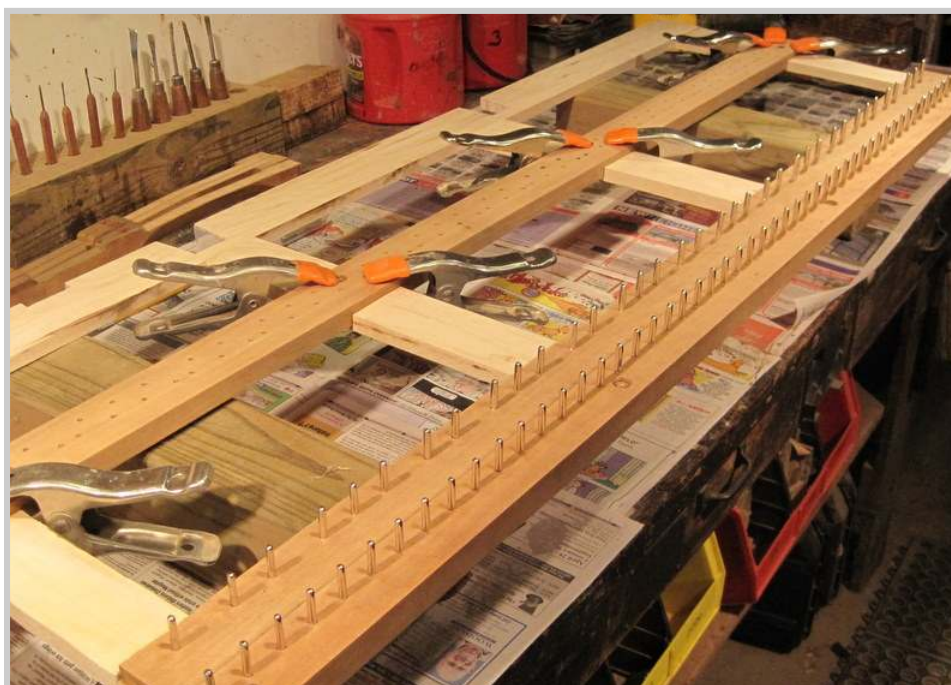
Photo 343: Using the 'press' feature of the drill press, the correct size of front rail pins are pushed into place using the depth setting on the tool. A pin punch is the tool in the chuck of the drill press. The concave tip fits over the end of the pin without marring it in the process.
