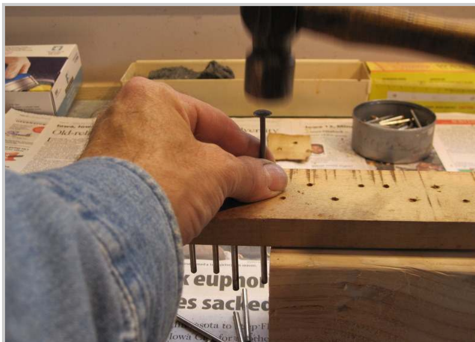
Photo 324: With the balance rail removed from the key frame, the corroded pins are punched out using a roofing nail with the point clipped off.
