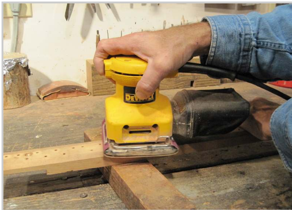
Photo 327: The sanding out process involves a once over with 100 grit paper, followed with 150 and 220. Being a harder wood (maple) than the keybed itself, the staining had not soaked far into the fibers of the wood, and was much easier to remove.
