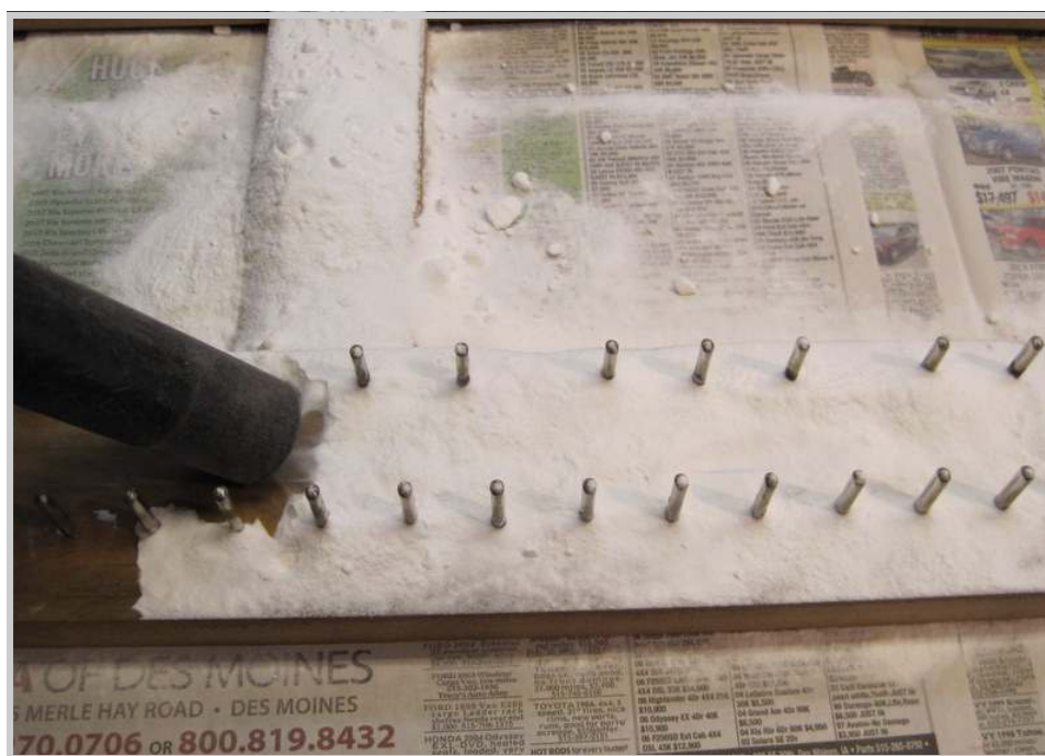
Photo 322: The six pounds of baking soda that have covered the keyframe for more than a month are vacuumed off, taking the mouse odor with it. All I can say is thank goodness for baking soda. It works wonders in this type of situation.
