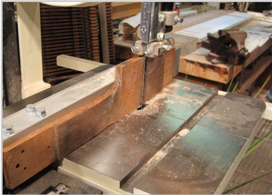
Photo 334: The band saw is set for the thickness of the old stock.
