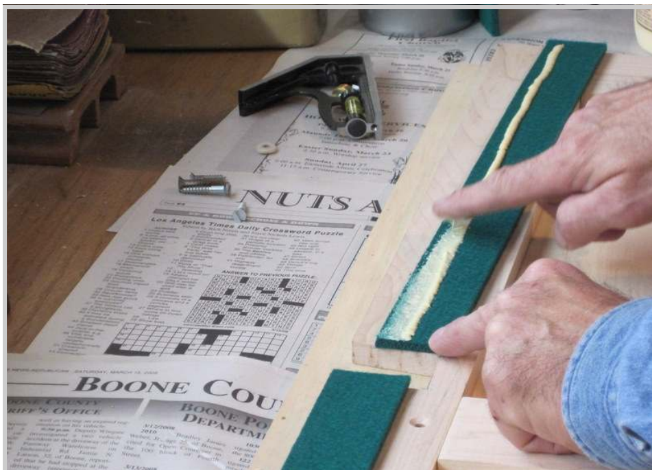
Photo 353: The glue is spread onto the back half of each strip. When the felt is flipped back over, the glue will be on the front half of each strip only. The back half (where the bottom of the keys make the heaviest contact) is left loose in order to reduce the amount of noise transmitted to the body of the piano from the keys falling onto the felt.
