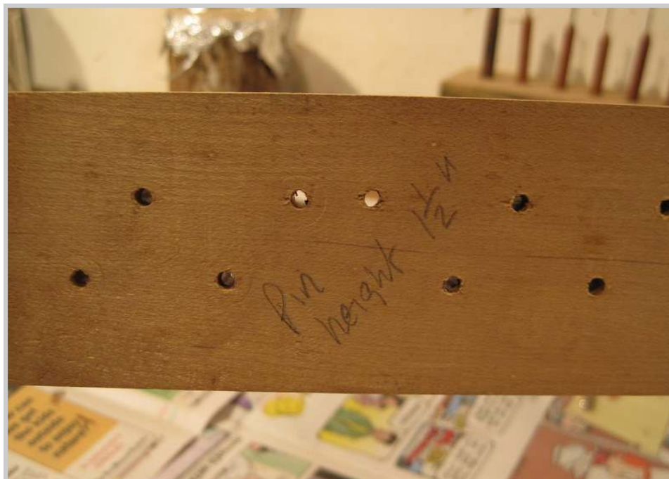
Photo 345: Important measurements, such as this one concerning the height of the balance rail pins, are best recorded in a spot such as this on the bottom of the balance rail itself, where it won't be lost
