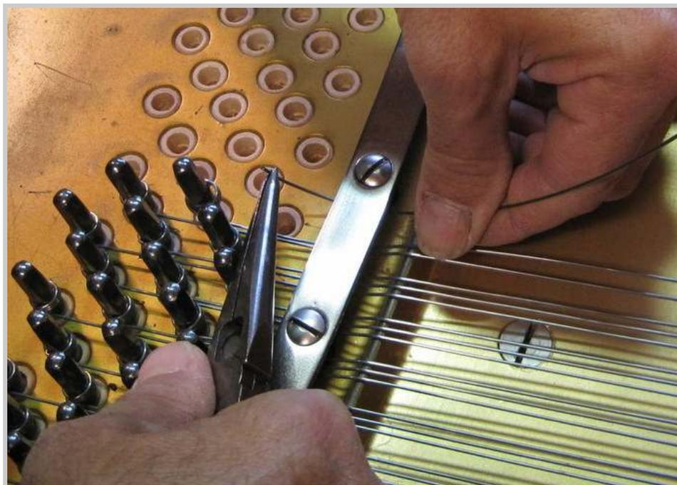
*Photo 273: The second end of the wire is bent in the same manner as the first, and slipped underneath the pressure bar. Once the wire is under the bar, the slack is pulled out of it, and the wire is checked to make sure that it is threaded correctly across the bridge both coming and going.*
