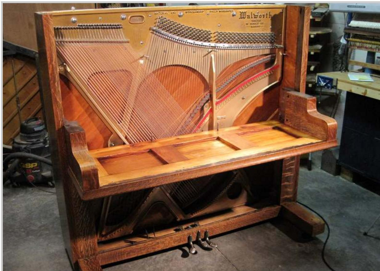
Next photo set: Bass strings are installed, new casters are put on, old rusted pedals are replaced with vintage nickel pedals, the keybed is installed, and the old girl is put back on her feet again! The light at the end of the tunnel is beginning to shine brightly!
