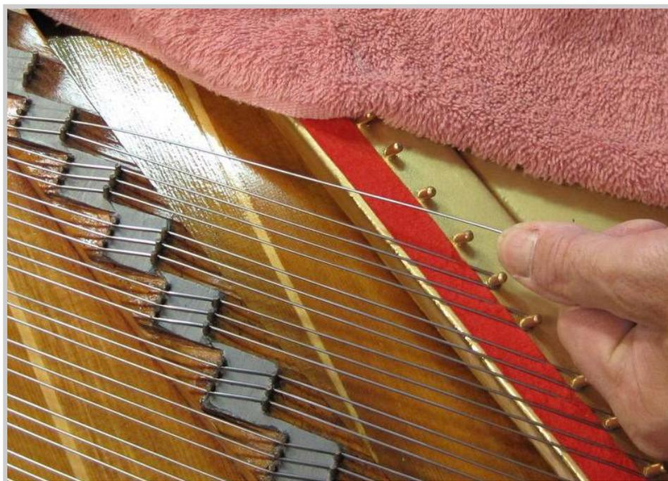
*Photo 268: While pulling back hard on the string to remove any slack, the string is lined up with the intended hitch pin. The felt strip that the string passes over cushions the string from the cast iron plate.*
