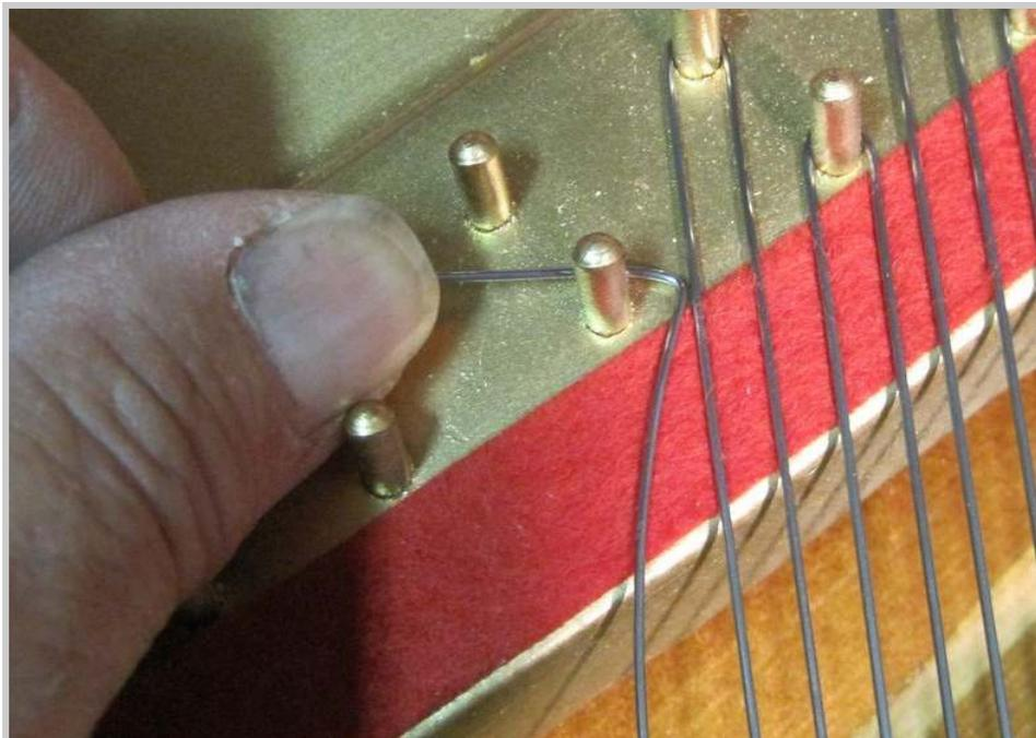
*Photo 271: The bend that has been made in the wire is slipped around the hitch pin.*
