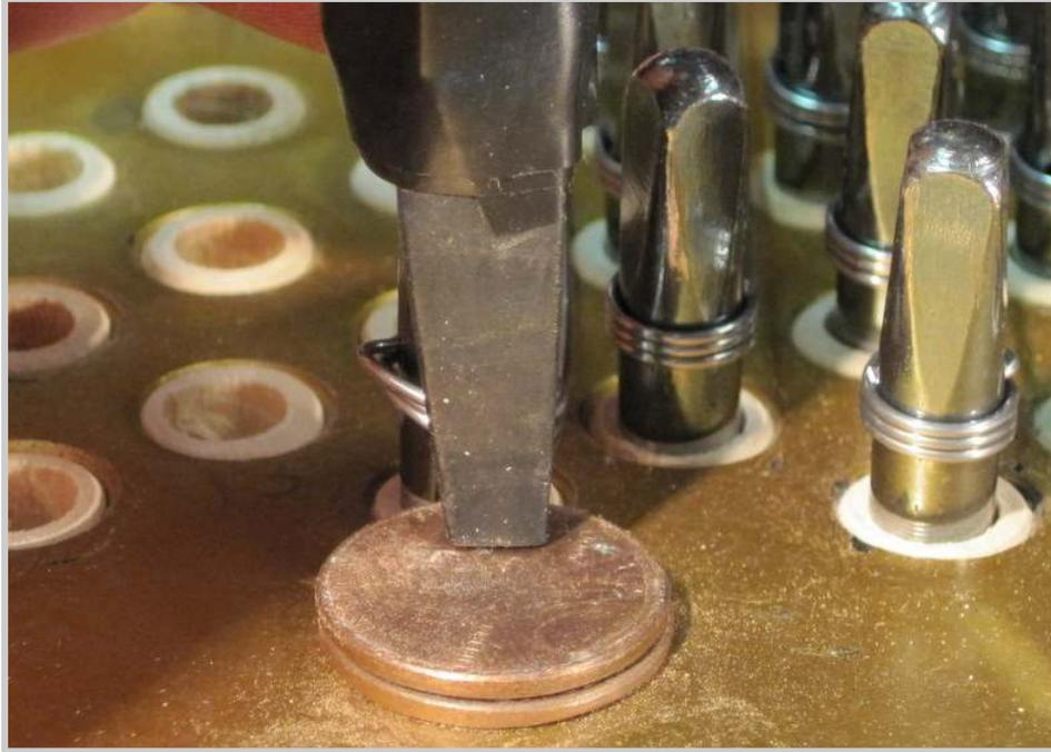
*Photo 265: At this point, the downward progress of the pin is stopped slightly short of what it will be when the pin is completely pounded in. The depth gauge at the initial pounding in should be about the thickness of two pennies (inserted here for the purpose of illustration) from touching the plate.*
