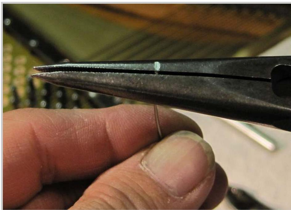
*Photo 258: Before being installed, each wire is first bent in a pair of needle nose pliers which has been marked to produce a bend, or 'becket' of an exact length.*
