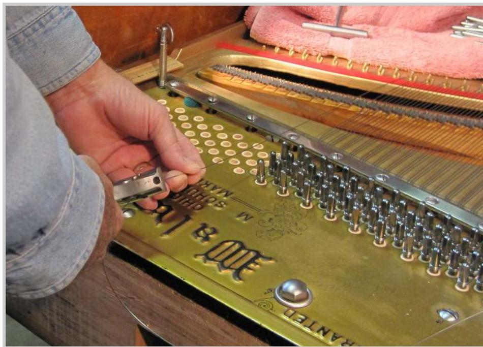
*Photo 272: The wire is now pulled back over the pressure bar and tuning pin field and cut to a workable length. The exact length of the wire is not determined yet, so it is important that the wire be cut longer than will be needed to allow room for error.*
