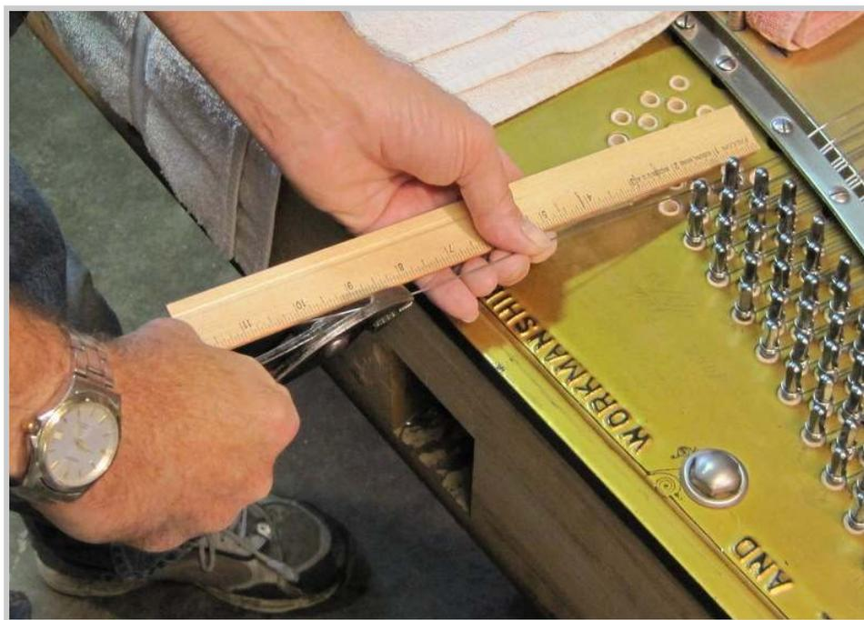
*Photo 274: Using ordinary pliers to firmly grip the end of the wire, it is pulled taut, while a ruler is used to measure the point at which it will be cut.*
