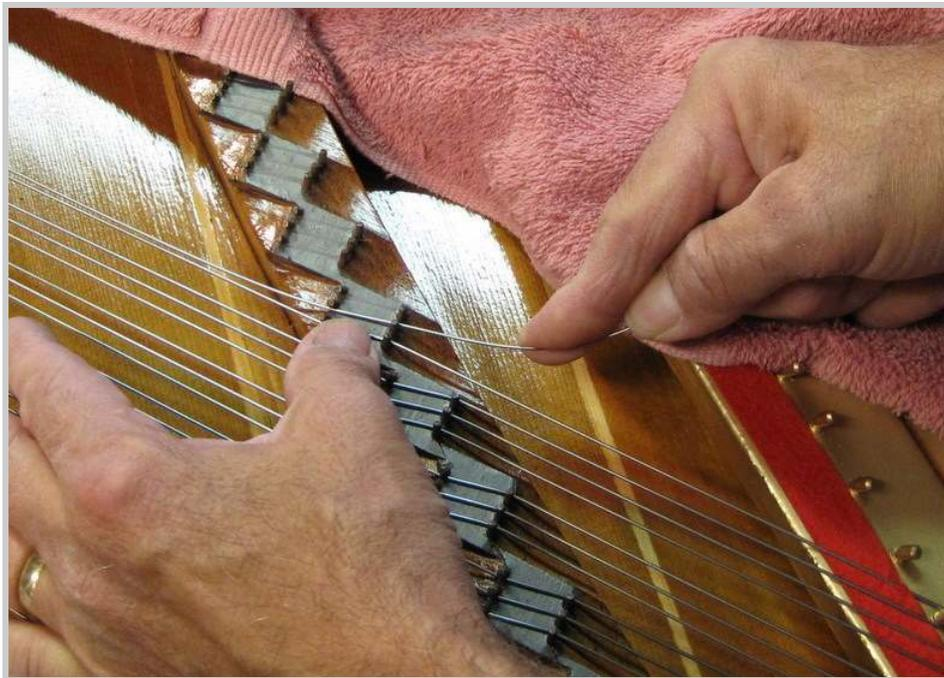
*Photo 267: The string is threaded past the two bridge pins that mark the lower end of the speaking portion of the string. The strings have a slight angle over the bridge, so that when pulled tight the downward bearing, or pressure, will result in the vibrations to be transmitted into the soundboard.*
