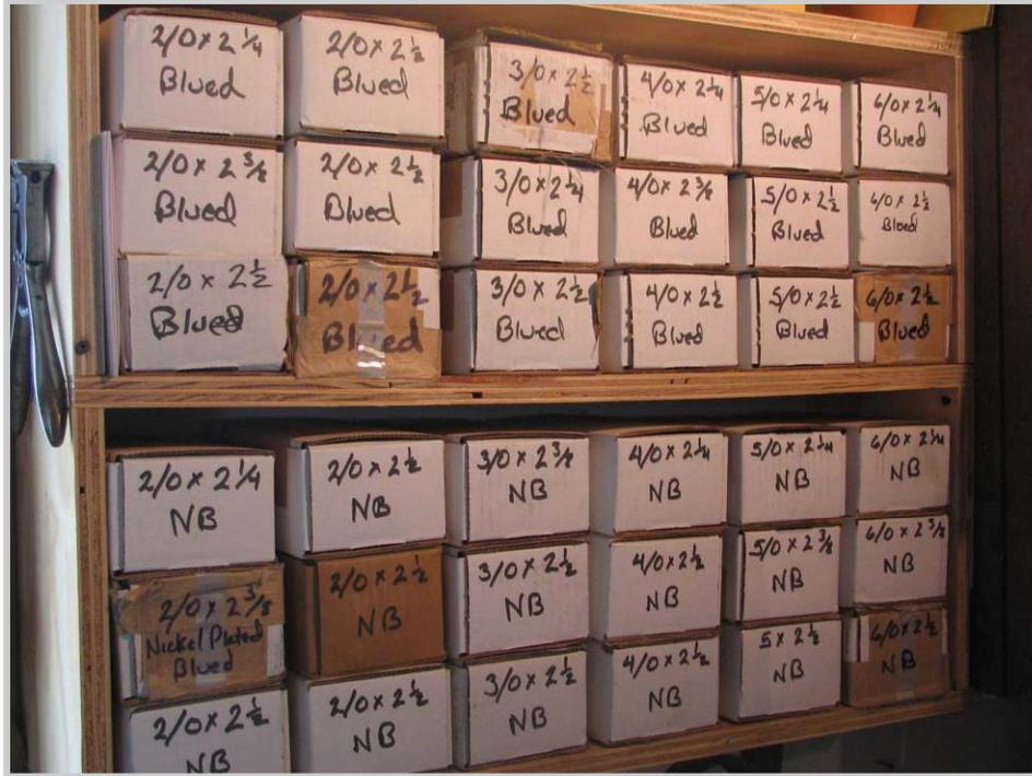
Photo 253: A set of tuning pins are taken from inventory on hand. Depending on the circumstances, different sizes of pins are used in the pinning operation. For a new set of pinblock panels, size 2/0 X 2 3/8 are the necessary size. With a vintage piano, blued pins are what I prefer to install. To me, nickel plated give the piano too much of a modern look.
