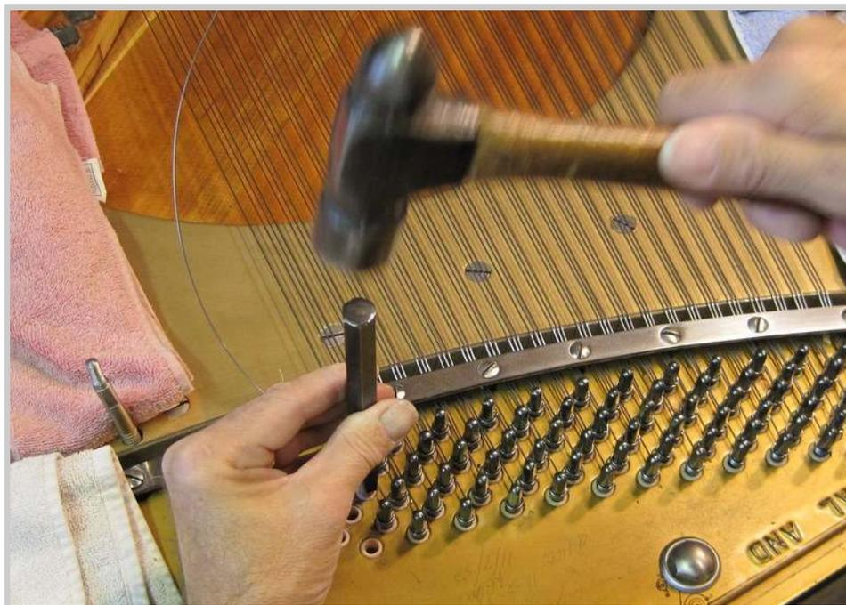
*Photo 264: Using a tuning pin punch with a homemade "depth gauge," the first of the two pins to hold the wire is pounded most of the way in. This pin will serve as a secure post to allow the exact measurement of the wire needed to produce coils with exactly three turns.*
