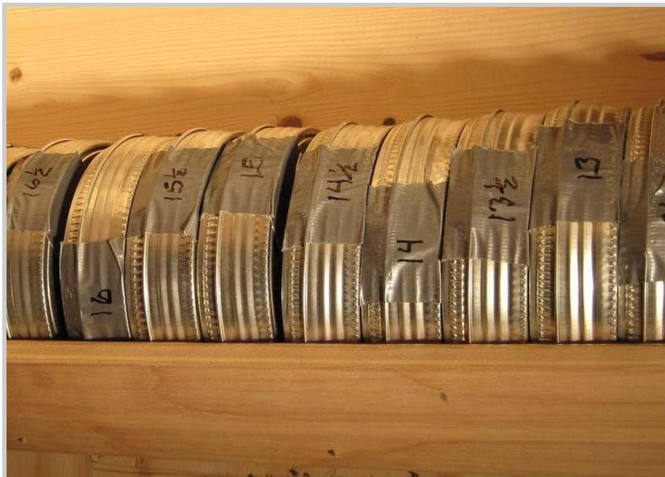
Photo 254: String in one pound canisters is used to restring the piano. I start with the heaviest gauge wire, which in this case is size 20, or .45 thousands, and work my way towards the treble end, where the smallest gauges are used.
