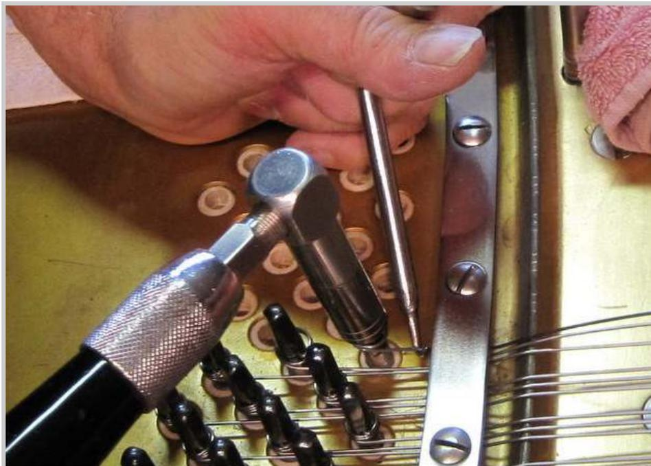
*Photo 279: As a string hook is used to pull the coil tight, the string is given a bit of tension.*
