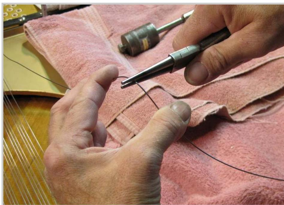
*Photo 270: Without releasing the grip of the round nose pliers, the tension on the wire is released, and the wire is bent into a u-turn at the designated point.*
