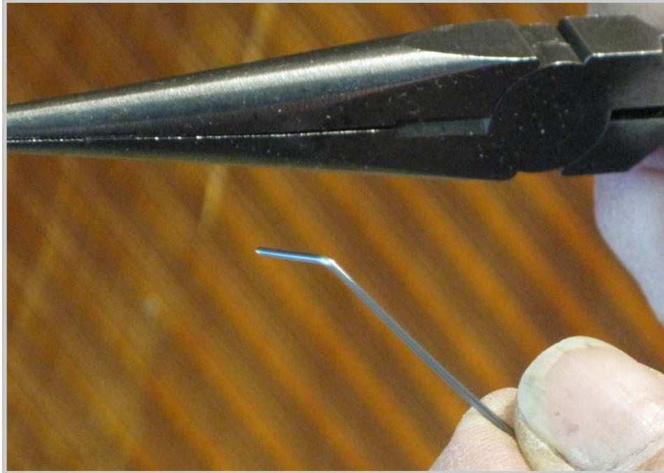
*Photo 259: The becket is first bent to a somewhat shallow angle.*
