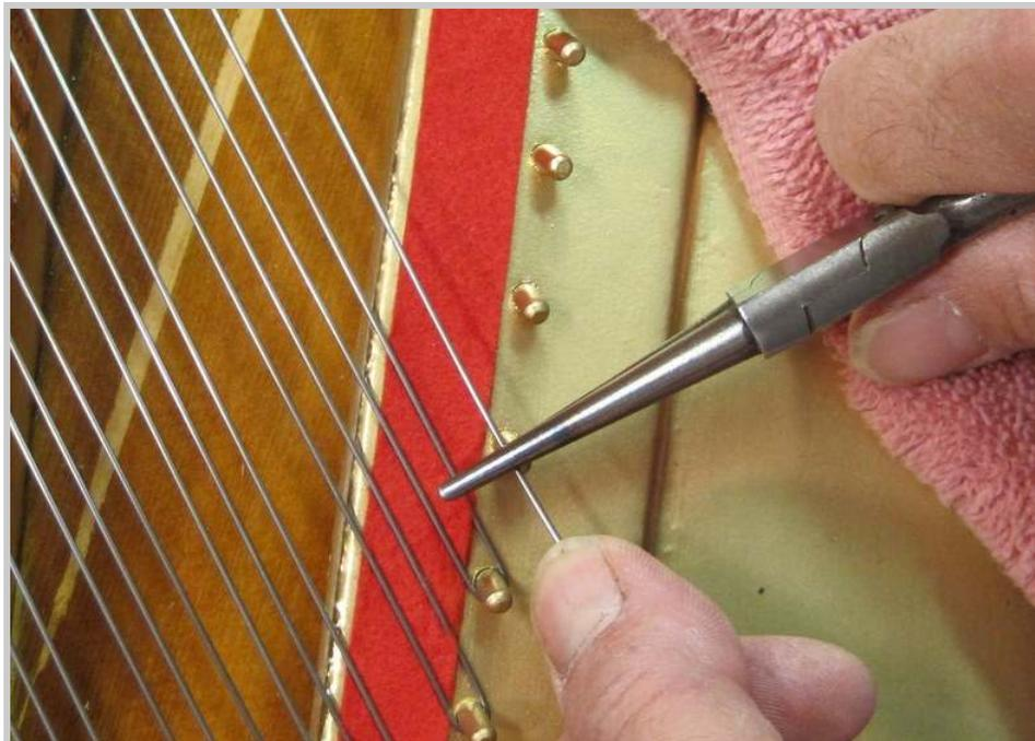
*Photo 269: The string is grasped firmly with a pair of round nose pliers at the exact point at which it will make the turn around the hitch pin. It is vital to be looking straight down when marking the location for the bend.*
