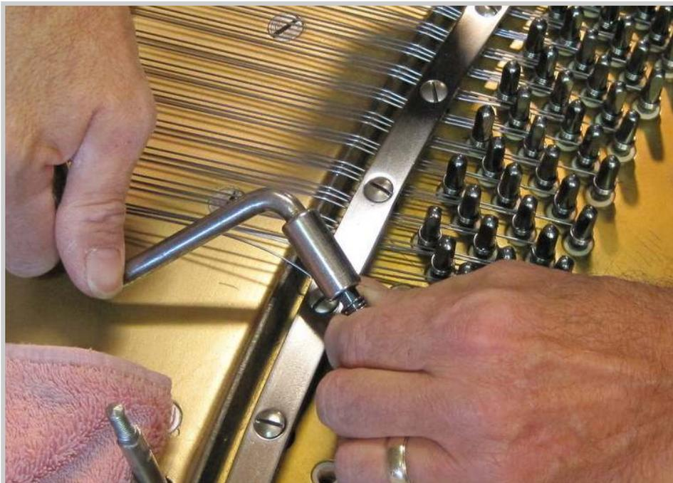
*Photo 277: The tuning pin crank is used a second time. This time, because of the close quarters of the pressure bar, it is a bit more of a challenge to get the required number of turns on the coil.*
