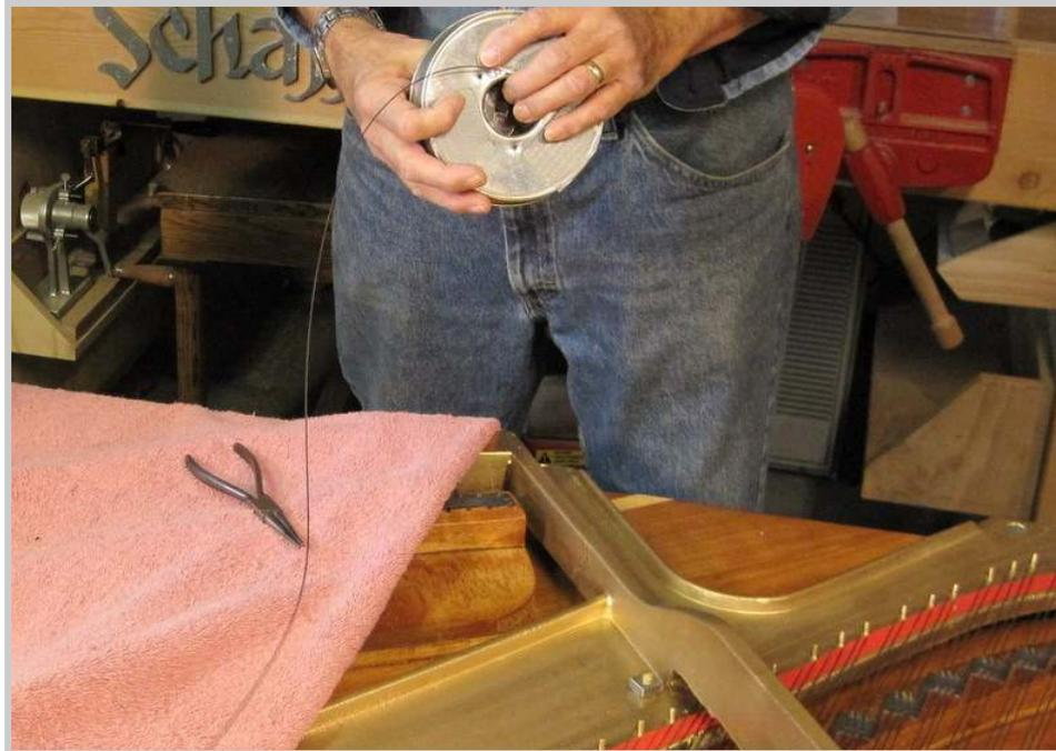
*Photo 266: Wire is unreeled to reach past the hitch pin on the bottom end of the plate.*
