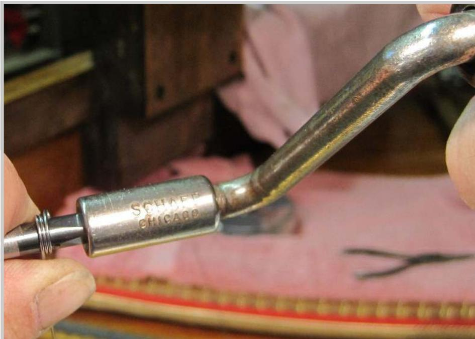
*Photo 263: Using a tuning pin crank, a coil is put on the end of the piano wire. The coil is to have three complete turns when the wire is installed and brought up to tension.*
