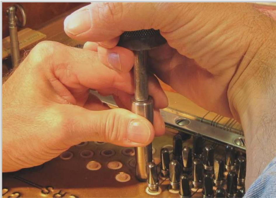
*Photo 281: An impact coil tightener is used to produce more tightly wound coils. The beauty of this tool is that unlike levers used for the same purpose, the coil tightener does not touch or mar the cast iron plate.*
