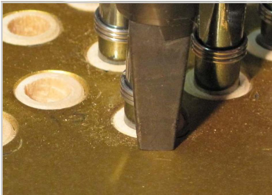
*Photo 283: The pin is now pounded all the way in. The depth gauge should just touch the plate.*
