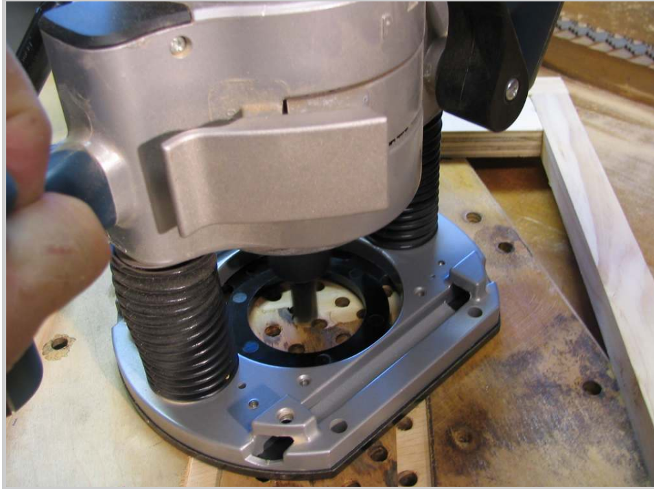
Photo 155: With the outside perimeter of the cut made, the router bit is worked back and forth to clear out the wood in the middle. It is important that both sides of the router remain supported by the sides of the original pinblock, to avoid having the router bit dip inward and cut a divot in the bottom of the cutout.
