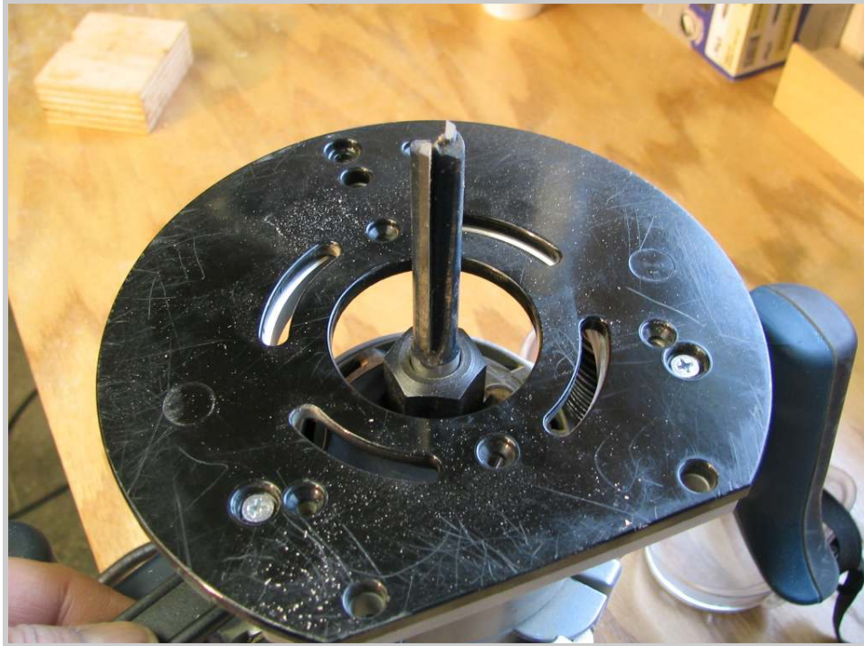
Photo 157: A long straight bit is substituted at this point. This bit is too long to have begun the cutting process with, but is needed to complete the cutout to the required 1 3/8" depth.
