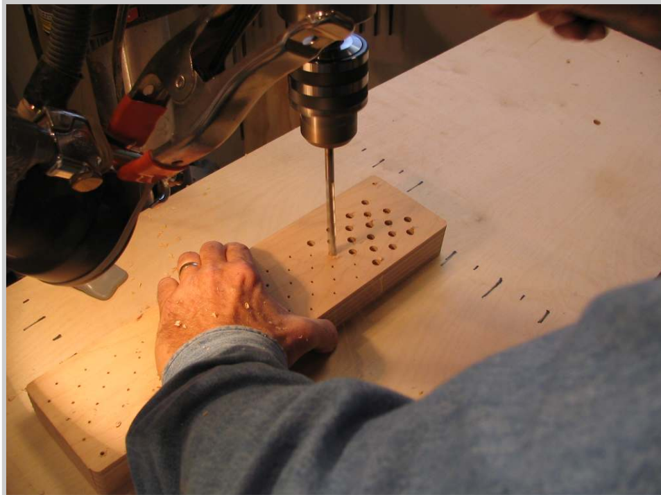
Photo 174: The pin holes are drilled on the drill press. A high speed drill bit is used which is .01" smaller than the size 2 pins to be driven in. A air stream is focused on the drill bit, which helps to keep it cool. With this setup, one hole can be drilled every several seconds continuously. The bit is slightly warm when all the holes are finished.
