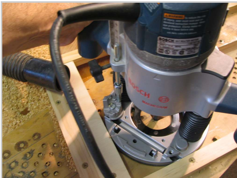
Photo 158: The cutting continues, using the guide frame to cut the outer perimeter first. Each cut is made in the same way, with the perimeter cut made first, then the inner area cleaned out. Again, the cut proceeds at 1/8" increments for a perfectly smooth finish to the cut.
