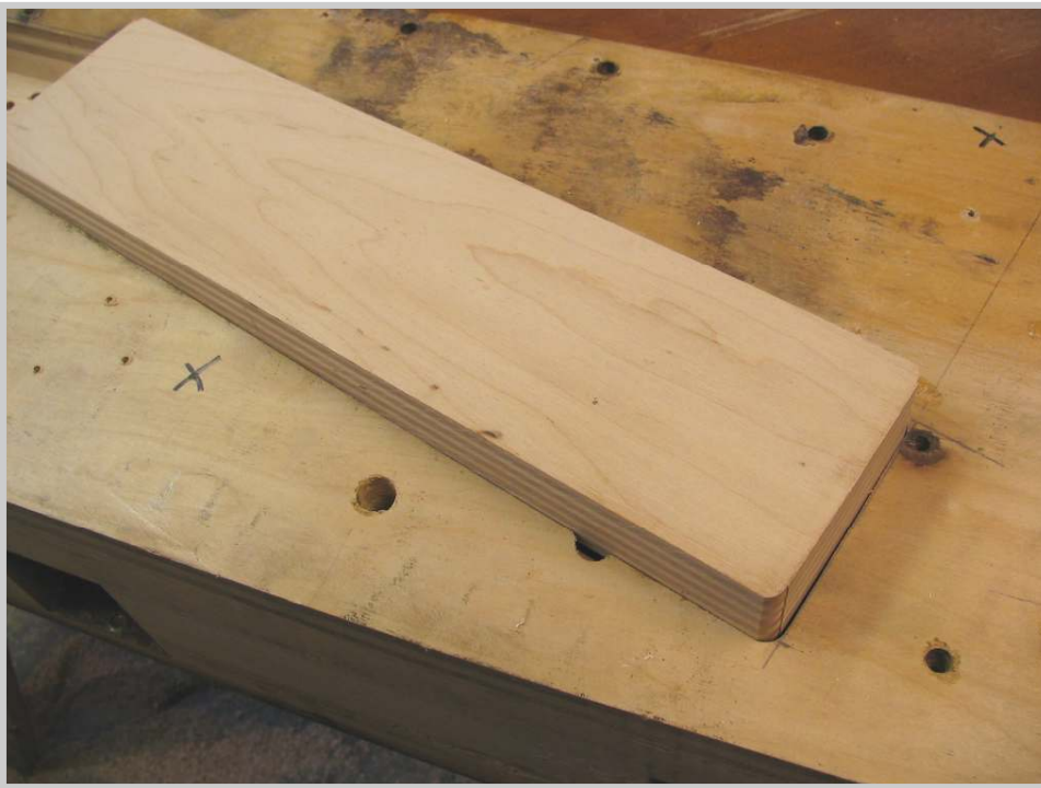
Photo 166: Final fitting. The corners of the panel have been rounded on the router table to match the inner curvature of the corners of the cutout.
