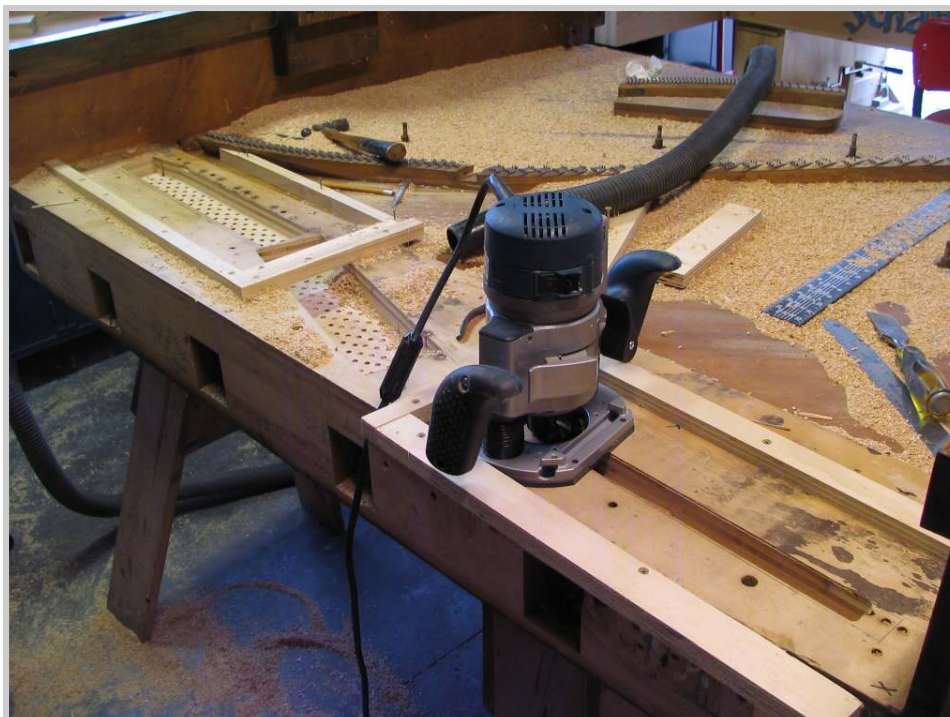
Photo 161: With the middle pin field cutout made, guide frames are made for the pin fields on the bass and treble ends of the pinblock. These cutouts are then made in a similar manner.
