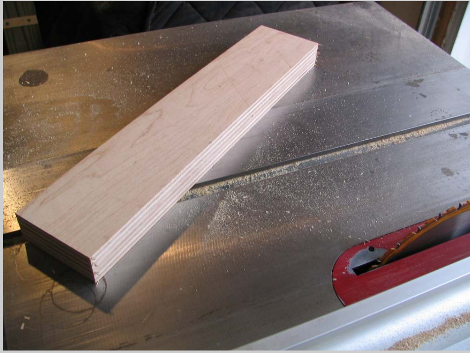
Photo 165: The middle panel is cut to approximate size. I like to cut it just a bit big, then shave it down a hair at a time until it just slides into the cutout hole without binding. I shouldn't be so tight that it has to be pounded in, since it will be put in and pulled back out several times in process of drilling the pin holes.
