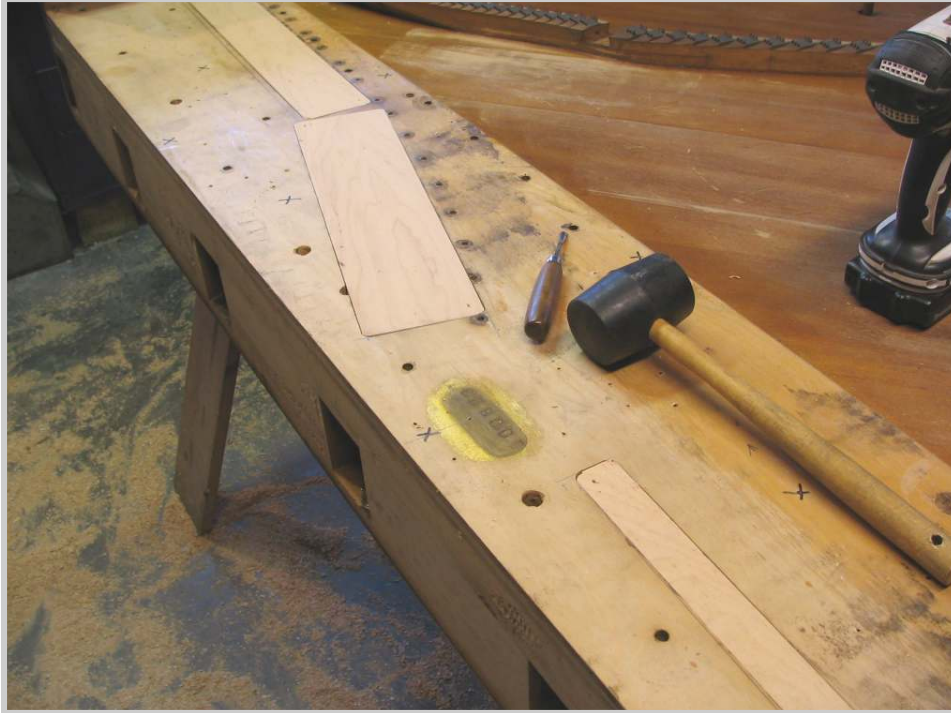
Photo 167: The three panels fitted and in place and ready to mark for pin holes.
