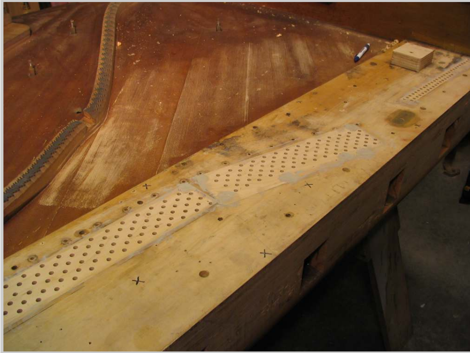
Photo 179: The top of the screw holes are filled with epoxy.
