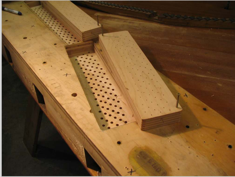
Photo 173: The panels are removed for drilling the pin holes. The slanted line on the sides of the panels references the orientation of the holes to be drilled, which will slant backwards 7 degrees from the vertical. The pins will lean slightly back from the soundboard area of the piano.
