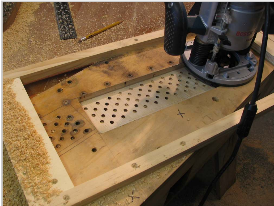
Photo 156: After six cuttings, the depth of the excavation is at the limit of the initial router bit. A change of bits is necessary at this point.
