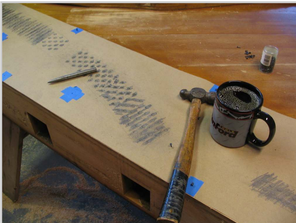
Photo 170: The position of each of the pins in the three pin fields is thus marked.
