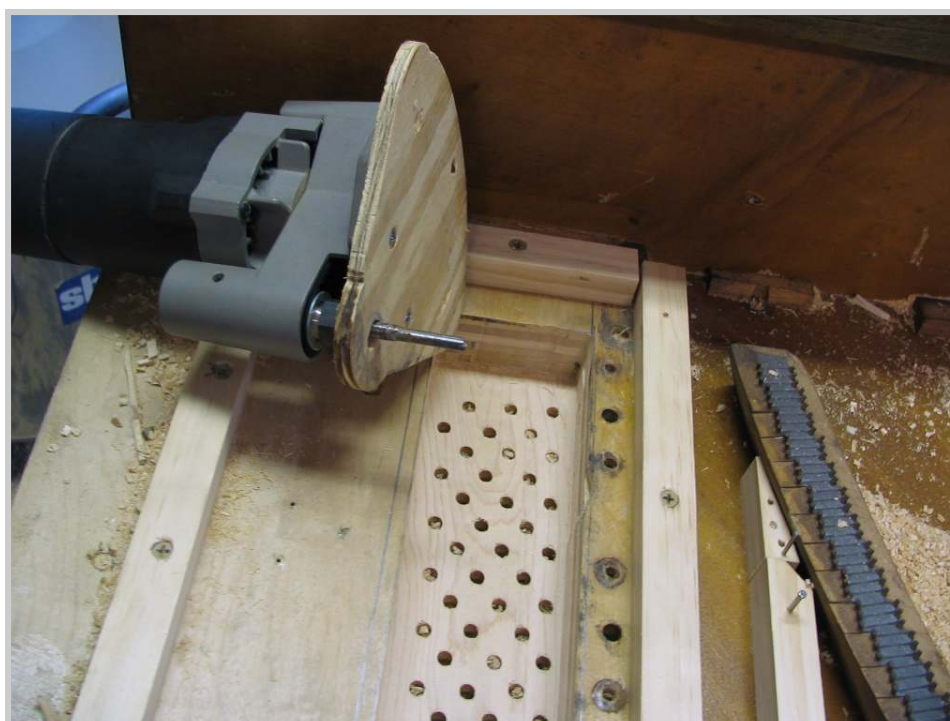
Photo 162: For the very ends of the bass and treble cutouts, an offset router is used to get in closer to the edge than possible with the big plunge router.
