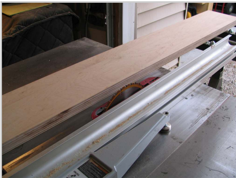
Photo 164: The panels will be cut from 1 3/8" hardrock maple pinblock stock.
