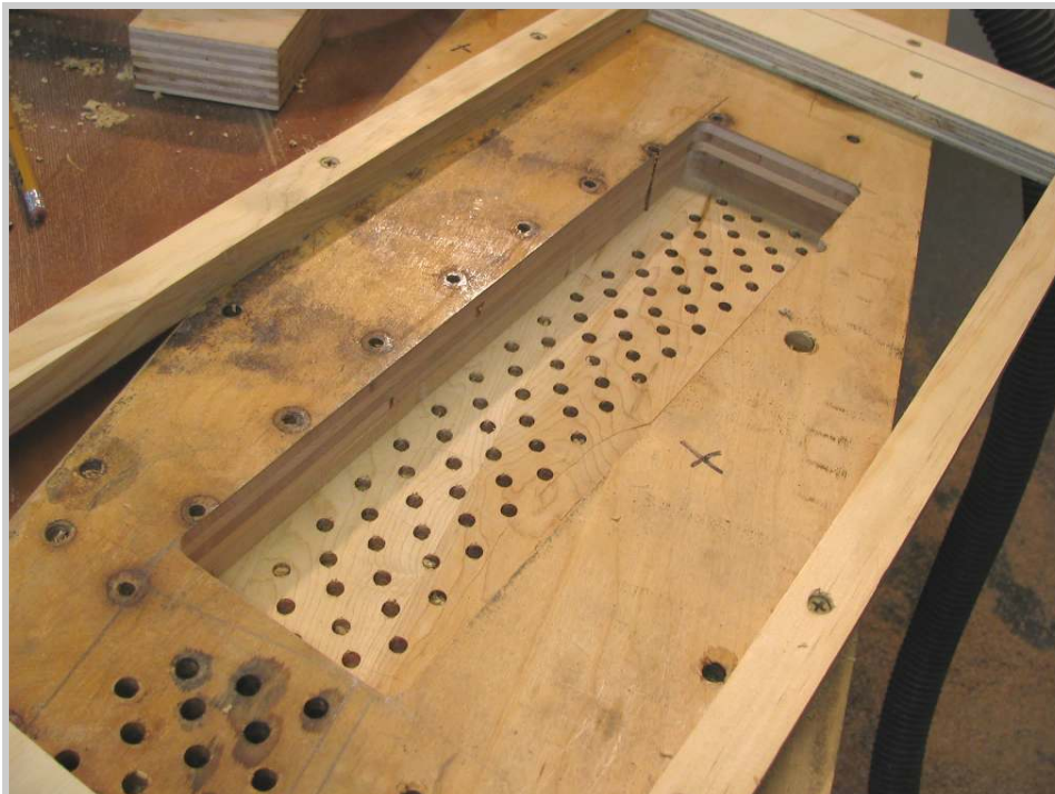
Photo 159: The full depth of the cut is accomplished. The bottoms of the original pin holes remain, in that they were drilled deeper than the thickness of the replacement panels which will be used.
