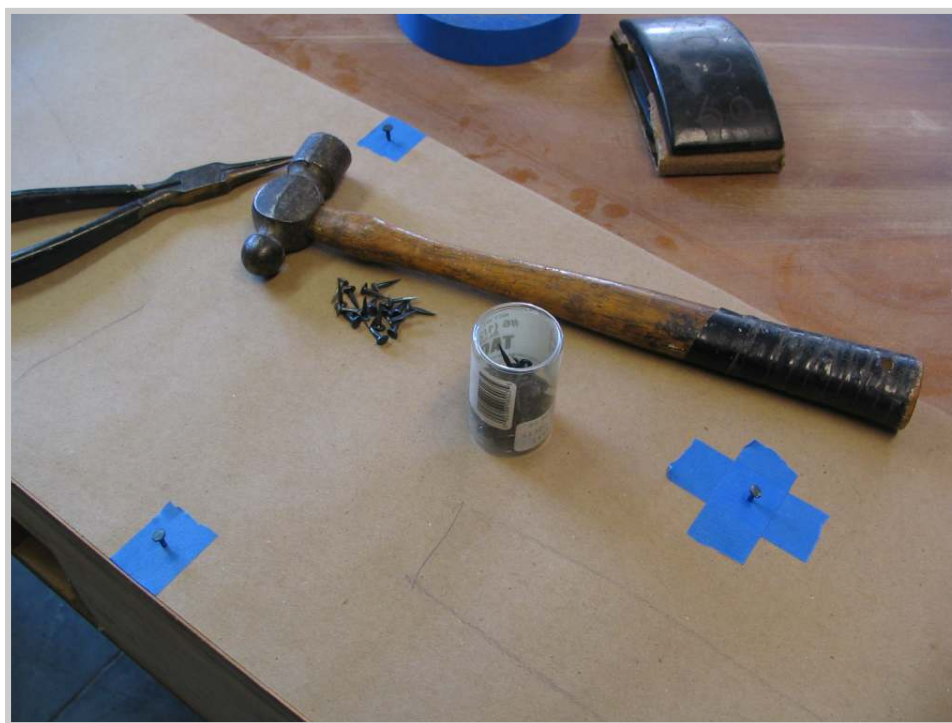
Photo 148: The first step is to spread contractor's paper over the entire pinblock. The approximate location of the pin fields are marked with pencil. The tacks are to locate the exact position of the contractor's paper again at a later step.
