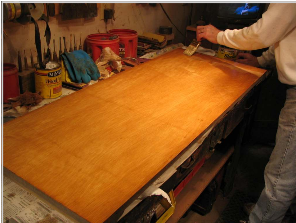
Photo 144: Before applying finish to the fronts of parts, Dave applies 3 coats of shellac for protection to the backs of all the pieces.
