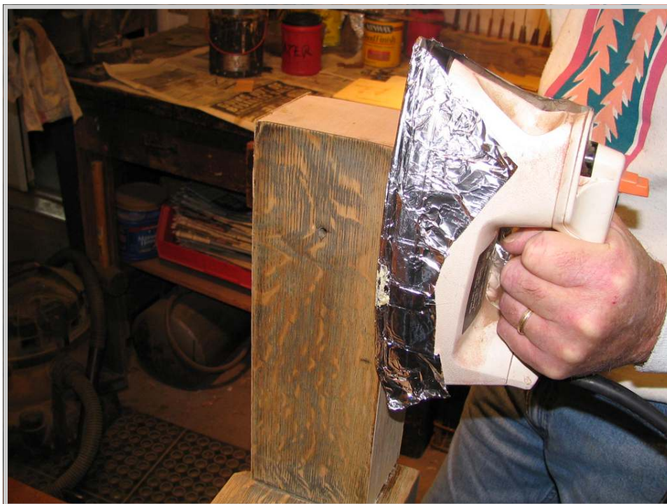
Photo 138: Dave applies the new face veneer to the sides. The hot glue is brushed on the veneer and allowed to cool, then the piece is heated with an iron to remelt.
