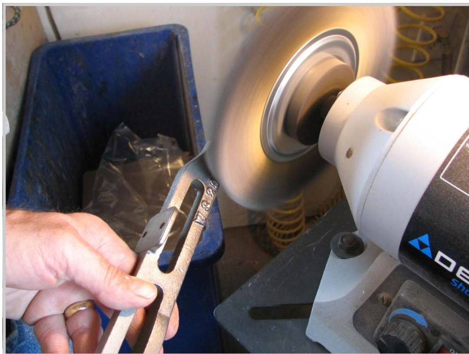
Photo 131: A few minutes on the buffing wheel with a brass wire brush brings a shine back out.
