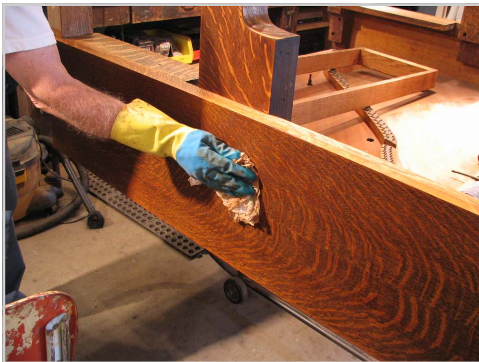
Photo 142: At long last, Dave is able to apply the stain. The desire of the owner is to use a lighter shade. Golden oak was the preferred tone, which will bring out the grain beautifully.
