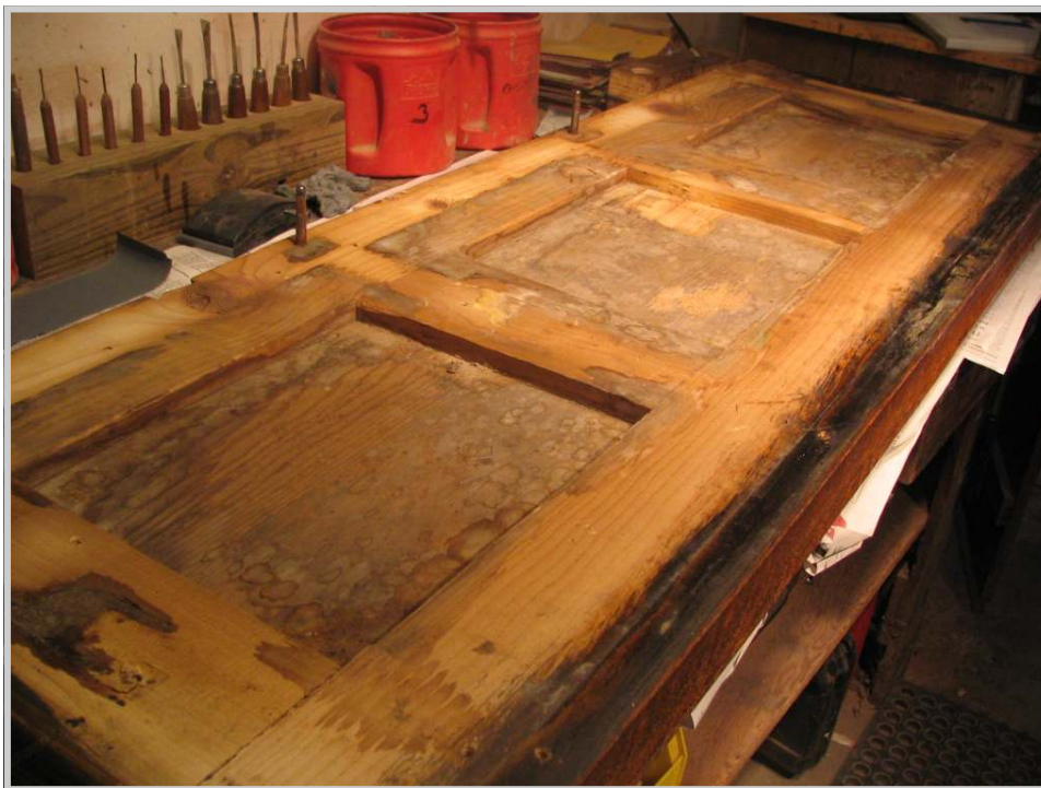
Photo 122: The keybed of the piano, which for decades served as a restroom for mice, could be ignored no longer. With every thing else sanded and ready to finish, I told Dave that I wanted the keybed looking (and smelling) like new. In a word, it reeked.
