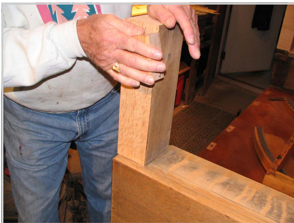
Photo 139: A cold block of pinblock scrap is then used to flatten the veneer out and set the glue.
