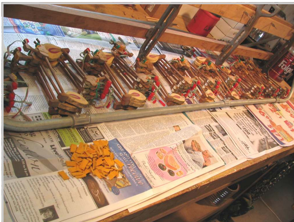
Photo 128: With every bit of leather and felt replaced, I put the hammer butts in order in preparation of reinstallation on the action..
