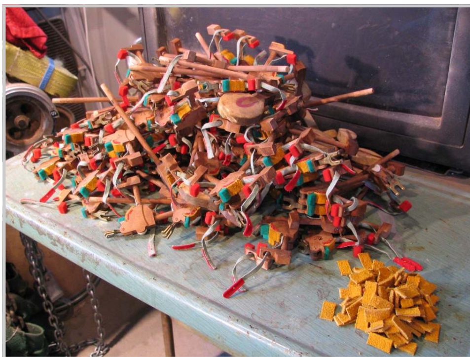
Photo 127: While Dave has been in the finishing stages of preparing to apply varnish, I wrapped up the hammer butt restoration project. Here, the stack of nearly finished butts piles up, needing only new catcher buckskin to finish the job.
