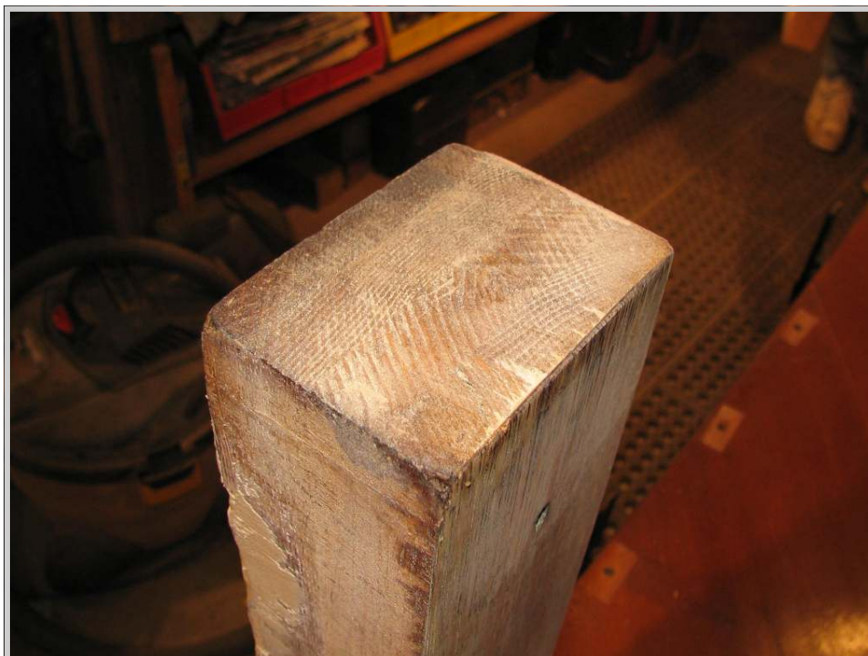
Photo 134: With both the veneer and crossbanding (underlying layer of veneer) removed, the foot of the piano is ready for reveneering.
