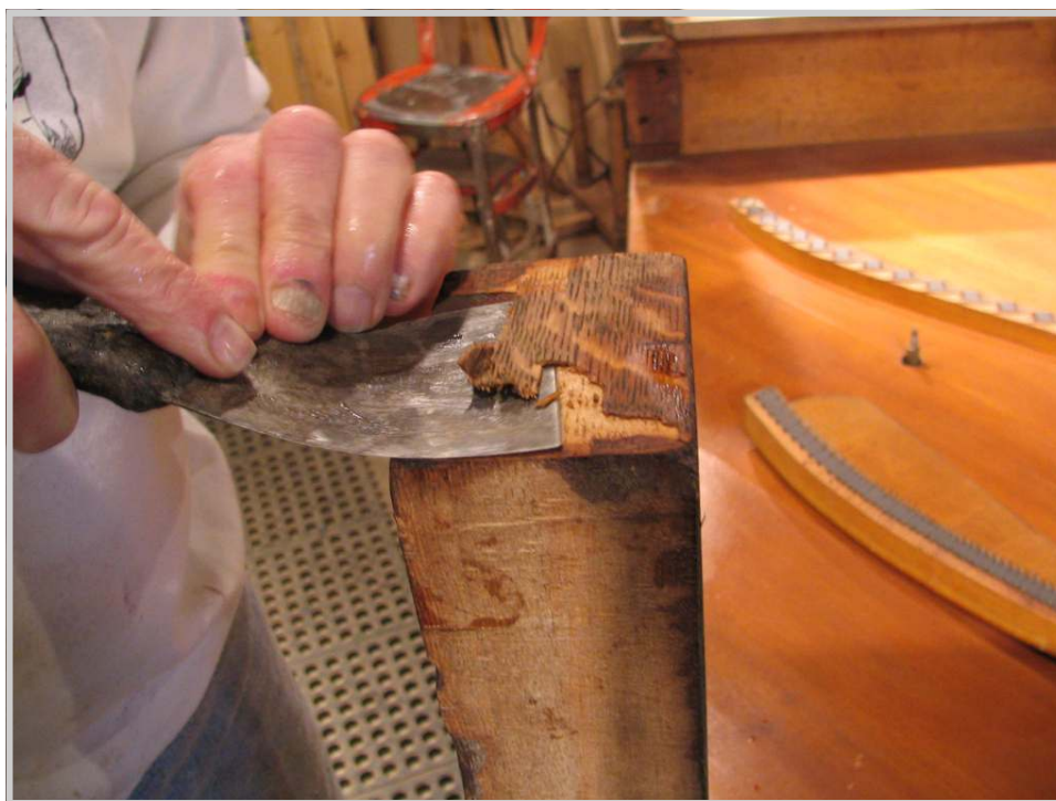
Photo 133: After steaming, the old veneer comes off easily with a putty knife.
