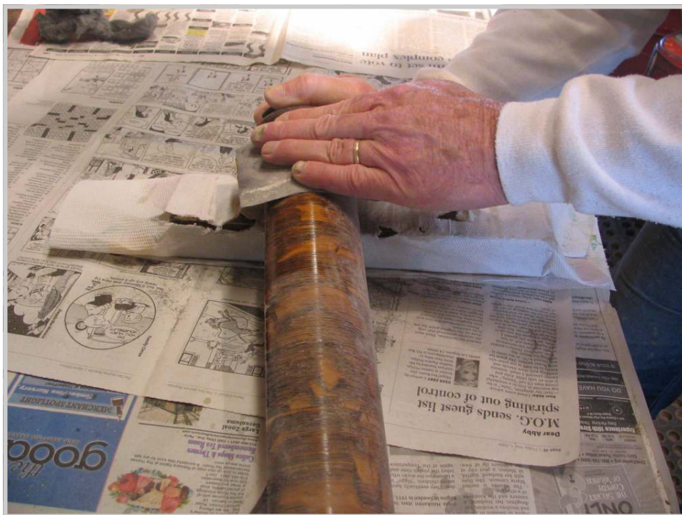
Photo 145: Dave buffs a part in between coats of varnish.
