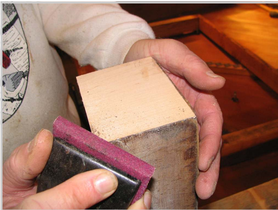
Photo 136: Dave sands the edges of the crossbanding layer flush to the sides.
