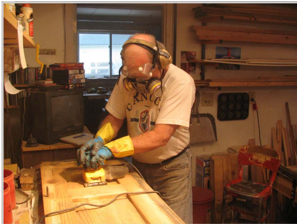
Photo 124: While I retire to another room of the shop (and close the door behind me) to work on another piano, Dave has at the keybed with sheet after sheet of 60 grit sandpaper. The shop is thick with evil smelling dust. I help Dave out by opening doors and windows, and turning on the dust filters—before heading back to the other room.
