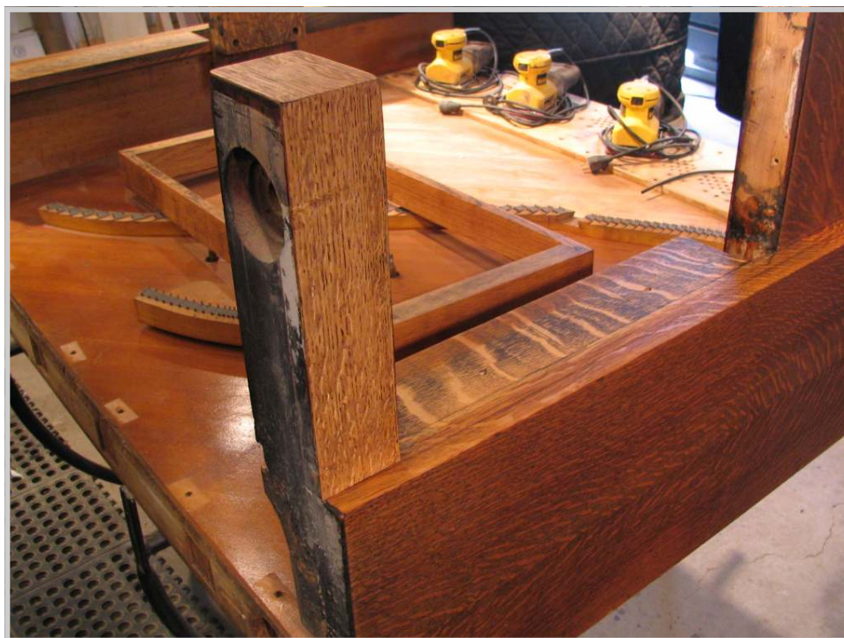
Photo 143: The stained body, sporting newly veneer feet. Minor differences in shade between old and new veneer will be resolved later with an application of colored varnish in between clear coats.
