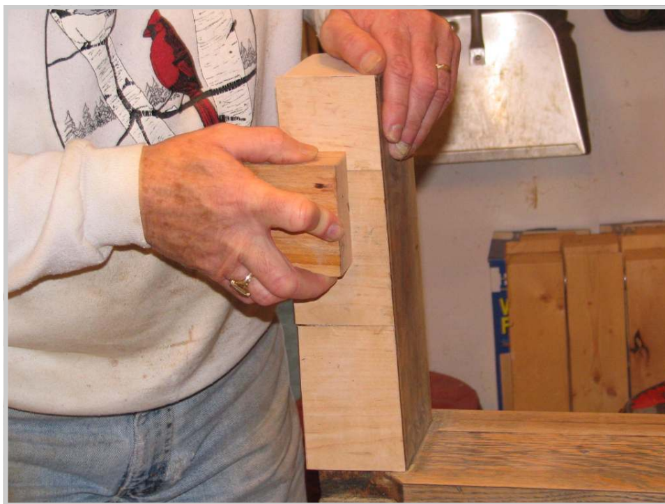
Photo 137: After filling in several gouges in the core wood with an epoxy filler, Dave applies the crossbanding layer to the sides of the foot.
