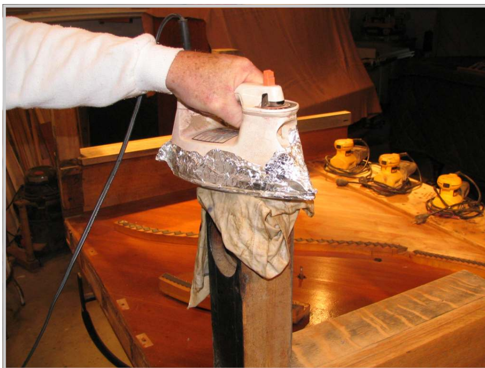
Photo 132: Dave has some final veneer replacement and lacquer stick work to do, then it's on with the stain. Here, he heats up damaged veneer for removal.
