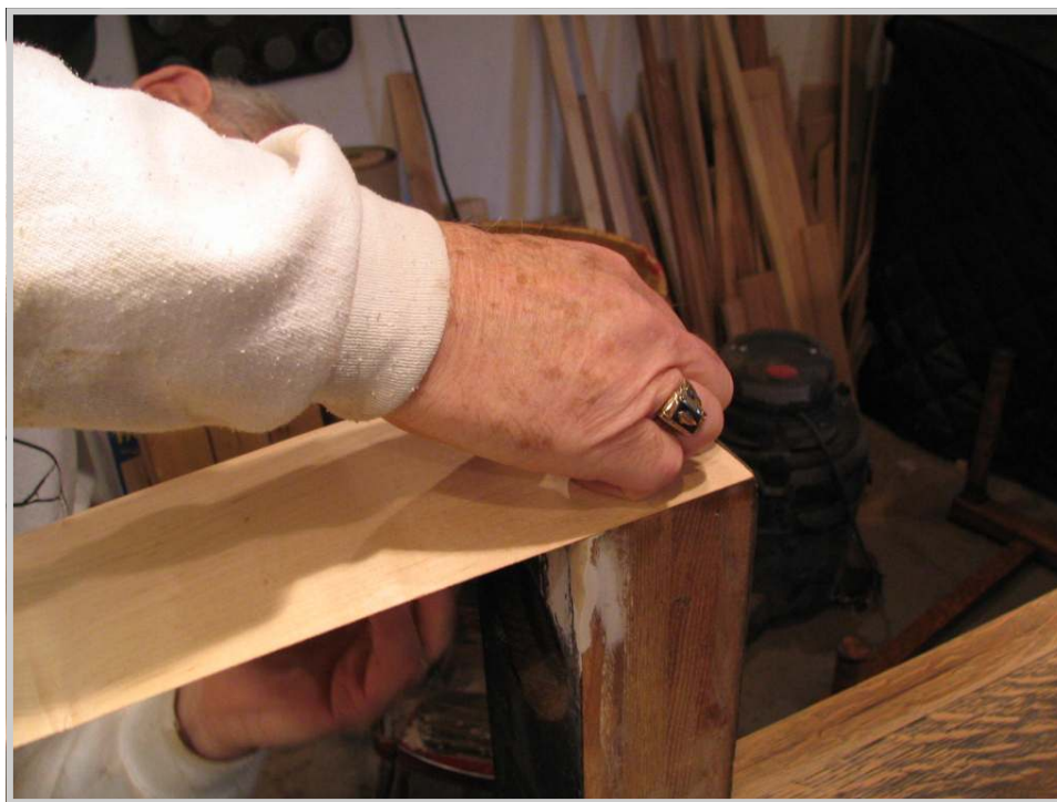
Photo 135: Dave marks the crossbanding veneer for cutting. It will run with its grain perpendicular to the face veneer.
