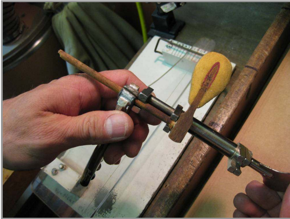
Photo 112: he takes off one of the shanks to determine the bore diameter. Chuck has decided to use new upright shanks so we can use a standard 7/32" drill bit.
