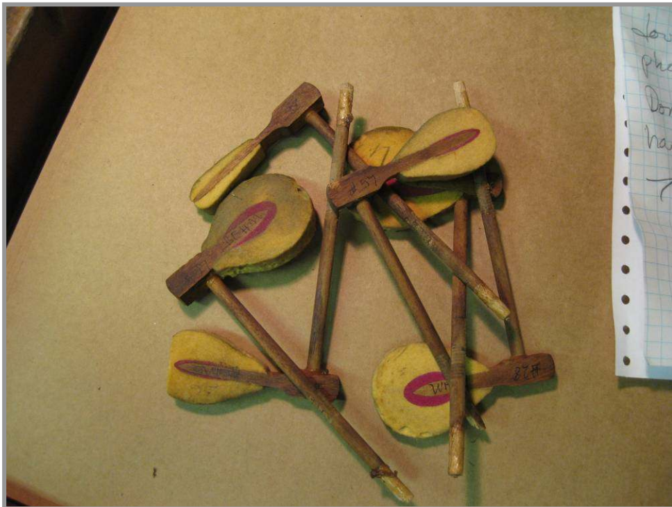
Photo109: Our hammer department receives the first and last hammers in each section. Each sample is numbered as they lie in the scale. We strongly recommend that all shanks are left in so that we can get the most accurate dimensions.
