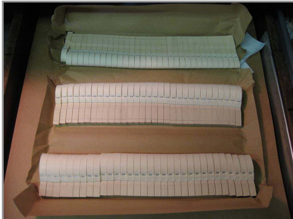
Photo 115: The overall length of #1 and #88 are measured. He opens the best matching hammers based on hammer manufacturer, weight and overall length.
