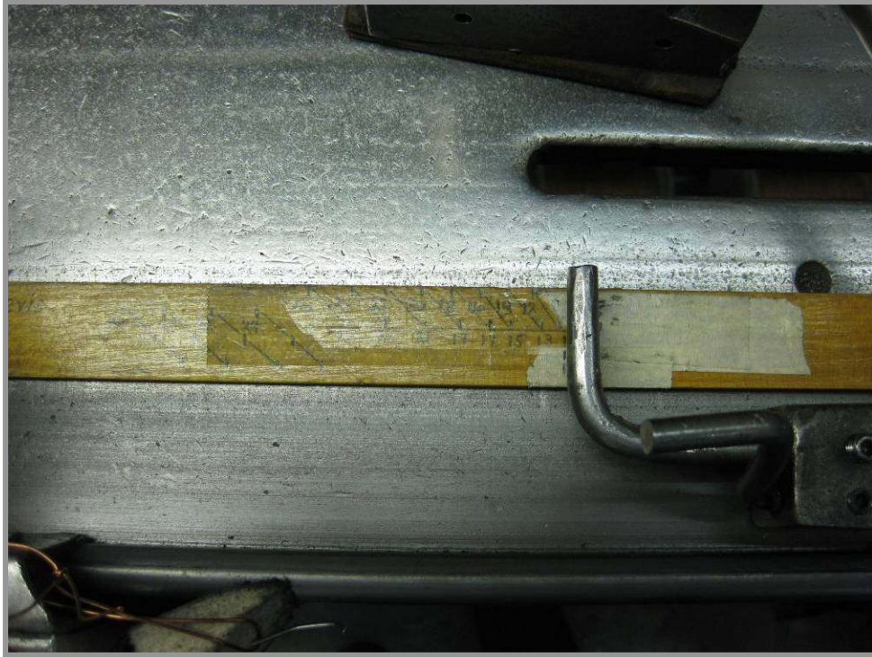
Photo 102: The right measuring device is then set according to the spot where the winding ends
