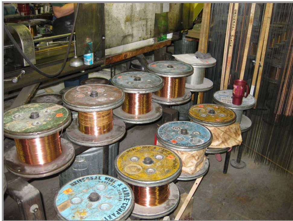
Photo105: Behind the string winders are all of the different gauges of heavy copper. Each scale lists which core diameter and copper size to use.
