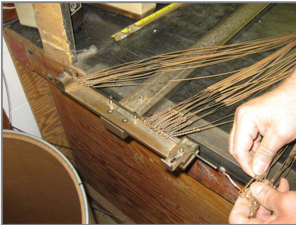
Photo 99: Ed is laying out a set of strings to be duplicated. They are strung on our measuring device to count strings, measure winding dimensions and diameters. He then consults with our records to determine if we have a scale. Once the scale is found, he double-checks the measurements against the stick. Now the set of bass strings is ready to be duplicated.
