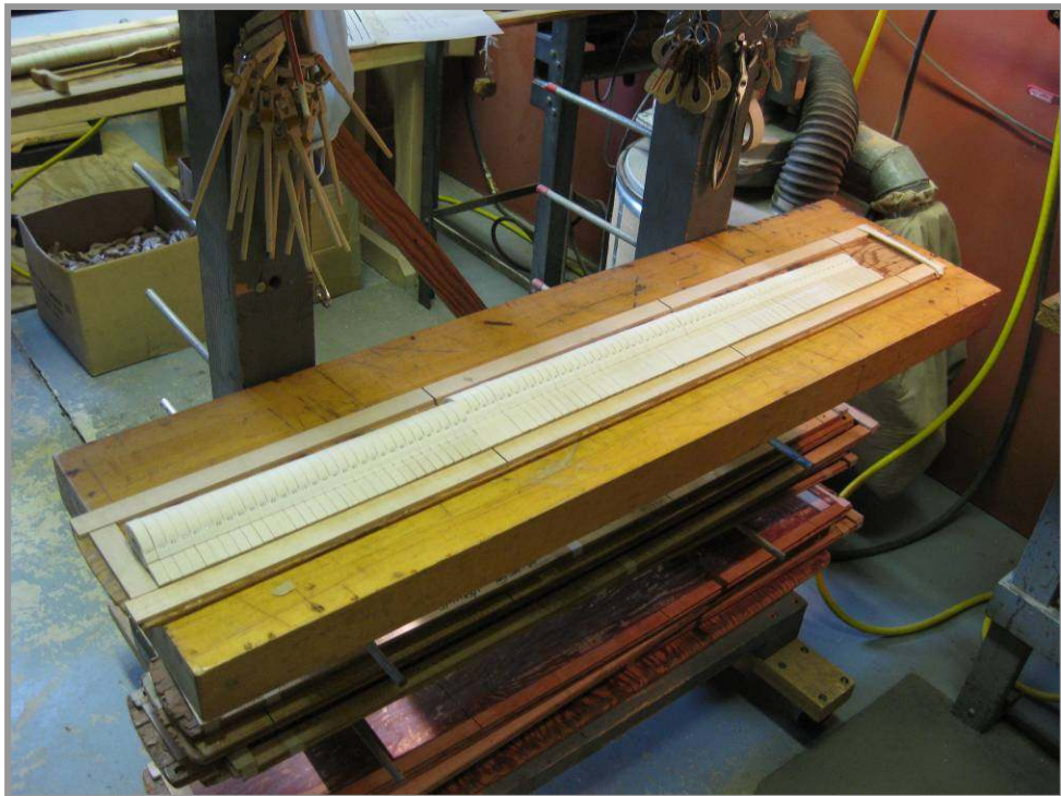
Photo 117: The new set of hammers are laid out and are now ready to be drilled.
