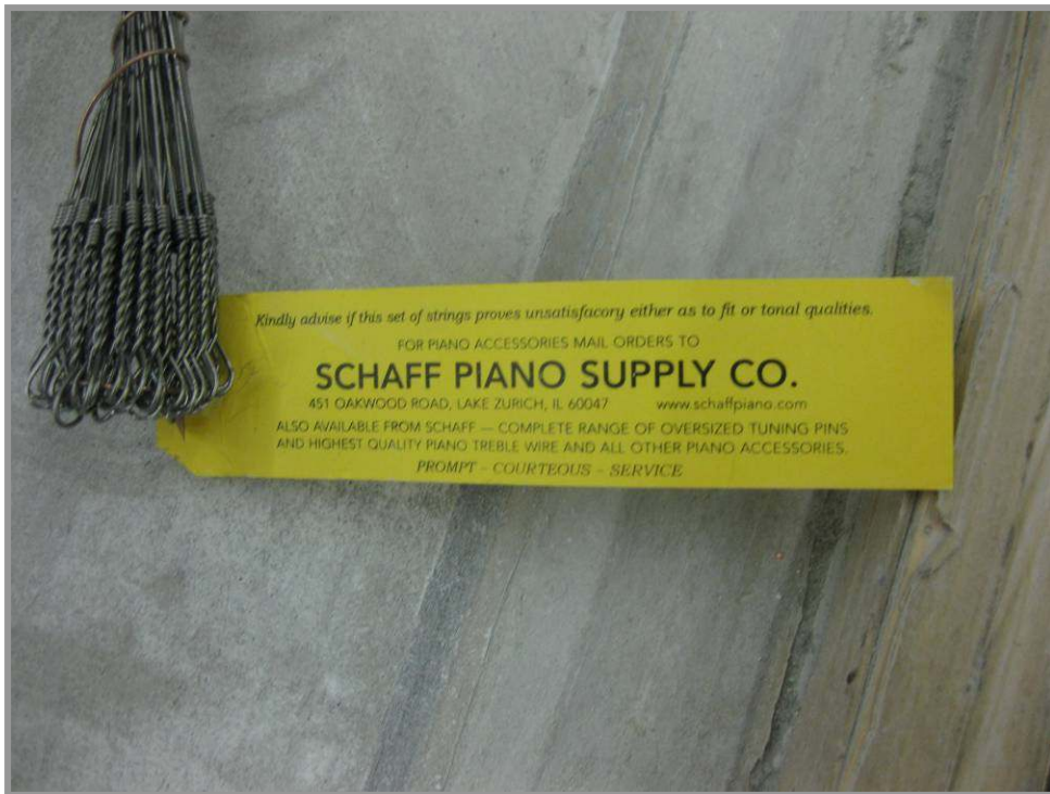
Photo 108: Once the set is complete, the string winder gives the set back to Ed to double check the dimensions with the scale. Once approved, he applies a copper tarnishing preventative and wraps up the set for shipping.
