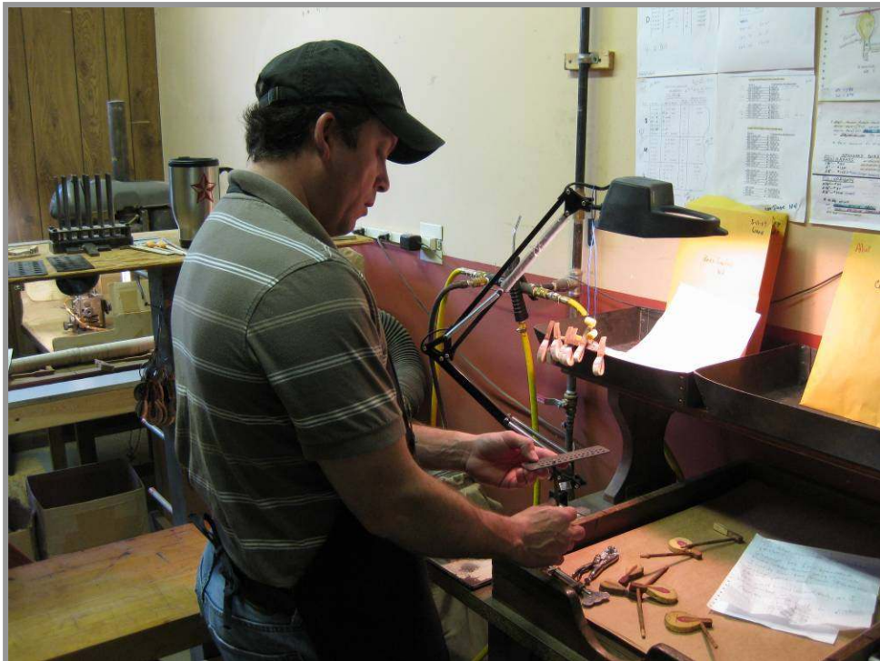
Photo 113: Joe uses a hole gauge to determine the shank diameter. If someone requests a snug or loose fit, he will make the appropriate changes in the drill size.
