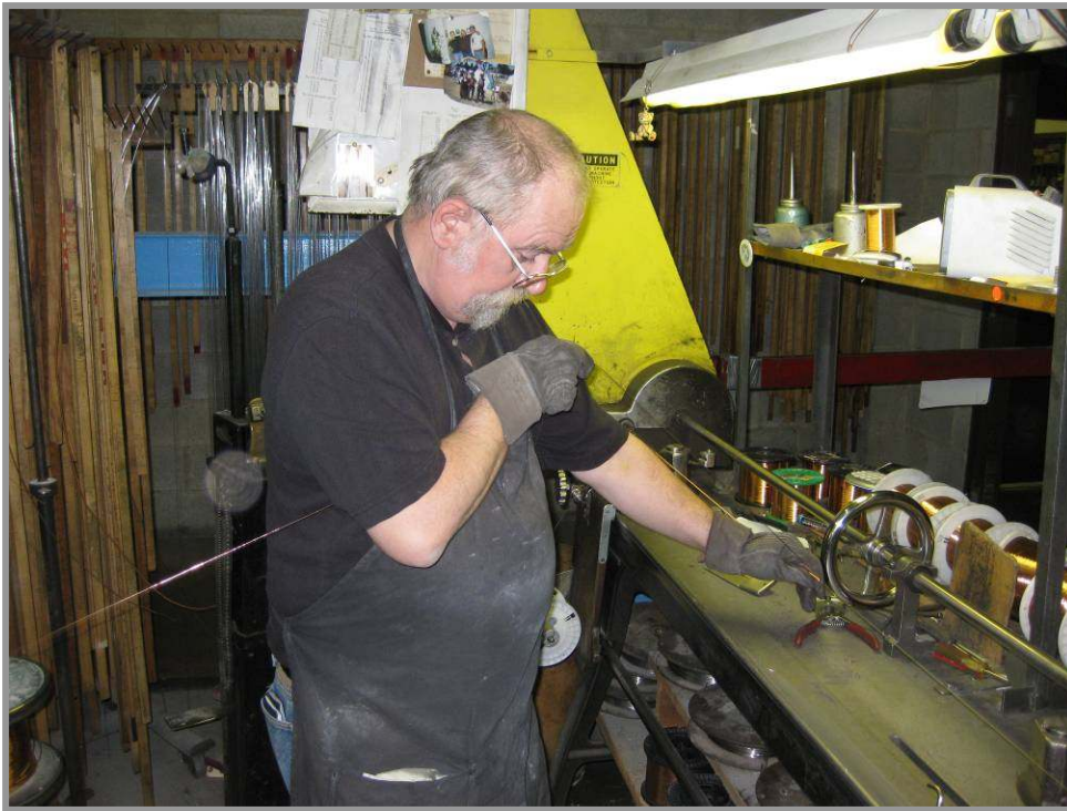
Photo 106: Tom Smith is hand winding a double wound string. This takes years of skill to master. It takes just the right amount of tension to make a great sounding/looking string.
