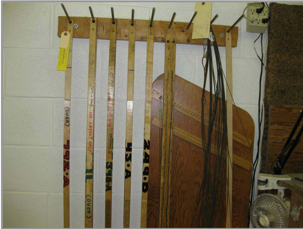
Photo 100: The scales are then hung up for duplication. The sets are made in order in which they were received. The string winders will then pull the scales and begin to make the sets of strings.
