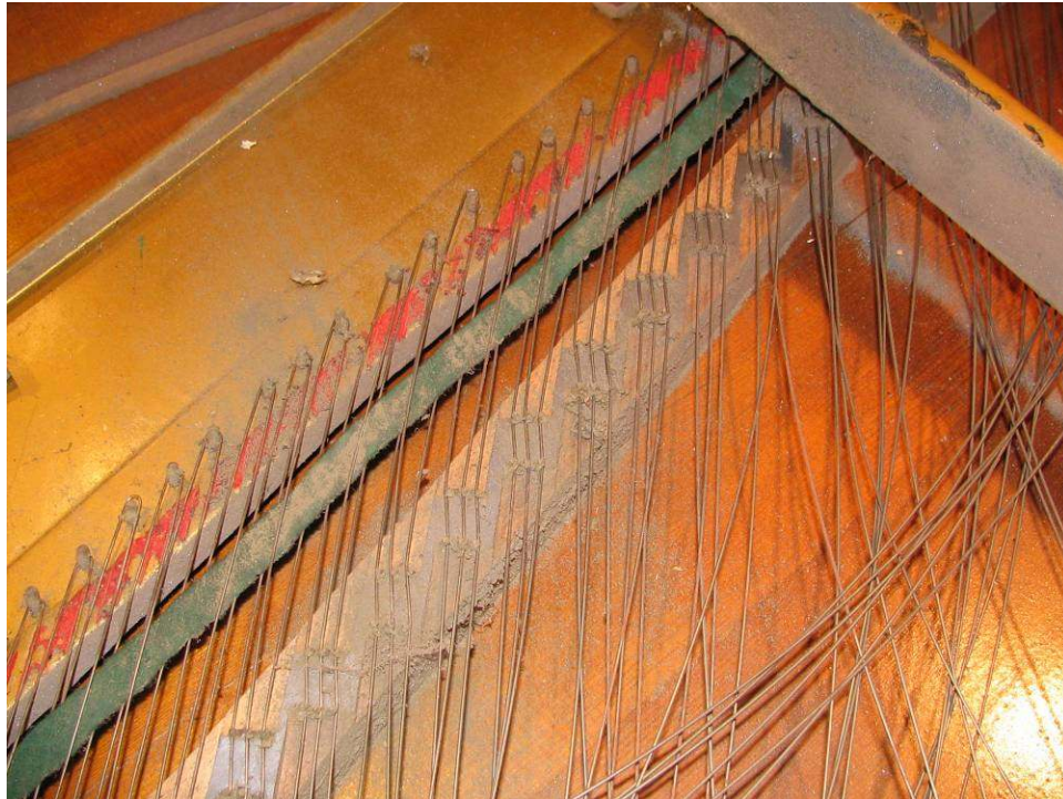
Photo 35: On the lower end, the strings are miked, then removed.
