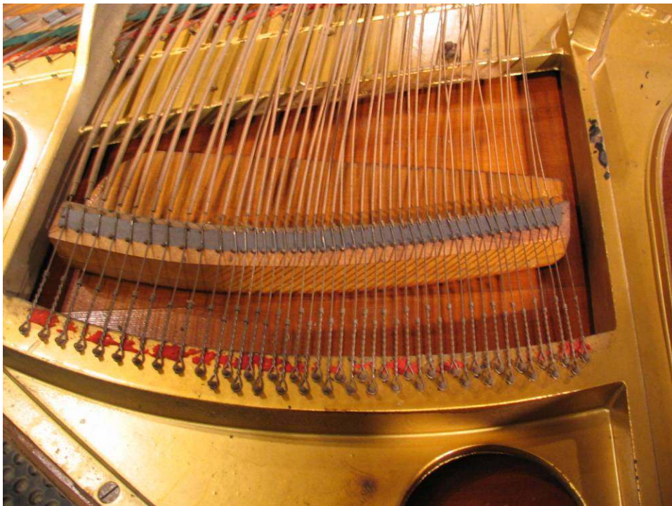
Photo 28: Although strings are slack over upper bridge, they are still attached to hitch pin and are still held by the lower set of bridge pins.
