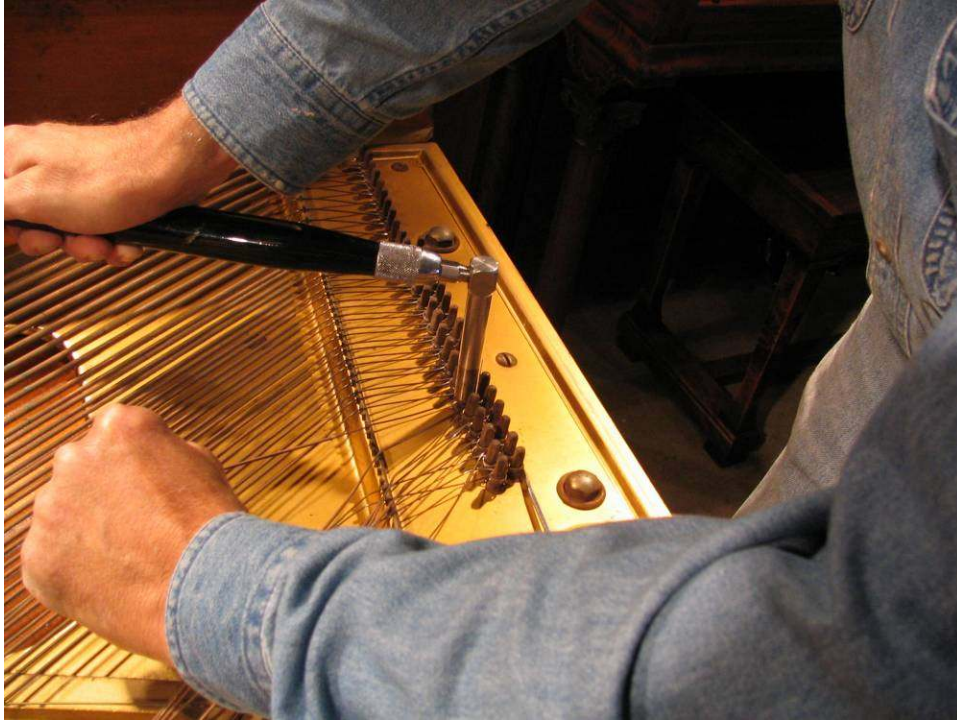
Photo 27: Bass strings are removed from upper bridge by further loosening tuning pin, and stretching string up and off of bridge pin.
