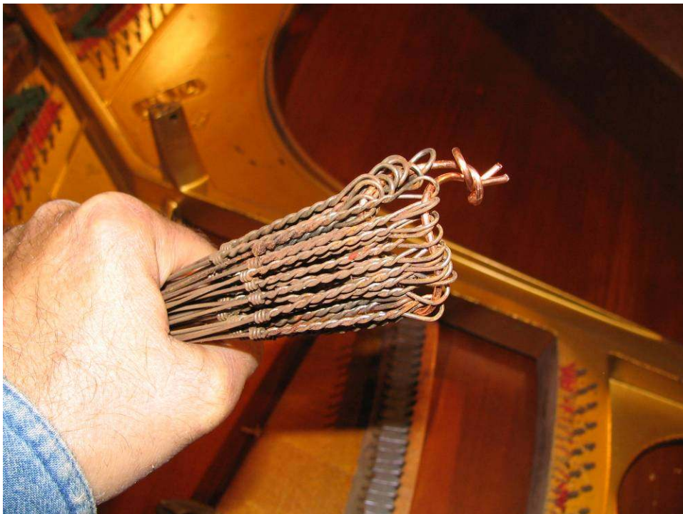
Photo 30: With all the strings removed, they are tied together with the copper wire through the loop on the end of each string.
