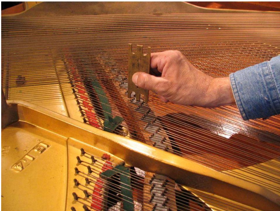
Photo 24: The bearing over the bridges feels normal.
