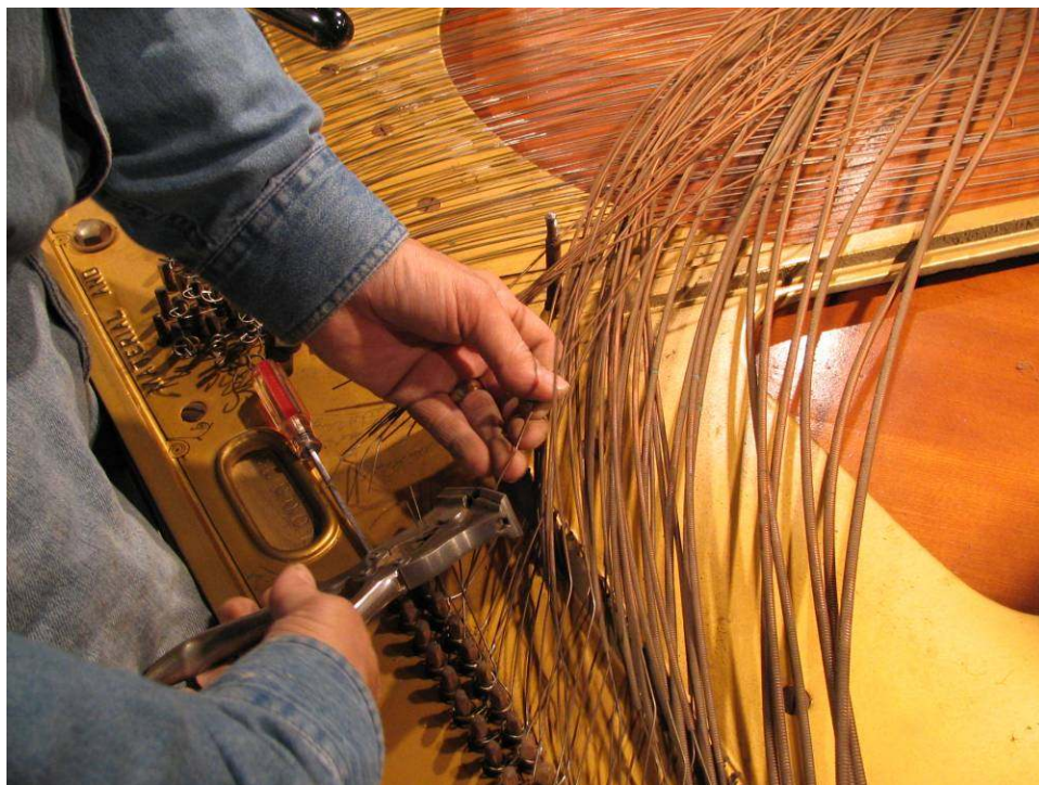
Photo 31: The strings are now snipped above the copper winding on the upper end. The entire set of bass strings is bundled in a loop, boxed and sent to the factory for duplication.
