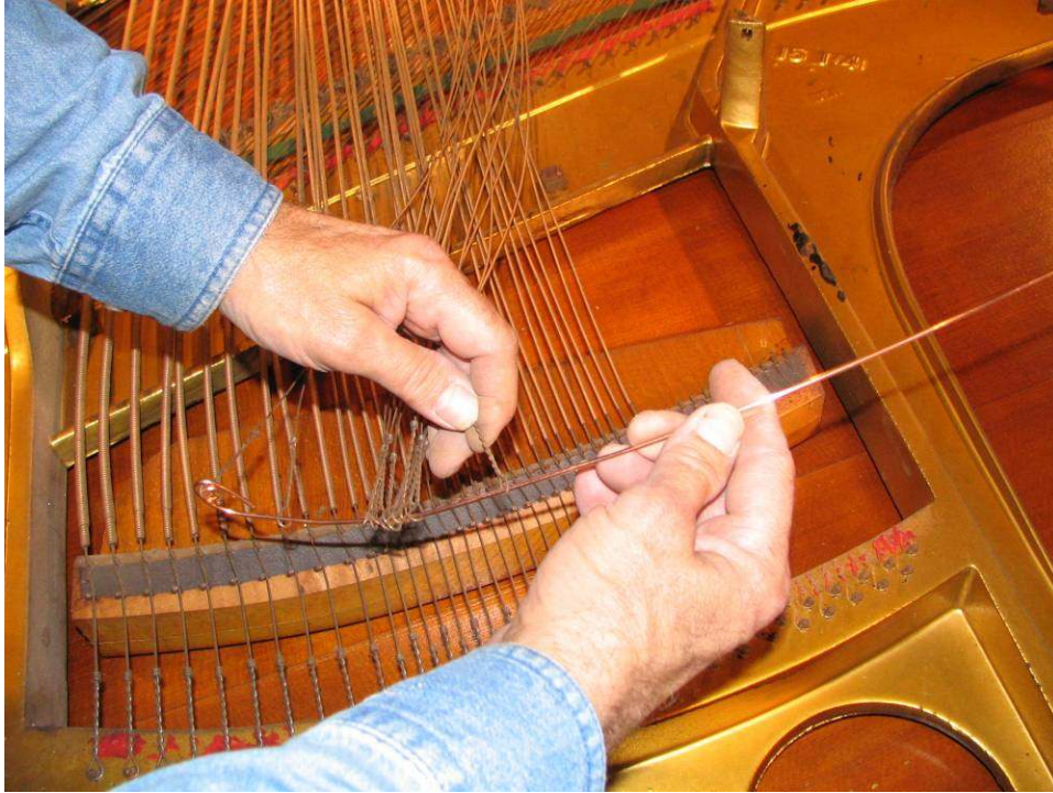
Photo 29: Starting from right, each string is removed from bridge and hitchpins by grasping and pulling up hard. Strings are then put in order on copper wire for shipping.
