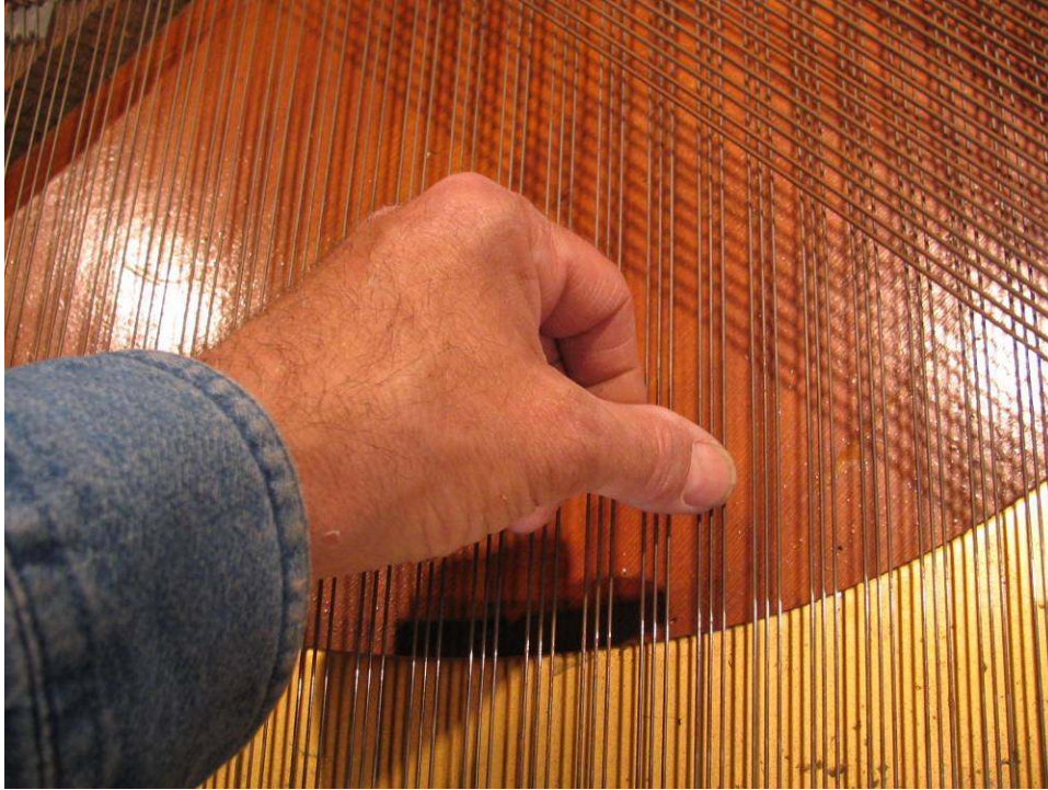
Photo 25: The “pluck test” reveals no extremely loose or slipping pins. Size 3’s should be adequate to improve overall torque.
