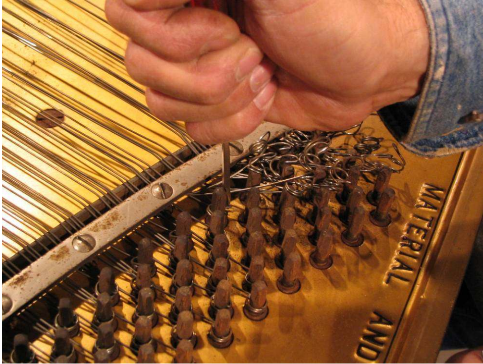
Photo 33: Treble strings are removed from pins. First the becket is pried loose with a small screwdriver, then a string hook is used to pull the coil from the tuning pin.
