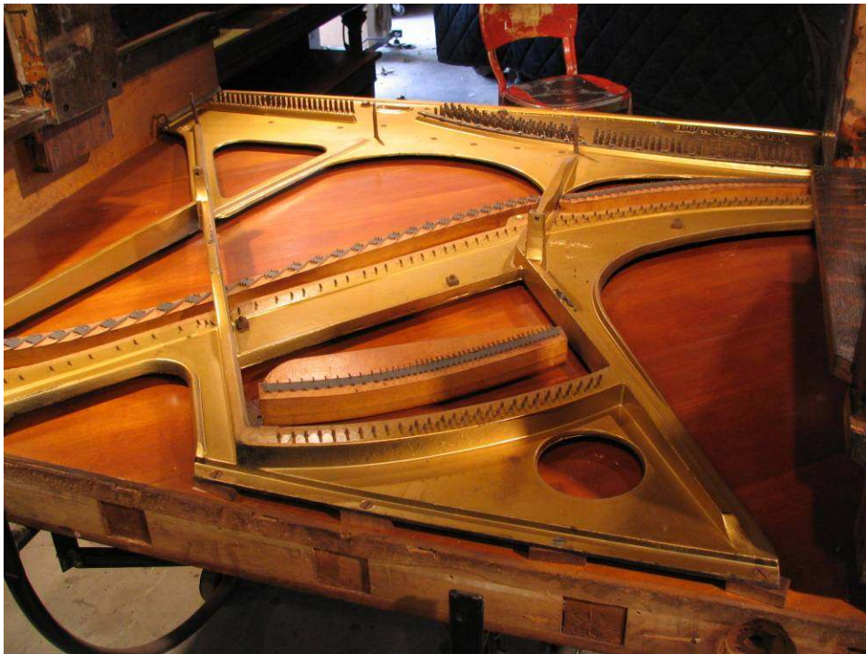
Photo 37: Piano with strings removed. Pins will be left in place until right before repinning and restringing.
