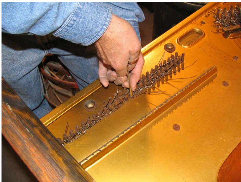
Photo 32: The coil is pried off the pin and discarded.
