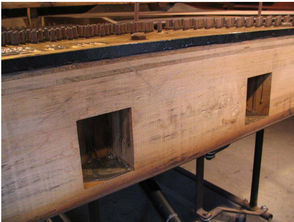
Photo 16: Back and pinblock that is rock solid – like it was built yesterday
