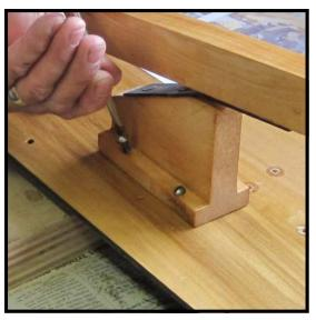
**Step 53:** With the pedals in place, screw the trapwork mechanism down once again to the pedal board.
