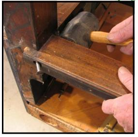
**Step 58:** To add the finishing touch to a pedal restoration job, the toerail may be removed for easy replacement of the felt around the notches for the pedals.
