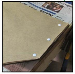
Step 12: If the decision is made to drill and plug the screw holes for either the bracket hardware or any other of the trapwork mechanisms, an accurate template of the exact position of the existing screw holes should first be made. Cut a piece of contractor's paper to cover the bottom board, and secure it on one end by tacking it firmly in place.
