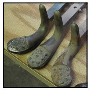
Note: Some pedals show potential for restoration, while others don't. This set of pedals from another piano is a prime example of a situation where new pedals are not necessarily called for. These have a lot of potential.
