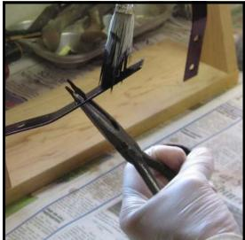
**Step 34:** A particularly good protective coating for metal springs and other similar hardware is Nu-Blue (Cat. No. 438), sold specifically for coating old tuning pins, but very functional for this use as well. Apply with a soft brush..
