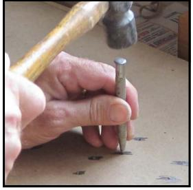
**Step 31:** Use a punch or scratch awl to tap in the location of the screw holes.
