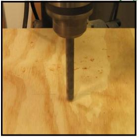
Step 18: Before drilling the holes for the dowels, set your drill press so that the depth of the hole will be nearly all the way through the bottom board, with just enough of the tip of the drill emerging so that excess glue has a place to escape. Select a size of drill to match whatever size of dowel you plan to plug the holes with. In this case a 1/4" bit was used to drill for a 1/4" dowel.
