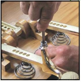
**Step 46:** Use your scratch awl to mark a center point for each of the conical springs.
