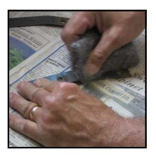
Step 33: With the pedal board itself prepared and ready to receive brackets and mountings once again, one's attention should be turned to the components of the trapwork mechanism. To begin with, trap lever springs which have minor corrosion may be cleaned and treated to prevent further damage. First clean off all rust and residue with Grade 2 (medium coarse) steel wool (Cat. No. 412-2).
