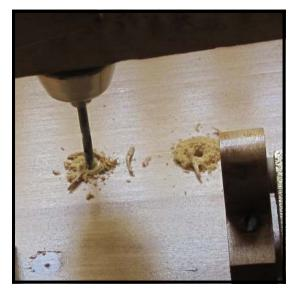
**Step 42:** Having verified the position for the brackets, drill the new pilot holes using the correct sized bit.
