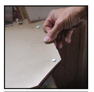
**Step 30:** With all the wooden parts refinished, the original location of the screw holes should be marked. Retrieve the template produced earlier, and tack it to the pedal board, using the same holes as before.
