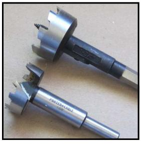
Note: Oftentimes sets of Forstner bits are sold with a 1 5/8" bit and a 2" bit, but not the in between 1 3/4" size. The smaller 1 5/8" bit will drill a hole that the spring will fit into, but it will be too tight and the spring will click each time the it is depressed, as the first two coils of the spring slide by each other. The slightly larger 1 3/4" bit will produce a hole with a slightly more relaxed fit, allowing the spring to compress in upon itself without any clicking noise.
