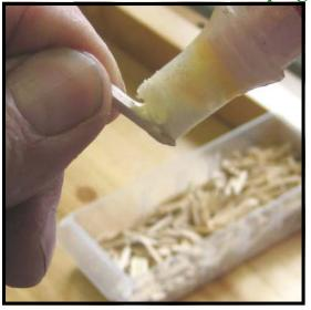
Step 37: If any of the screws in the trapwork mechanism seem loose, inserting a shoe peg with a drop of Titebond glue is a good idea. Insert the pegs into the offending holes (or simply do them all) and snip off any excess length. A pair of Maxi-Shear flush cutters (Cat. No. 215) work nicely for this job.
