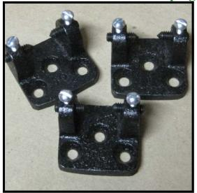
In some cases where the condition of the original brackets has deteriorated to the point where repair would be difficult or impossible, replacement might be a better option. These heavy duty pedal brackets (Cat. No. 2582) are replacements for brackets that don't use the fluted pedal pin.
