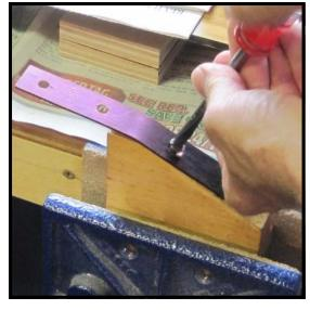
**Step 36:** When the treated springs or hardware is dry reassemble the trapwork mechanism before remounting on the pedal board.
