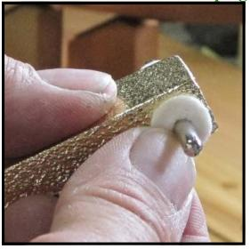
**Step 43:** Balance rail punchings (Cat. No. 332 C) work well on the pedal pin as bushings.
