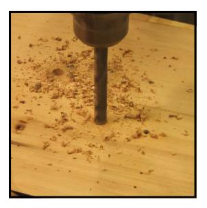
**Step 19:** Drill out each hole to the complete depth that the gauge has been set to.
