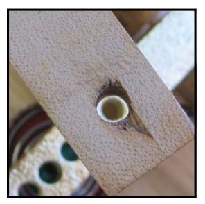
**Step 54:** Align the trapwork mechanism with the pedal by eyeballing down through the hole in the trapwork lever to find the nearest hole in the pedal.
