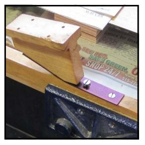
**Hint:** Attaching the trapwork spring to the underside of the trapwork lever is facilitated by placing the lever lengthwise in a vise.
