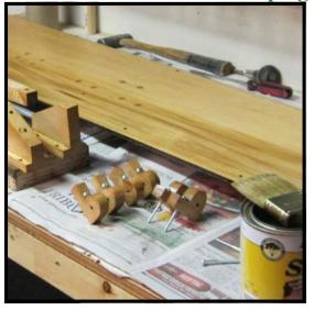
**Step 29:** After cleaning and sanding, all wooden parts should be given three coats of shellac for protection.
