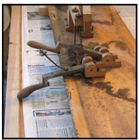
Step 2: Clear a bench top to locate the pedal board during the course of repairs. A careful inspection to determine what parts may be salvaged and what parts need replacing is the first order of business. If a new set of pedals are needed, now is the time to put in the order to Schaff so that the pedals are on hand when the time comes to install them. If pedals are ordered, check catalog specifications to ensure a proper fit. Schaff carries a wide selection of upright pedals to chose from!
