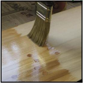
**Step 27:** Apply a topcoat to the pedal board. Shellac is an ideal finish in that it dries quickly enough that 3 coats may be applied in the space of a single morning or afternoon.
