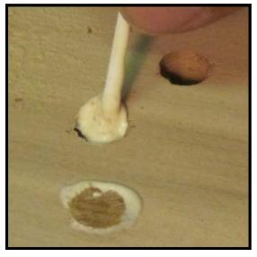
**Step 22:** Swab the each hole generously with Titebond using a Q-Tip.
