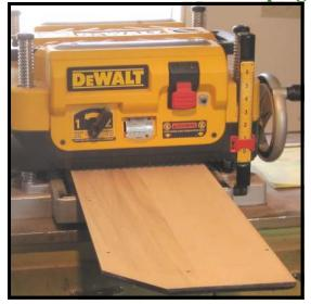
Alternative repair method: For those who don't want to be bothered with chiseling a number of dowels try running the pedal board through a thickness planer adjusted to just skim over the top of the board and plane the excess wood from the tops of the dowels.
