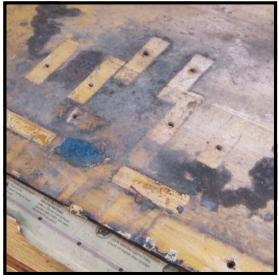
Note: For maximum cleaning and/or refinishing, continue disassembly until you've reached the stage illustrated on the left. It is obvious that trying to clean around the brackets and mounts would be much more difficult in this situation than simply cleaning the uncluttered pedal board minus all hardware as shown.
