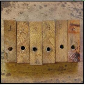
**Step 6:** With any parts for which there are multiples, number them in a spot that will be evident later. While it may not cause problems to interchange parts, it is always safer to simply return each part to its original spot.
