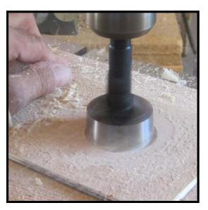
Hint: An easy to make template for perfectly sized felt discs may be made by using the 1 3/4" Forstner bit to cut a hole in a thin piece of stock.
