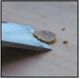
**Step 25:** Once the glue has dried adequately, shave the excess off with a sharpened chisel from your chisel set (Cat. No. 292).
