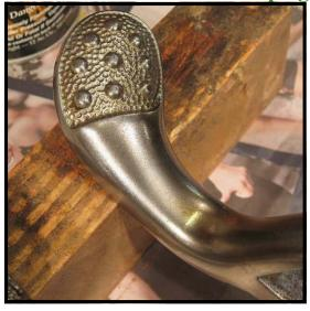
With the nickel plating thoroughly cleaned, the sprayed-on lacquer finish brings out the original beauty of the pedals.
