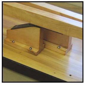
**Step 38:** With the trapwork lever mechanisms reassembled, screw them down temporarily to check functionality, then remove again (if necessary for upcoming steps) for the time being.
