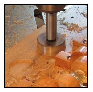
**Step 47:** Drill a shallow well for each conical spring with a 1 3/4" Forstner bit.
