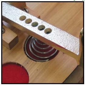
Step 52: Flip the pedals back into place, and check alignment with the springs. As a last precaution to prevent noise, a front rail punching (Cat. No. 337E) may be inserted in between the top of the spring and the underside of the pedal. Glue in place to the underside of the pedal with Titebond.
