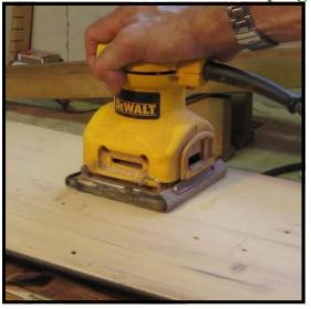
**Step 9:** With the bulk of the finish removed, switch to sandpaper to complete the job. Here, a hand sander is used with 60 grit paper on an initial pass over the bottom board to remove the remainder of the old shellac.
