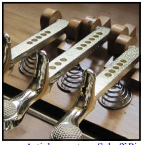
Step 45: Old springs are often broken or weakened with age and need attention. In the case of the example piano, the trap lever springs functioned, but seemed weak. An added spring which assisted the left and center pedal was probably not factory (see page 4). Conical springs (Cat. No. 586) were decided upon as an easy-to-install supplement to bolster spring strength. The location where the springs should be installed was here determined by positioning the springs under the pedals.
