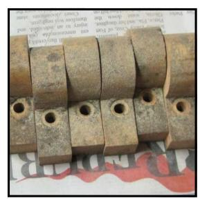
**Step 28:** If the old pedal brackets are to be retained, now is the time to focus attention to their condition. The brackets for this particular piano were good quality maple, filthy dirty, but otherwise in very useable condition. A thorough cleaning and sanding, followed by an application of 3 coats of shellac, was decided upon.
