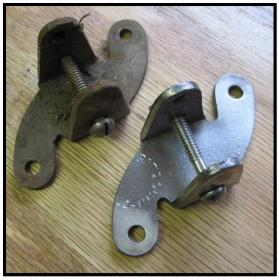
Note: In the case of certain metal pedal brackets such as those shown on the right from a different piano, a simple wire brushing followed by a protective coat of sprayed-on clear lacquer (Cat. No. 1438) is all that may be needed to bring the hardware back into like-new condition.
