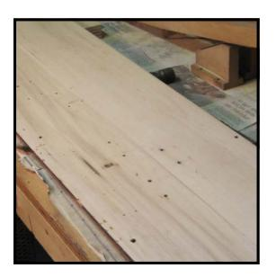
**Step 10:** Continue sanding by going through several finer grits (100, 150 and 220 are recommended) until a smooth board without discolorations is produced.
