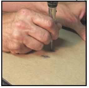
**Step 15:** To pinpoint the center of each hole, use the pointed end of a scratch awl (Cat. No. MF-365) to pierce the paper for each hole.
