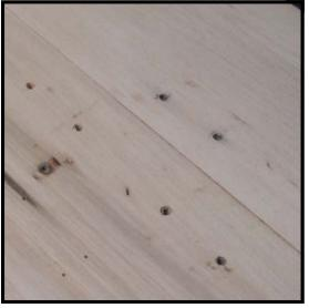
**Step 11:** Decide on a course of action for the bracket screw holes. Plugging with shoe pegs (Cat. No. 6050) and a touch of Titebond glue (Cat. No. 392-1) may be all that is necessary. However, for a more reliable fix, drilling out the old holes, inserting hardwood dowels, and drilling new tap holes (which will be discussed) is the preferred method.
