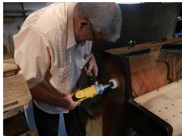
Photo 4: Dan Shere does ventilation holes.
