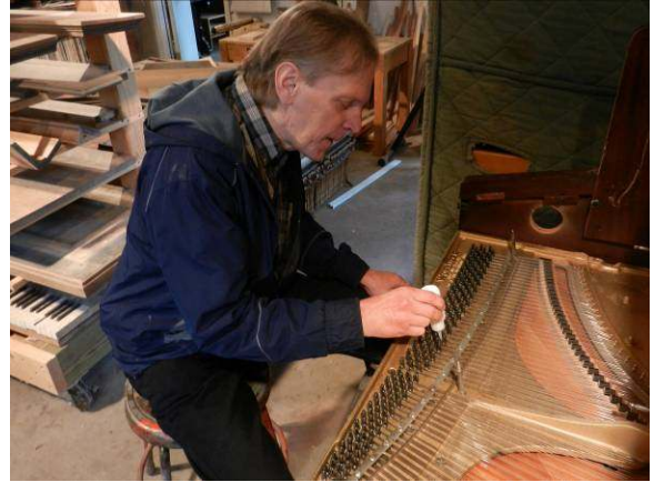
Photo 6: Steve Haag applies C.A. treatment to the pins.
