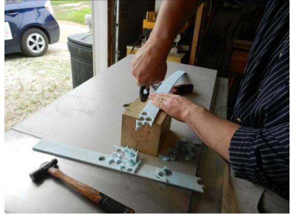
Photo 9: Dan Winchester cuts new punchings.
