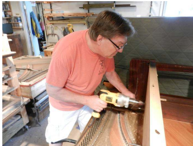
Photo 7: Roger Todd bevels the drainage holes.
