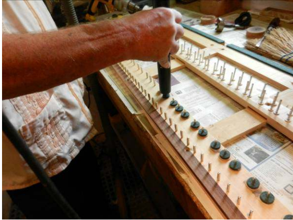
Photo 8: Dan Shere removes old punchings.
