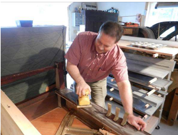
Photo 13: John roughs up the case parts.
