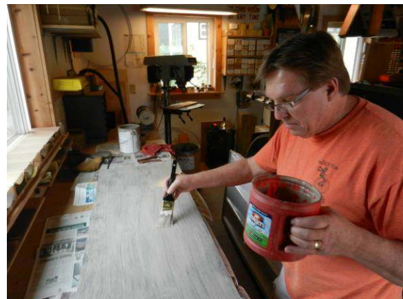
Photo 14: Roger applies the primer coat.
