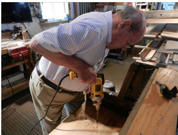
Photo 3: Harold Marling drills drainage holes.
