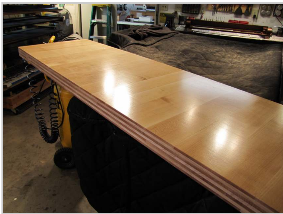
Photo 97: By the end of the week (after the chapter meeting) all three of the pinblocks have arrived, and they are each a beautiful work of craftsmanship. Shown in this photo is a gorgeous 7-ply 2" thick pinblock sent by WNG.
