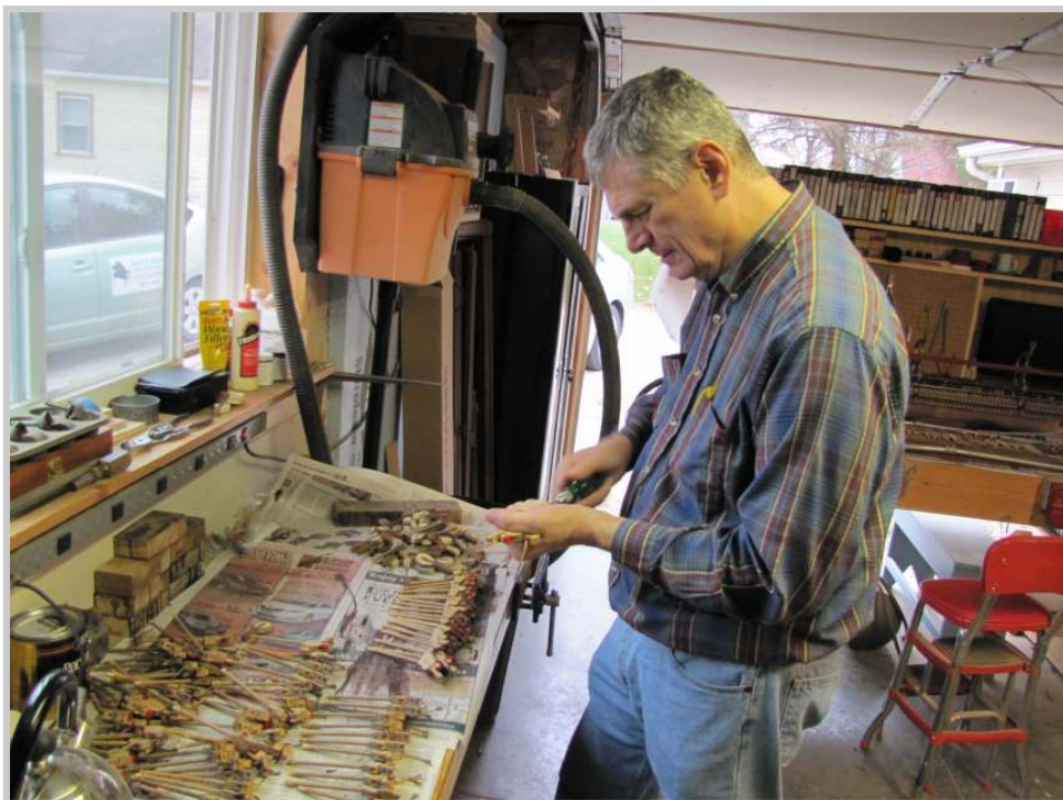
Photo 88: With all the hammers removed, David takes a turn at the bench, using a hammer shank reducer to remove the 100 year old remnants of hot animal hide glue.
