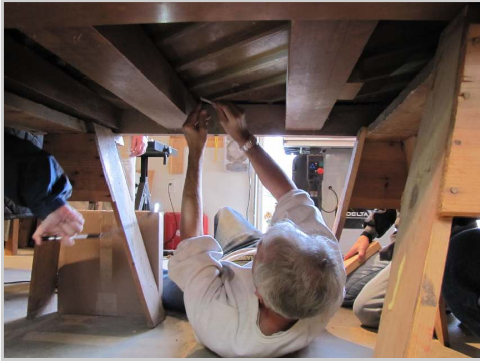
Photo 94: Realizing that the entire bridge will need to be removed, I make myself useful for the first time of the day, and crawl under the piano to remove the screws holding it in place. One of them, being conveniently located behind a post, requires an off-set screwdriver to remove - the type of tool you don't need on a regular basis, but when you do, nothing else will work.
