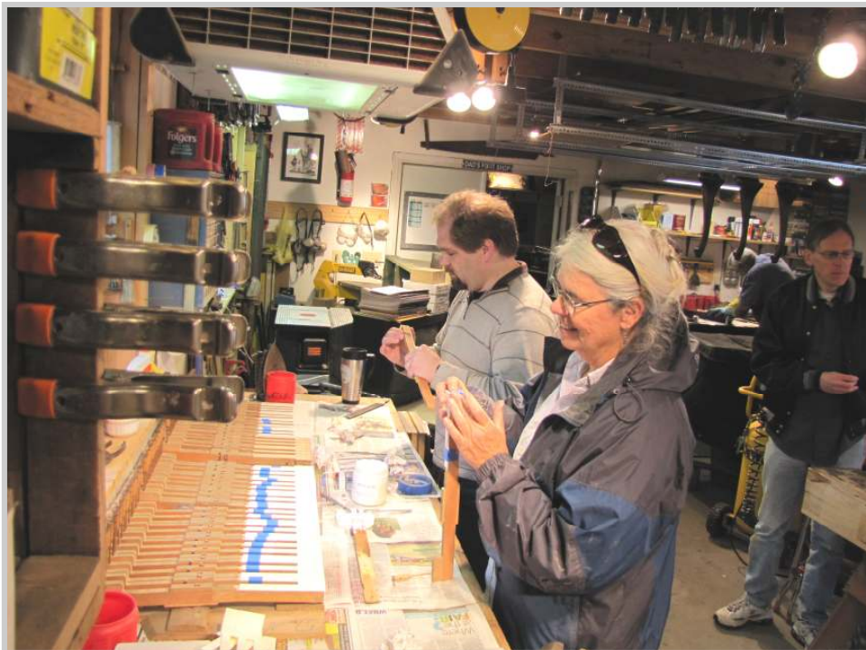
Photo 92: Don Winchester (with the beard) and Annie Greishop (sunglasses) work at the keytop replacement bench gluing new German keytops from Schaff onto the prepped surface of the keysticks using PVC-E glue. All the keytops were glued, and are now ready for filing.
