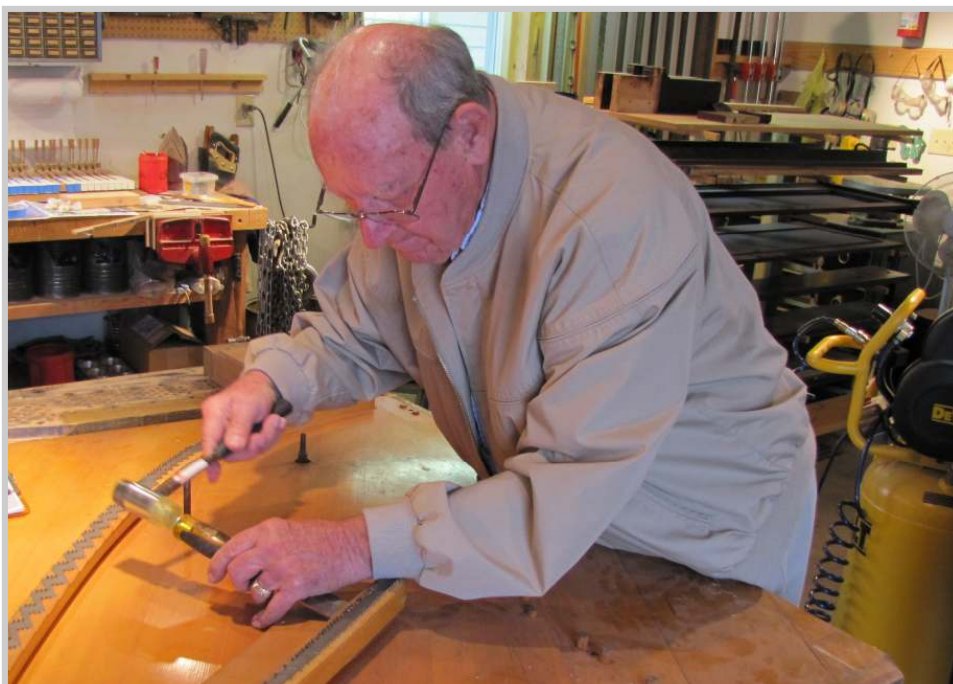
Photo 93: Harold Marling offers to lend his expertise in bass bridge duplication. I agree that he can take the bridge home to his shop on one condition - "Take lots of pictures!" We'll just see if he comes through with them or not. Here he makes an initial attempt to pop off the top portion of the bridge.
