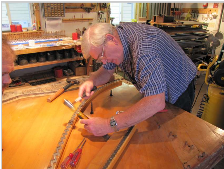
Photo 95: Dan finishes the job, removing the entire bridge assembly with several smart blows from the mallet to the large chisel.
