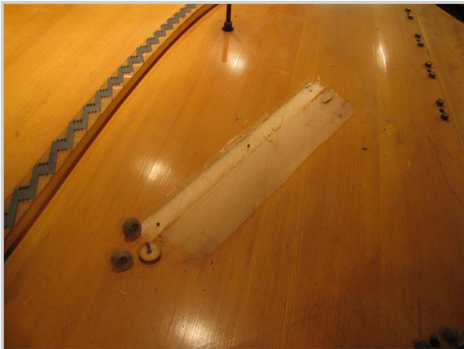
Photo 96: The bass bridge comes free with minimal damage to the soundboard.
