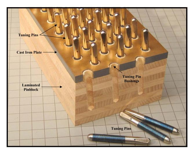
The above cut-away model of a piano pinblock, plate and pins illustrates the origin of the problem. The pinblock is made of hardwood, in this case hard rock maple. Its laminations run cross grain to each other to prevent splitting, and to better hold the tuning pins. The pinblock is not ordinarily visible, but is hidden beneath the cast iron plate, which is necessary to hold the tremendous tension on the strings, measuring anywhere from 18 to 20+ tons for the piano as a whole.
