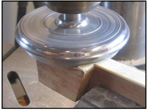
milling down process gives a completely flat surface on which to glue the new keytops.
