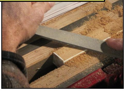
files to produce an edge which is perfectly flush to the wooden keystick. When done correctly, there will be no overhanging edge along the sides of the keys.
