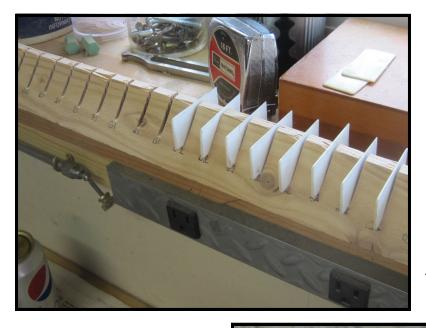
In situations where keytops are loose to the point where they are popping off unexpectedly, the only real solution is to remove them all, (usually both heads and tails) to reglue with proper methods that will ensure they stay put in the future. This is one potential aspect of the job which would add a great deal of shop time to the job.
