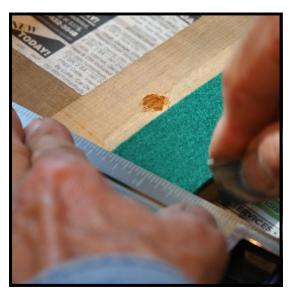
**Step 14:** Use either a felt cutting knife (Cat. No. 213), a square end knife (Cat. No. 216) or a single edge razor to cut the backrail cloth around the notches in the keyframe that fit around the supports for the action brackets. Either knife gives the advantage of a easy-to-grasp handle, that the razor blade does not.
