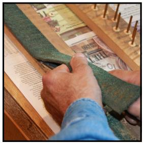
**Step 6:** Remove the backrail cloth. Sometimes the old glue has deteriorated to the point where the strips of felt may be simply pulled off. In this case, a 1" chisel from chisel set (Cat. No. 292) was used as the felt strip was pulled upward.
