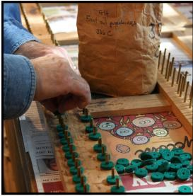
Step 11: After measuring the thickness of the old front rail punchings, select new punchings to install. Front rail punchings in white cloth, (Cat. No. 331), kelly green cloth (Cat. No. 335) and dark green cloth (Cat. No. 336 and 336) are available in two widths (3/4)" and 7/8") and a range of thicknesses. If you do much of this work, you'll find that it's convenient to have a selection on hand to avoid having to wait to get to a job while supplies are ordered.
