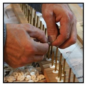
Step 12: Select and install new center rail punchings to match the punchings that were removed. Center rail punchings (Cat. No. 332) are available in five thicknesses. Push the new punchings down on the center rail using two thumbs as shown.
