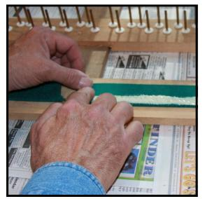
Step 17: With your finger, spread the glue on the half of the felt nearest to you. Do not get glue on the other half of the felt.
