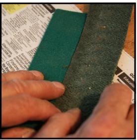
**Step 13:** Select the correct thickness of backrail cloth by comparing the thickness of the original cloth with the new. Lay a piece of the old side by side with the end from a new roll to determine which thickness is the best match.
