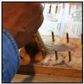
**Step 9:** Use a stiff brush to clean off as much residue around the front and center rail pins as possible. An effective brush may be made by taking an old varnish brush, and chopping off all but an inch or so of the bristles.
