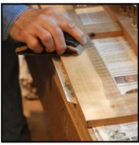
**Step 8:** With all the glue scraped off, finish the job with a sanding block and 60 grit sandpaper.
