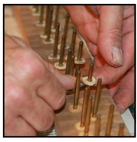
**Step 5:** Repeat the process with the center or balance rail punchings and the underlying leveling papers. Again, if a overall regulation of the piano is not in the plan, you may leave the leveling papers in place, although you still may want to at least relevel the keys by bringing all the keys up to the level of the highest key.
