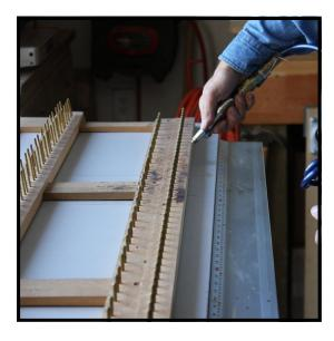
Step 10: Use a stream of compressed air to finish the cleaning process. If front and center rail pins are to be polished, now is the time to do that procedure.
