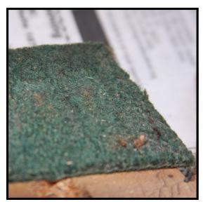
**Step 3:** Backrail cloth that is hard or coming loose on the front also needs replacement. A properly installed backrail cloth will not have been glued down in the back, so looseness there is to be expected
