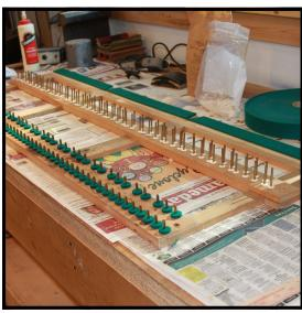
**Step 19:** Turn the keyframe back around in preparation for returning refelted frame to piano. If shims were removed from between the keyframe and the keybed in the disassembly process, return them to the correct position now and place keyframe back in piano.
