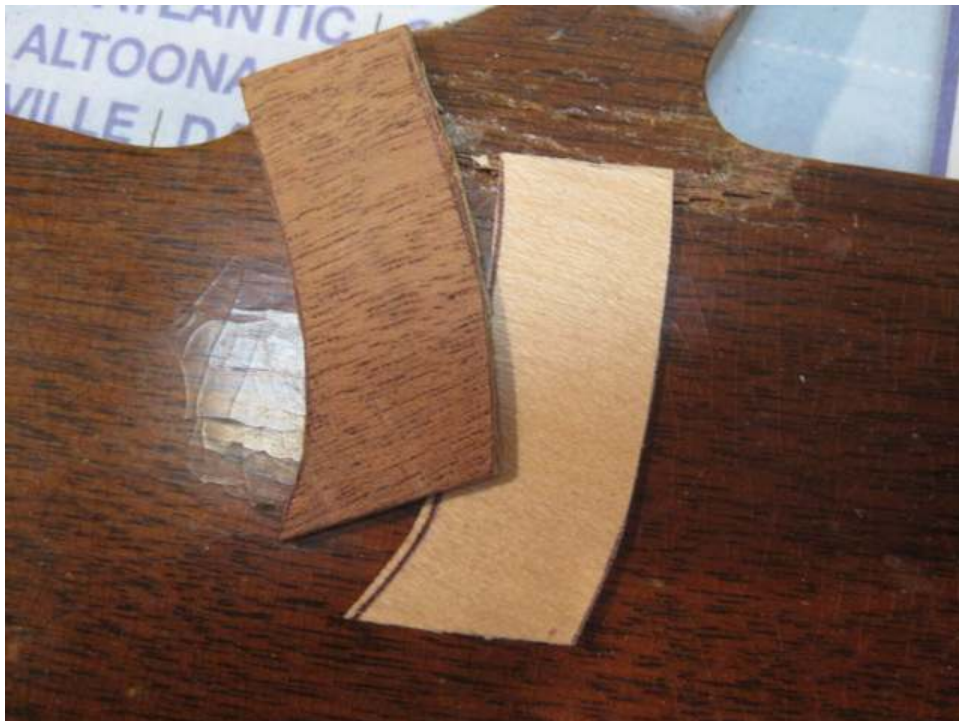
Photo 35: For the correct thickness, two layers of veneer are needed.
