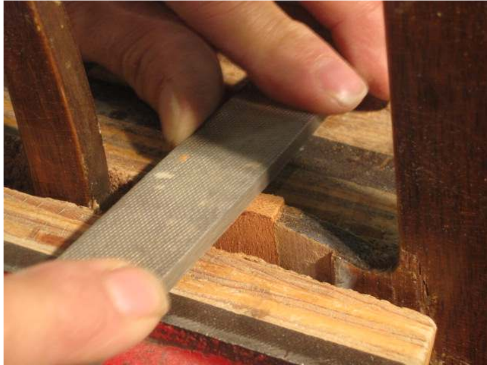
Photo 32: After rough cutting, the remaining excess is filed off, then sanded to a smooth finish
