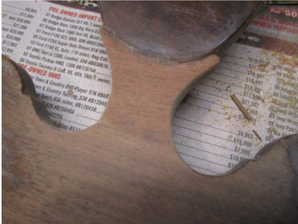
Photo 36: The middle support, with new veneer in place.
