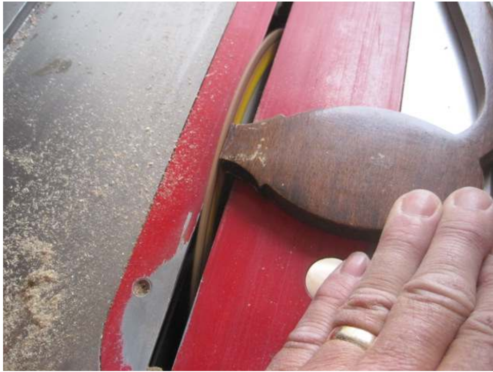
Photo 26: Each of the six broken edges is trimmed off on the table saw, removing as little wood as possible, but enough that a flat surface is achieved.
