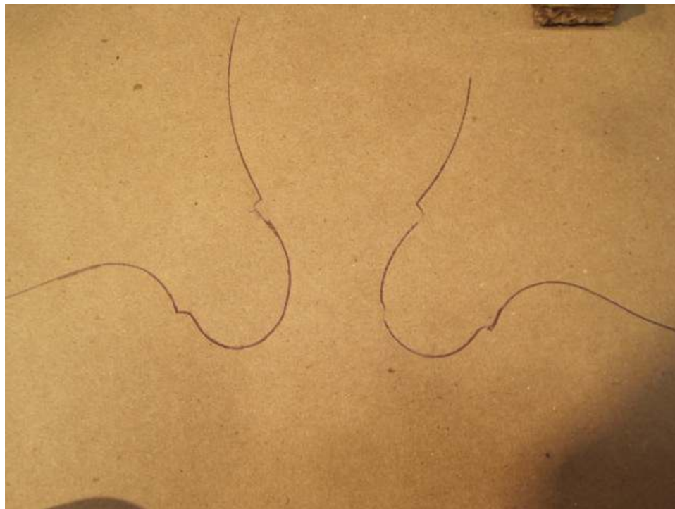
Photo 25: Before going any further, patterns were made of the profile of each of the three support sections.
