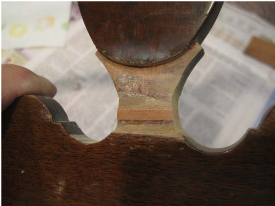
Photo 33: The middle support, with its core wood repaired, ready for new veneer.
