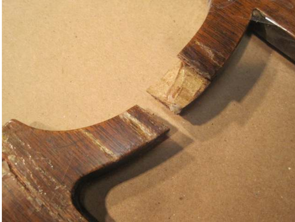
Photo 21: I decided it would be better to see what could be done with the old rack. The damage was compounded by the fact that repairs had apparently been attempted before. Old glue made a perfect fit impossible. Here's the condition of the left support.
