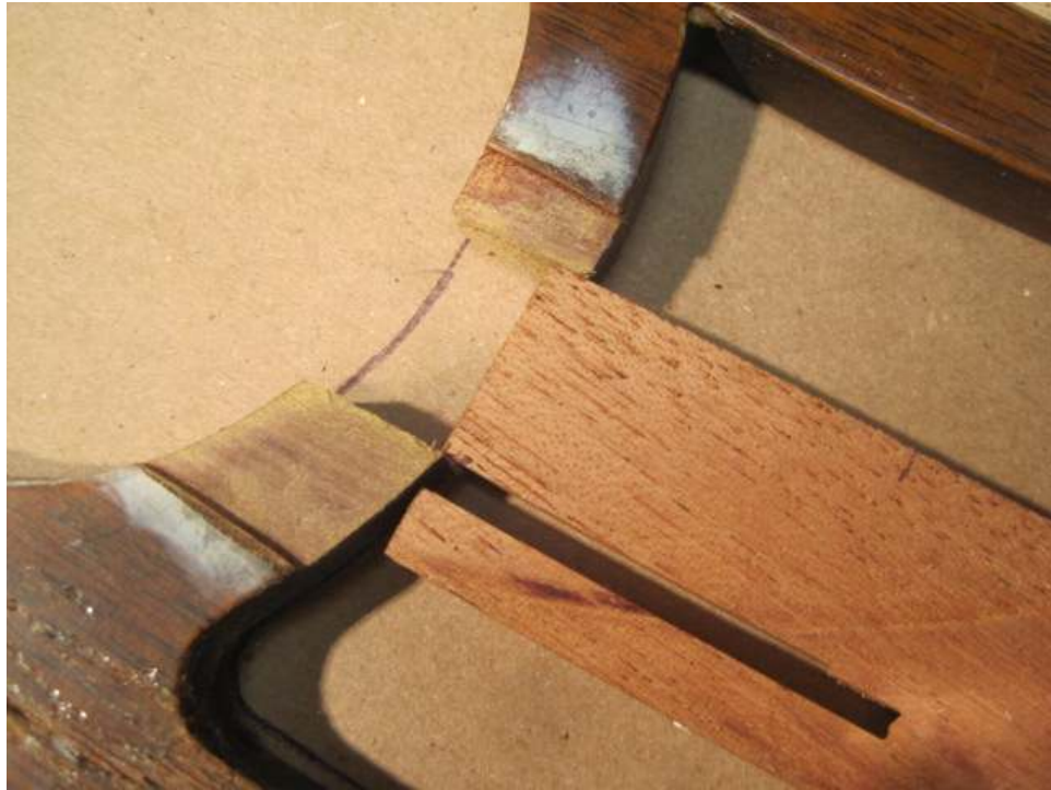
Photo 28: Here, a test cut in a block of mahogany is checked for correct dimension.
