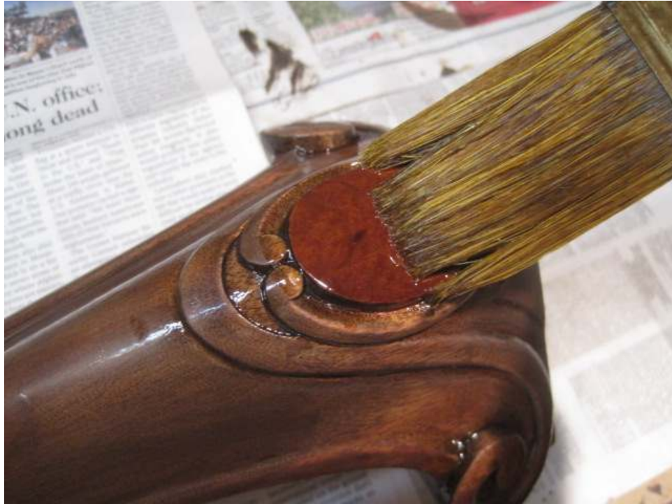
Photo 38: Meanwhile, the legs have been finished. Here, one of 6 coats of polyurethane is applied to the repaired leg.
