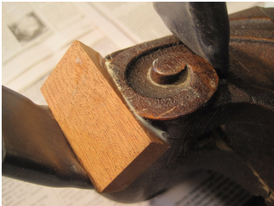
Photo 8: A block of mahogany is used to fill the gap. The excess will be trimmed. Mahogany is ideal for this type of work – easy to work and takes a variety of stains to blend in.
