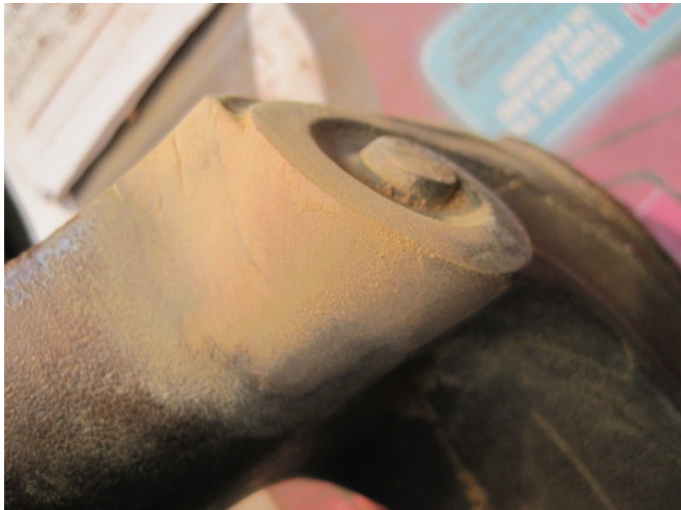
Photo 12: The patch is then sanded to blend in with the original surface.
