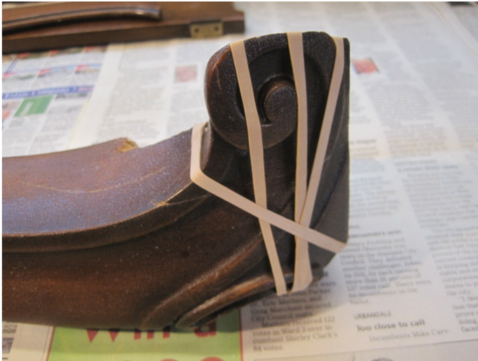
Photo 3: For small, uneven shapes, nothing works so well to clamp two surfaces together as simple rubber bands. Try doing this with a C-clamp!
