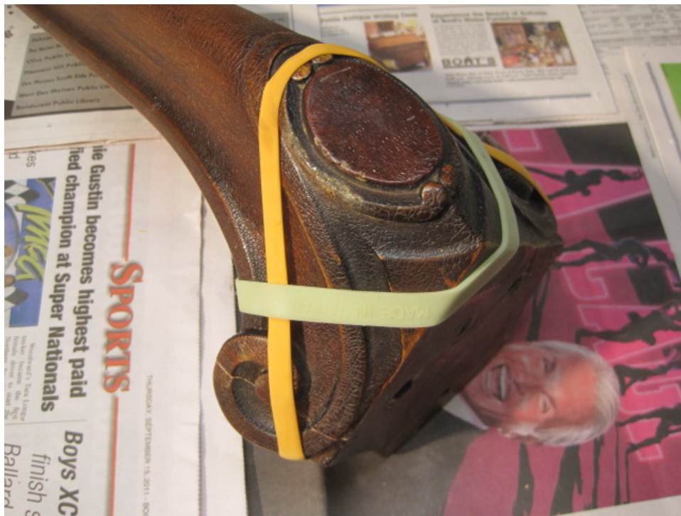
Photo4: After the small chunk has set, the larger piece is glued into place. These wrist bands fit the bill for this job.
