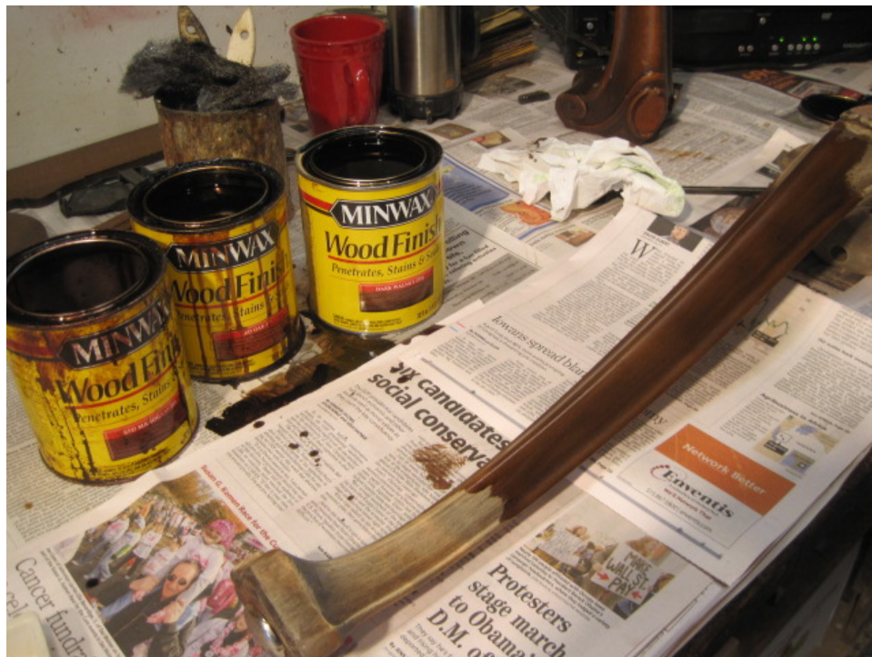
Photo 16: Staining to match begins. Several shades are used to duplicate original coloring.
