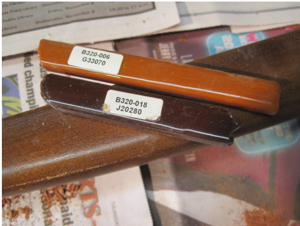
Photo 13: Potential lacquer stick colors for filling the small damaged areas on the back of the leg.
