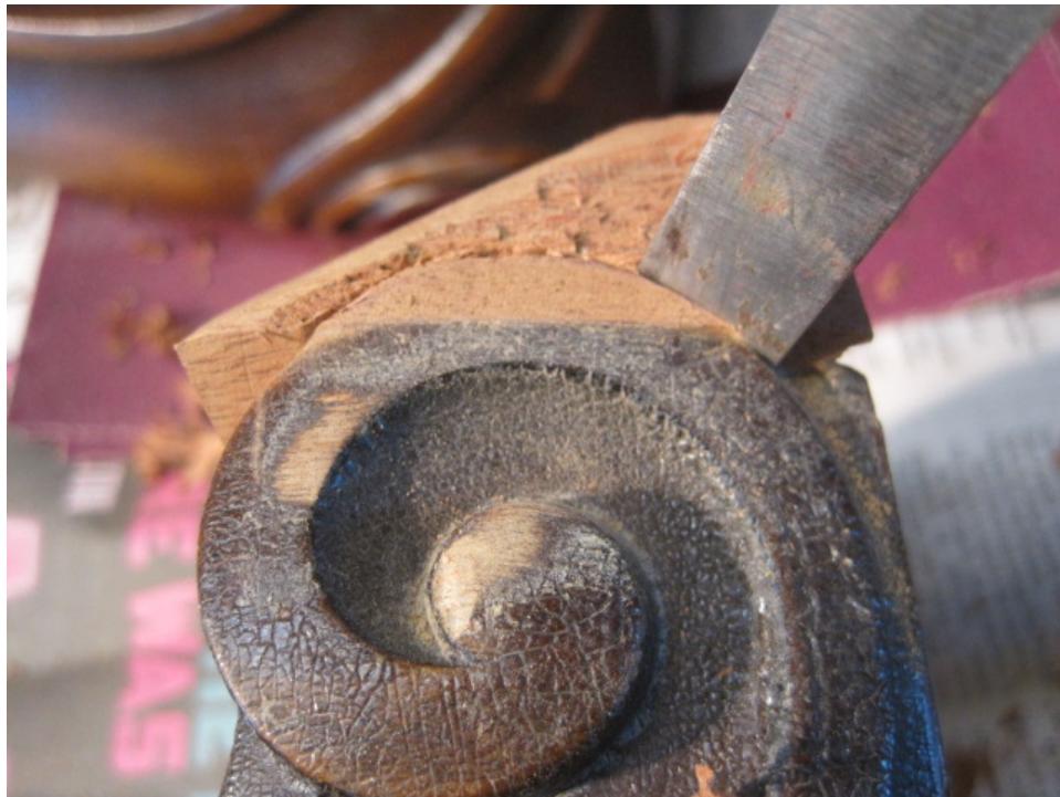
Photo 10: A chisel is used to start cutting away the excess.
