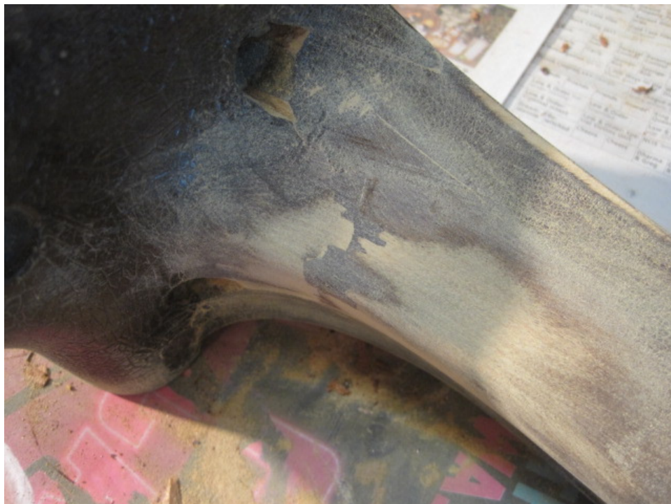
Photo 14: Staining will help blend in the patch. The wood will take the stain, the lacquer stick won't.
