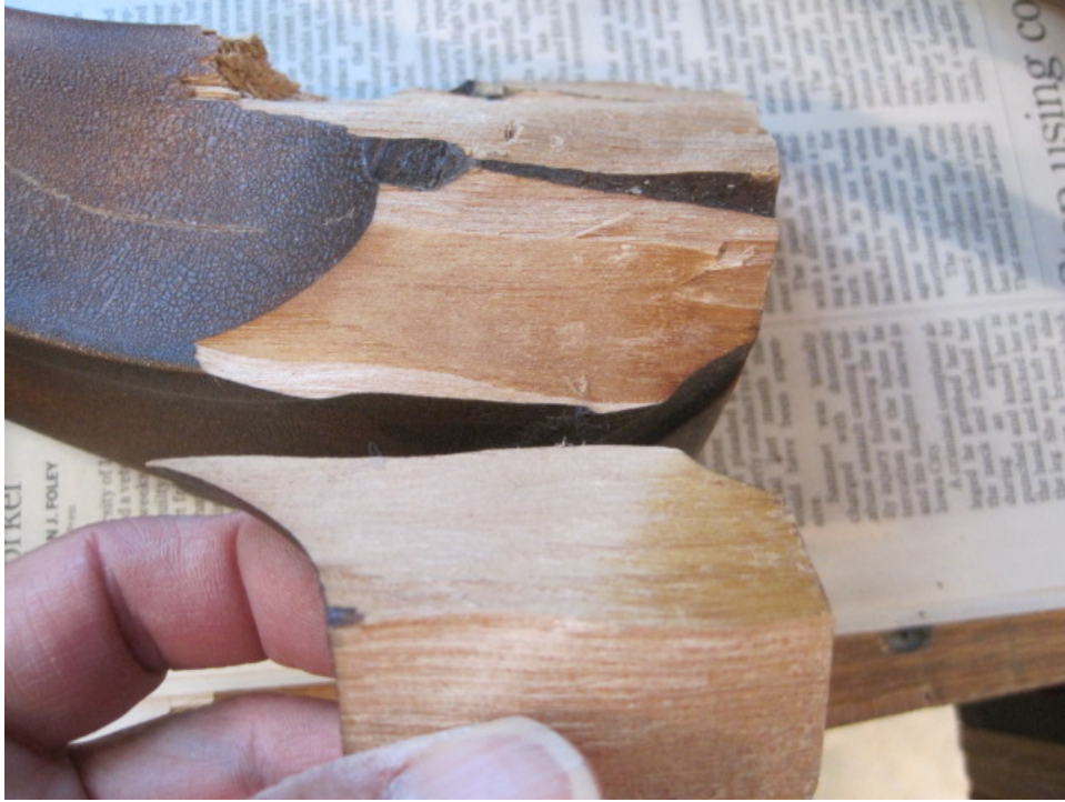
Photo 1: The bad news is of course the damage to the leg sent for repair. The good news is the break is clean, and that previous failed gluing attempts do not need to be dealt with.
