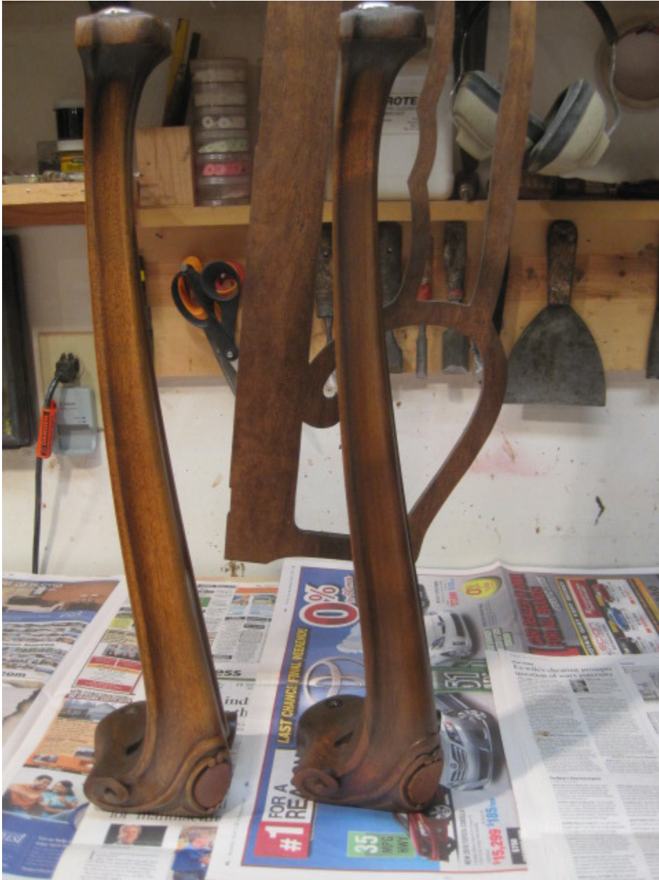
Photo 19: Both legs, stripped and stained, and new music rack hanging in the background. The stain will be allowed to dry 24 hours before the first coat of finish is applied.
