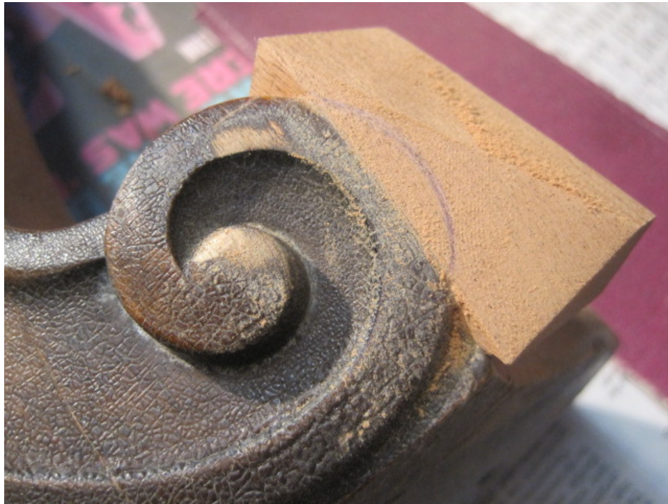
Photo 9: After a block plane is used to even the top surface, the curvature of the curl detail is marked in.
