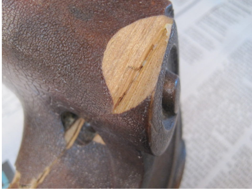
Photo 5: A missing chunk of wood on the corner makes the job interesting.
