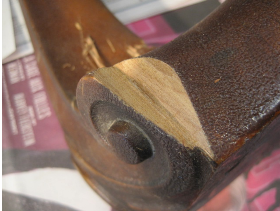
Photo 7: With a couple careful passes over the table saw, the damaged area is squared out.
