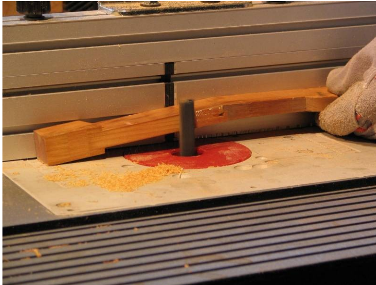
Photo 4: Using the router to surface the keytop.
