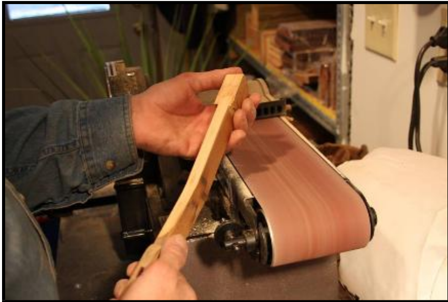
Photo 2: Used with care, old glue may be quickly removed.
