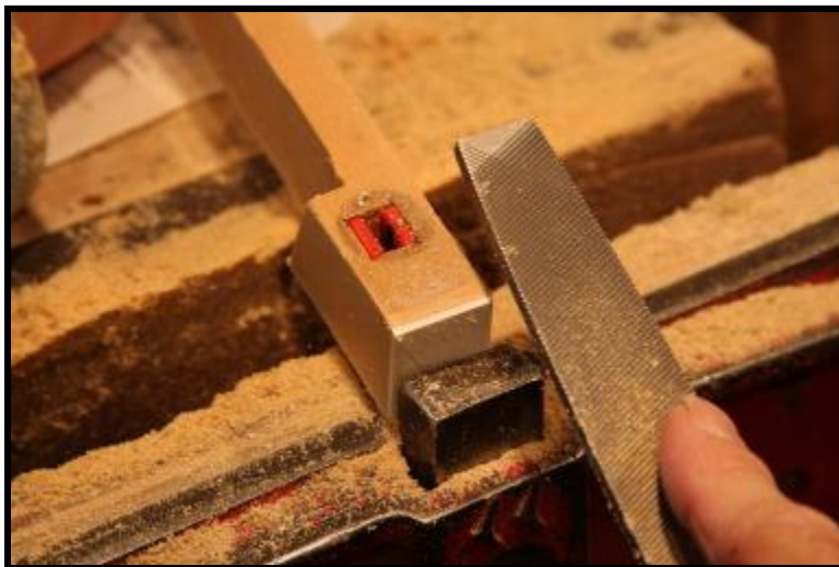
Photo 30: Finishing the bottom of the keyfront.
