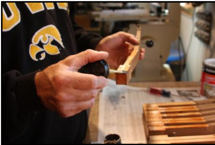
Photo 14: Applying second coat of contact cement.
