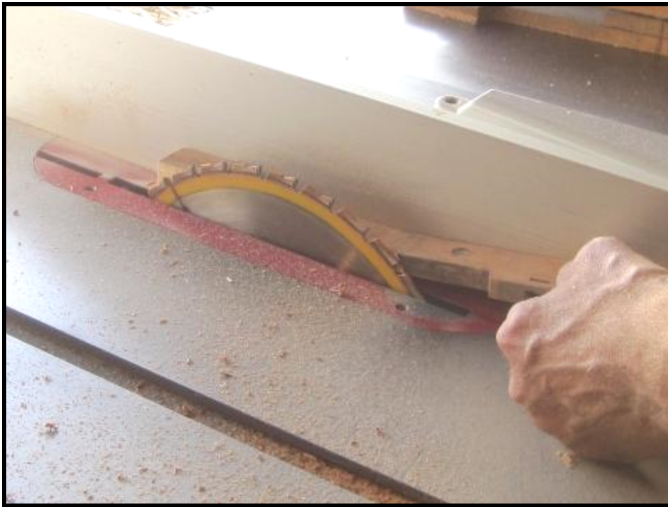
Photo 6: Blade too shallow - this would produce an uneven cut.
