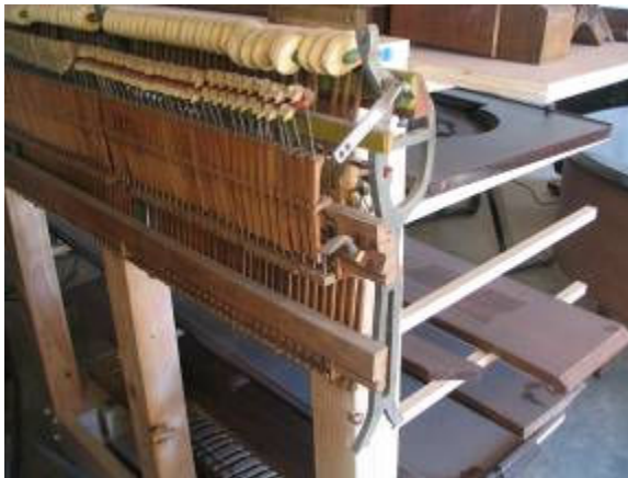
(TOP LEFT) Shelf on top provides storage for small parts. (TOP RIGHT) Removable grand damper holder. (BOTTOM LEFT) Bolts on back provide hanging spot for upright action.
