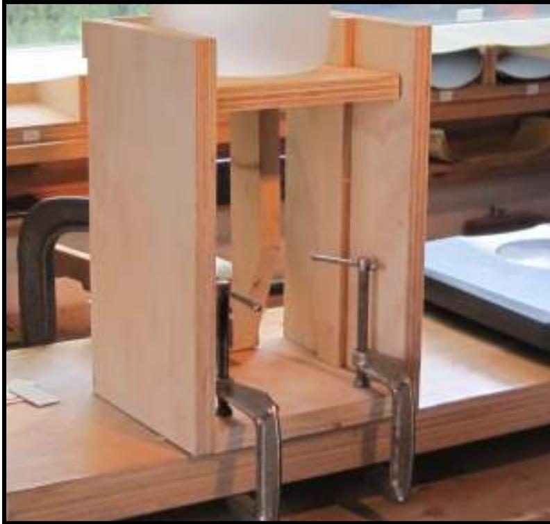
Knowing that many technicians would be disinclined to just take my word for this, I spent the better part of a day testing to verify the importance of this step. I built the device on the left to measure the adhesion of keytops which had been recovered using both cold and hot brass plates. I also tested various time periods for letting the glue set, to see if that made a difference as well.
