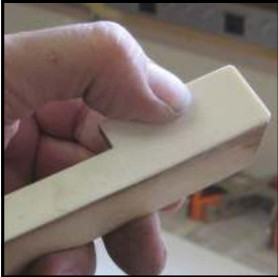
**Step 33:** Test the fit. The head and the tail should mate together with a nearly imperceptible seam. If not, try a bit more scraping and sanding.
