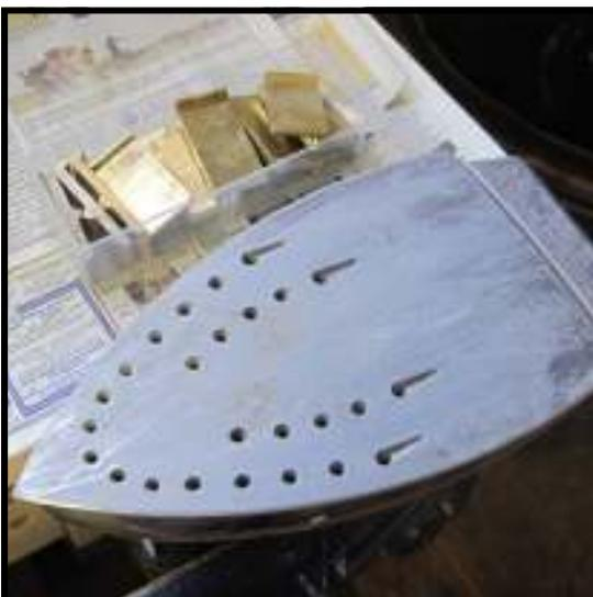
**Step 41:** Finally, position your shop iron flat-side up in a bench vise turned on to a medium heat. Have a supply of brass head plates in close proximity to the iron.
