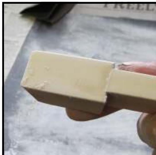
**Step 61:** Check your progress at the juncture between the head and the tail frequently to avoid over-sanding. In the photo to the left, the ivory powder which has caked to the left of the tail indicates that the tail is still a trifle high compared with the back of the head. Also, the portion of the head butted up to the tail appears as if it has not to this point been touched by the sandpaper. A bit more careful sanding is in order.
