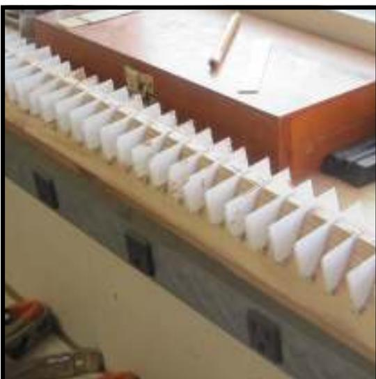
**Step 26:** Once all of the keysticks are prepared (if you are in fact regluing all the keytops), turn your attention to the ivories. Make sure that the set of ivories is complete, with all missing keytops filled in with acceptable substitutes from your collection of used ivory .
