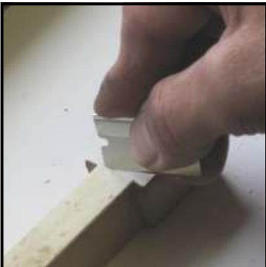
**Step 10:** For keys with a linen backing, first slice the fabric with a sharp razor along the front edge of the tail.
