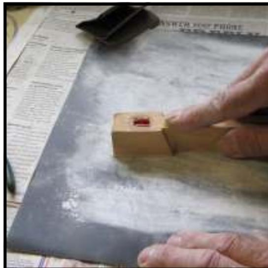
**Step 60:** Place the grits of sandpaper you are going to use face up on your bench, and sand the ivory by holding the keystick face down as shown. If unevenness between the head and tail exist, start with 400 or 500 grit, and sand until the joint is smooth. Then switch to the 800 grit paper to remove the sanding marks of the coarser paper.
