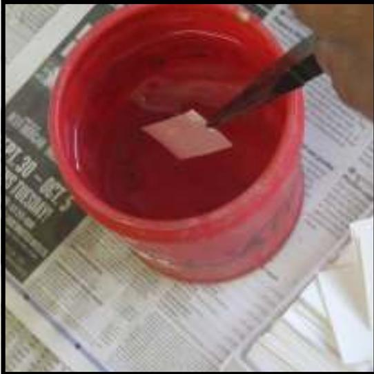
**Step 42:** With all the preparations made, insert the trimmed wafer into the container of water, holding the wafer with the tip of the needle nose pliers and waving it gently back and forth in the water. Keep an eye on your timer or watch, leaving the wafer in the water for approximately 30 seconds.
