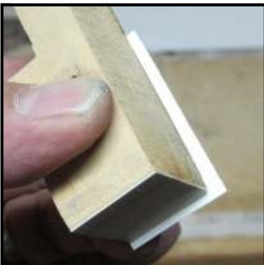
**Step 35:** Carefully turn the key over without disturbing the positioning of the gluing wafer. The excess on the front and side of the wafer needs to be trimmed away.
