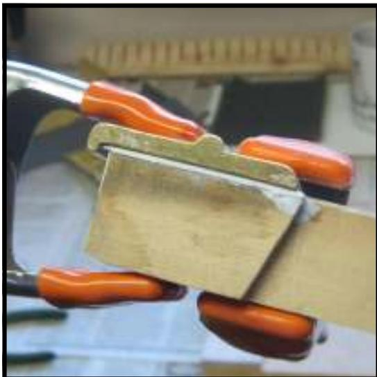
**Step 51:** Examine the ivory from the side to make sure that the back of the keytop has not lopped over the top of the front edge of the tail. Make sure also that the ivory has not slid slightly from side to side, leaving a portion of one side of the key uncovered, while the opposite side has an excess of ivory hanging over.
