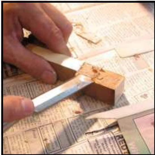
**Step 16:** Again try using a sharpened chisel. Instead of scraping the adhesive off, it is some times more effective to slice it off. Keep the flat side of the chisel flush with the top of the keystick, and swivel it back and forth across the surface to remove as much of the substance as possible. Again, be cautious not to remove wood from the keystick itself.
