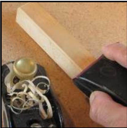
**Step 25:** Finish the procedure by using a small block plane (Cat. No. MF-33) to shave off the bulk of the excess, then by sanding the sides of the cap flush with the original keystick. (*Note: Refer to catalog for picture of actual plane.*)
