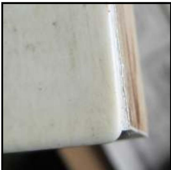
**Step 55:** This is what you hope not to see. An ivory has shifted position after the clamps were applied, leaving a portion of exposed. Don't be tempted to sand the side of the keystick flush with the ivory, as that will leave too wide of a gap between the keys. Better to bite the bullet, reheat and remove the ivory (and it will be harder this time) and start over.
