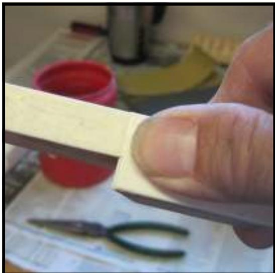
**Step 46:** Place the correct ivory keytop (make sure!!) on top of the wafer, pushing it up firmly against the seam.
