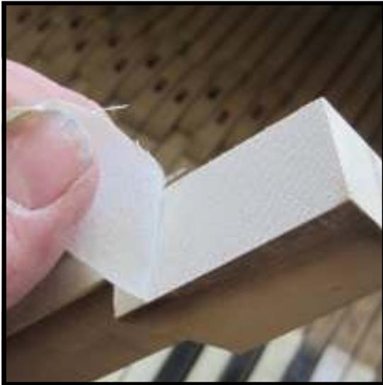
**Step 12:** Carefully peel the softened backing from the keystick, trying not to tear it as it is pulled away from the wood.
