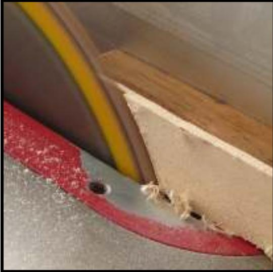
**Step 24:** Use your table saw to trim off excess thickness. (Before cutting, adjust the fence on the saw using the thickness of an adjacent note. Snug the fence up so that the key fits loosely between the saw blade [not turning, obviously] and the side of the fence.)
