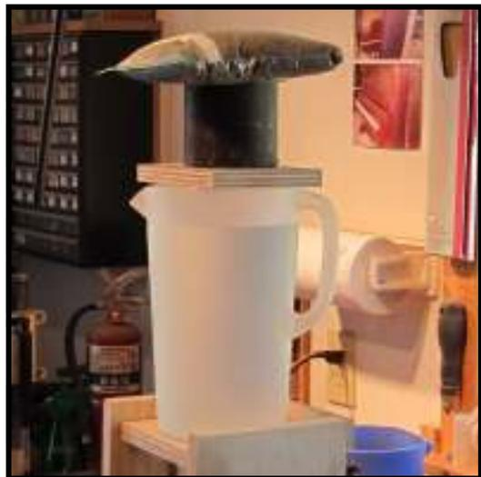
The upshot of all of this is that, unless I'm missing something here, using cement wafers in combination with brass plates works well if the plates are heated, but not well at all if the plates are cold, especially when used for shorter times. By heating the plates, good adhesion is achieved after as short of time as an hour. Thus, the procedure would be feasible in the field, if done before a tuning.
