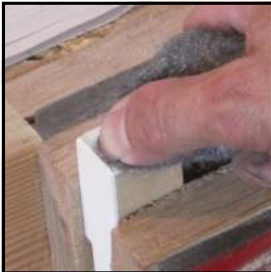
**Step 57:** Next, place the keytop in your vise to clean the front. Use 0000 steel wool if only a light cleaning is necessary. If heavy cleaning is needed, start with 400 grit paper, followed by steel wool.
