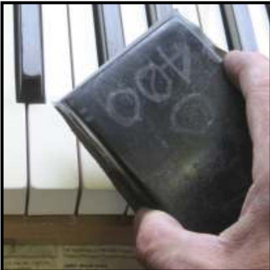
**Step 67:** Round the front edges of the keytops with a sheet of 400 grit paper on a sanding block. Use easy strokes, rotating the block slightly on each stroke. Work back and forth across the keyset until a even, gentle rounding is obtained. Follow this up with several swipes of 600 grit.
