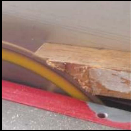
**Step 21:** For keysticks with a large amount of surface damage, it is sometimes advantageous to remove the top layer of wood altogether for replacement with a cap of basswood. To perform this procedure, first remove the ivory tail from the keystick. Use a table saw to cut off the damaged layer of wood. Cut off enough so that the resulting cap will be a solid piece of wood thick enough to work with and not just a thin layer of veneer.
