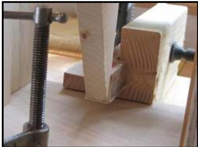
Using six old keys, I glued on ivories with ivory cement wafers using identical methods, except that for three of the ivories I used cold brass plates, and for the other three, heated plates. To avoid mix-ups in the process, I labeled the side of each key to label the process used and the starting and ending times.
