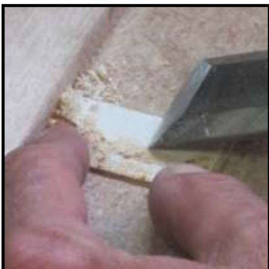
**Step 29:** Prepare each keytop as you go by scraping the underside of the ivory with a sharp chisel to remove old glue, linen or particles of wood.
