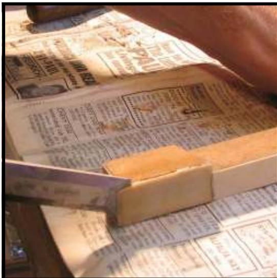
**Step 14:** Some adhesives will not loosen noticeably with the application of steam or heat. A sharp wood chisel will at times be more effective in prying the old ivory off than a putty knife. Swivel the sharp edge of the blade as you push towards the tail. Try rocking the chisel slightly to pry the ivory off.
