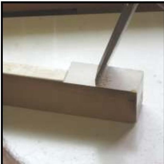
**Step 13:** Using a chisel, scrape off any remaining adhesive. *You do not need to be completely down to bare wood, but the wood should be showing through.*
