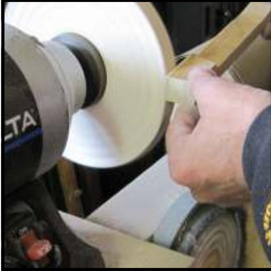
**Step 69:** Using a light touch, run the keytop at a moderate pace back and forth across the surface of the wheel. Two or three passes usually is enough.
