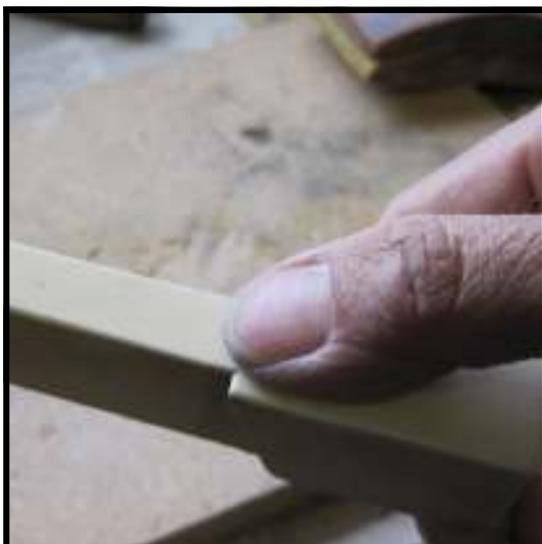
**Step 58:** Check the joint between the head and the tail for unevenness in height. A discernible difference in thickness will mean that either the head or the tail will need to be sanded down flush.
