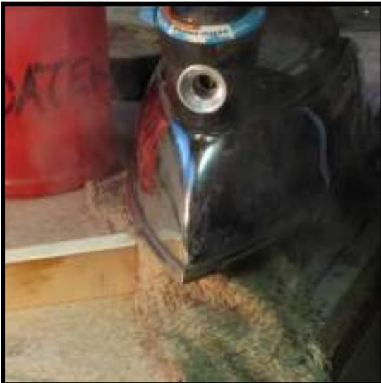
**Step 6:** If removal of old keytops is necessary, place a damp, absorbent cloth over the top of the ivory to be removed, and heat with an iron on a medium setting for about 30 seconds, or until the cloth quits steaming.
