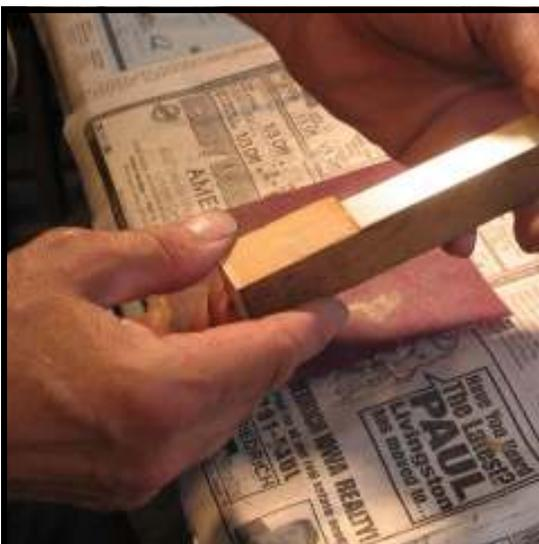
**Step 20:** Once the filler is dry, repeat sanding as in step 17, then reexamine the surface. If an indentation is still noticeable, apply a second application of wood filler and resand.
