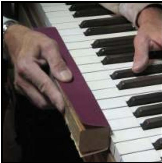
**Step 65:** Use a 11" piece of 2" x 2" lumber as a sanding block to even out the front edges of the keytops. Work back and forth across the keyset, checking your progress frequently to avoid taking off more ivory than absolutely necessary. Once the stand-outs are even with the surrounding keytops, quit.
