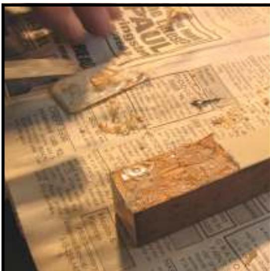
*Note: With the ivory keytop finally off, it is obvious that the keystick pictured would need more attention than normal to bring it up to the desired condition. The adhesive remaining in this situation proved to be very difficult to remove. Additionally, a chunk of wood from the top of the keystick adhered to the underside of the ivory.*
