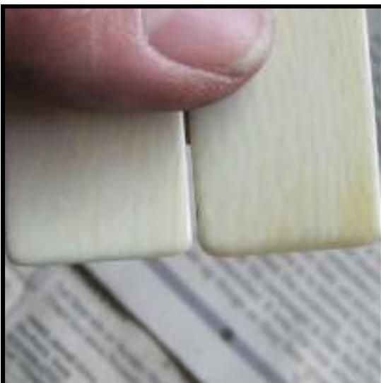
**Step 2c:** Finally, the amount of wear on the leading edge of the key can be a clue as to its proper location. An A key from the center of the keyboard, for example, will likely have more wear evident than an A key which comes from the either the bass or the treble end. The key on the right, which was an A4, has considerably more wear than the one on the left, which was an A1. *Notice the more translucent front edge.*
