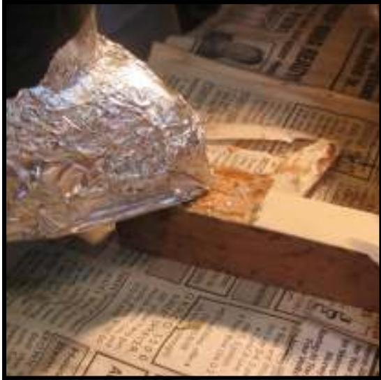
**Step 15:** For adhesive of such tenacious nature, try a direct application of heat to soften the substance, but don't be surprised if this is ineffective. (Be sure to cover your iron with foil to avoid a transference of the adhesive from the keystick to the surface of the iron.)
