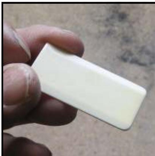
*Finally, keytops often have important dimensional differences with noticeable variations in length, width and thickness. Edging treatments may also differ. In searching for ivories to fill in missing spots, look for keytops that are at least as long, as wide, and as thick as the originals. Excess ivory may be removed by sanding, but a keytop that is too short, too narrow, or too thin will draw the eye as an obvious substitution.*
