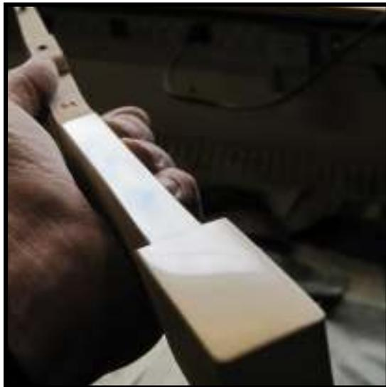
**Step 70:** Hold the key up to see the reflection from a window or overhead light. The surface should appear glass-like in appearance without visible scratches. If small defects are noticed, go back to sanding out the surface with 800, then 1000 grit of paper. Rebuff on the wheel and check in the light again.
