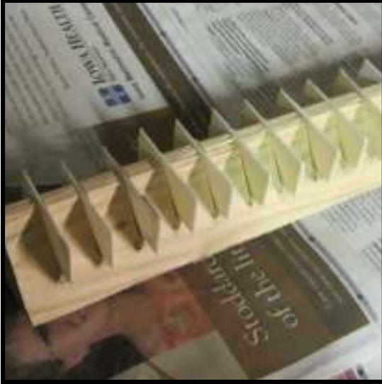
**Step 8:** If you are regluing the entire set of ivory fronts, use a holder to keep the keytops in order from A0 to C8. The homemade holder pictured is simple to make, consisting simply of a 2" x 2" cut on a diagonal with slots every 3/4". The slots may be then labeled starting with A0 and ending with C8.
