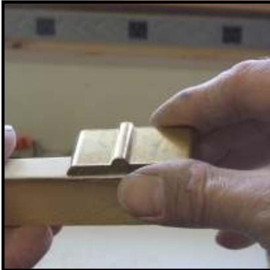
**Step 48:** Quickly place the heated head plate over the ivory, with the lip of the plate butted up against the front edge of the keytop. Make sure that the ivory is still aligned from side to side, with no portion of the ivory hanging over on either side.
