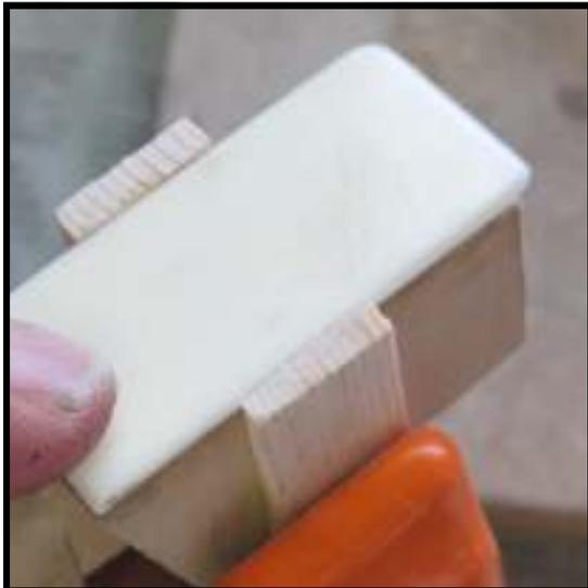
**II.** Have the restraints clamped in place before placing on the wafer and the ivory. With the overhanging lip of the restraints held in place at the bottom of the key, the top of the restraints should be cut so that the top edge sits just below the top surface of the ivory.
