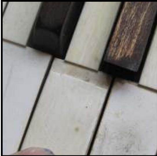
**Step 3:** Once the correct location for a keytop has been determined, place that top on the correct key for the time being so that you can turn your attention to filling in the rest of the gaps.
