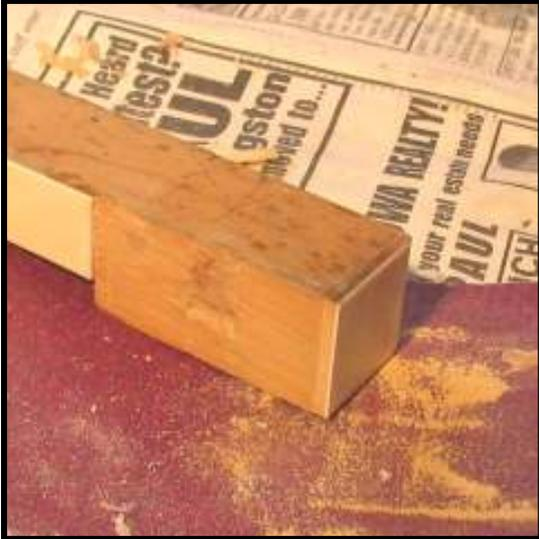
**Step 18:** At this point, ascertain the condition of the keystick. A bit of roughness is tolerable, but a missing chunk of wood such as is visible in the photo (notice the key is turned side-ways), needs to be filled.
