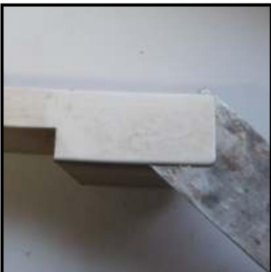
**Step 7:** Carefully remove the ivory by prying up with a narrow putty knife. Start from the front of the key by gently pushing the overhang up, then work the blade of the putty knife between the ivory and the fabric backing cloth or the wood of the key. By working the putty knife back and forth and pushing it towards the tail, most keys will come loose. If the keytop refuses to come completely loose, try reheating with the damp rag and iron, then repeat the process.
