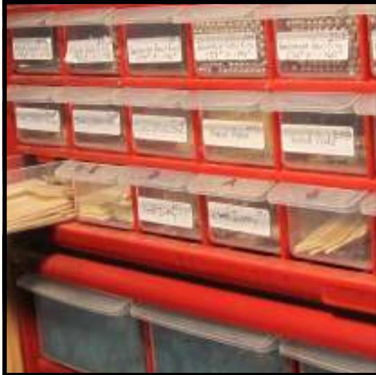
*Hint: In order to replace ivory keytops, it is helpful to have your collection of used ivories cleaned and sorted by note. C's and F's, though not identical, are close enough to be stored together. The same goes for B's and E's. D's, A's and G's all are distinct. For replacing a C8, you will need an ivory with no filing marks. Obviously, the larger your collection of ivory, the better your chances at finding good matches that will blend in.*
