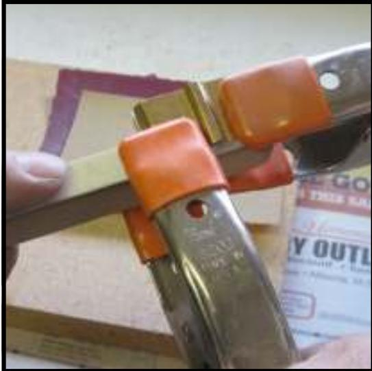
**Step 50:** Apply a second clamp as shown, this time tilting it slightly from side to side so that the bottom jaw is again further back than the top jaw.
