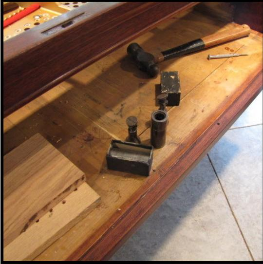
**Step 6:** Before installing new tuning pin bushings in the plate, the pin block should be supported from underneath. [Pinblock support jacks \(Cat. No. 800\)](#) or a [pin block support \(Cat. No. 799\)](#) are both proper tools for the job.
