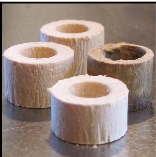
**Step 8:** Select the correct size of tuning pin bushing. Compare the lengths of available new bushings to the length of a sample old bushing. [Tuning pin bushings \(Cat. No. 346A, B and C\)](#) are 7/16" in diameter and are the common size for most older and some newer pianos. A smaller 13/32" size of [tuning pin bushings \(Cat. No. 345A, B and C\)](#) are available for newer pianos that have been drilled with a slightly smaller hole.
