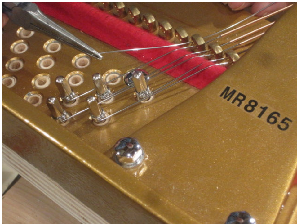
Photo 113: Each bass string is first attached to its own hitchpin at the back of the piano, then pulled through the hole in the agraffe meant for it. These agraffes have 2 holes each instead of 3 as in the treble section. Further down still, the agraffes for the lowest notes will have a single hole each.
