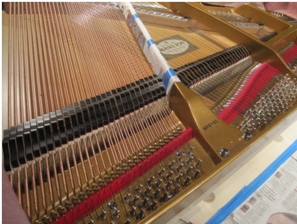
Photo 124: All dampers reinstalled.
