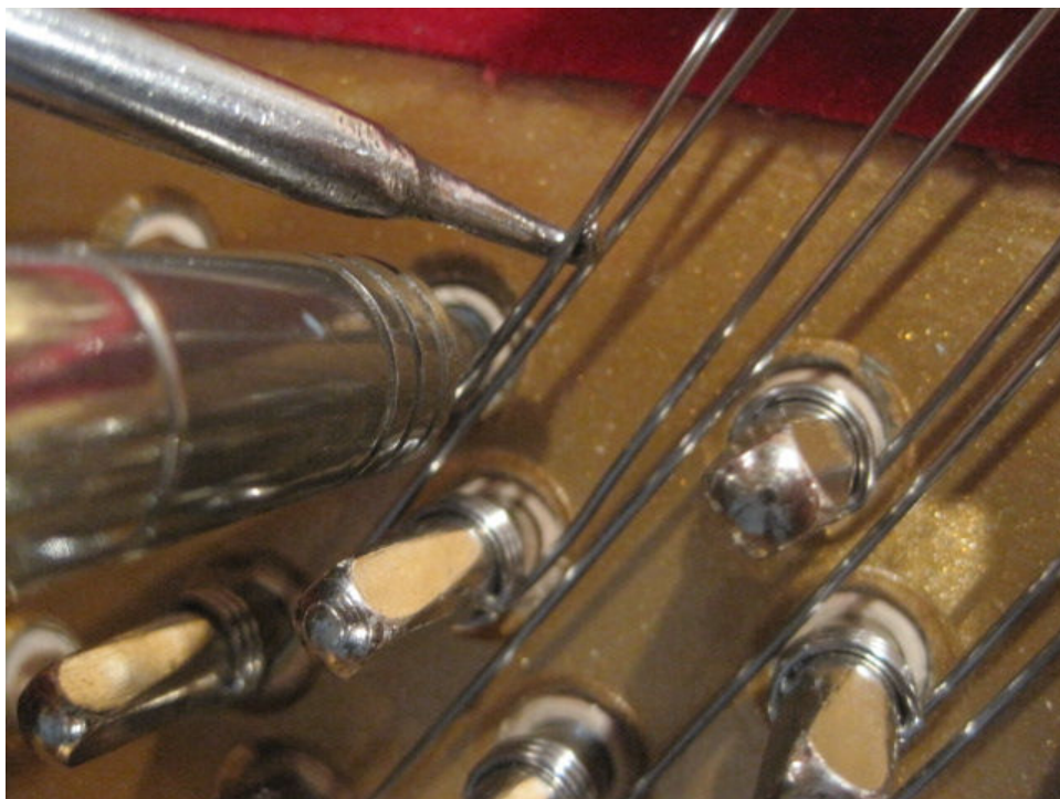
Photo 118: The string is pulled up with a string hook while tension is put on with the tuning hammer.
