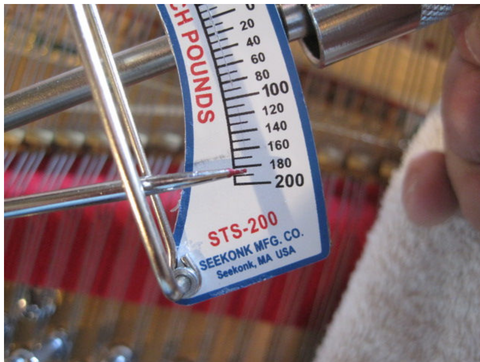
Photo 112: I check the initial torque on the pins in the bass. Readings have been consistently in the 180 – 200 inch pound range, where you want it with new pins.
