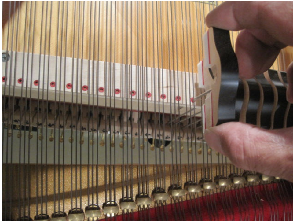
Photo 123: Damper wires are connected to the back action in the cavity where the action of the piano goes. Careful adjustment from side-to-side, and up-and-down is necessary for each damper.
