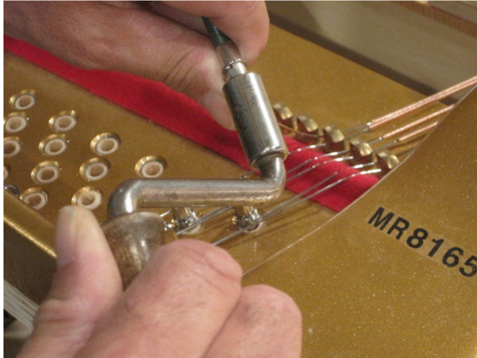
Photo 115: Using a string crank, the coil is formed on the end of the string.
