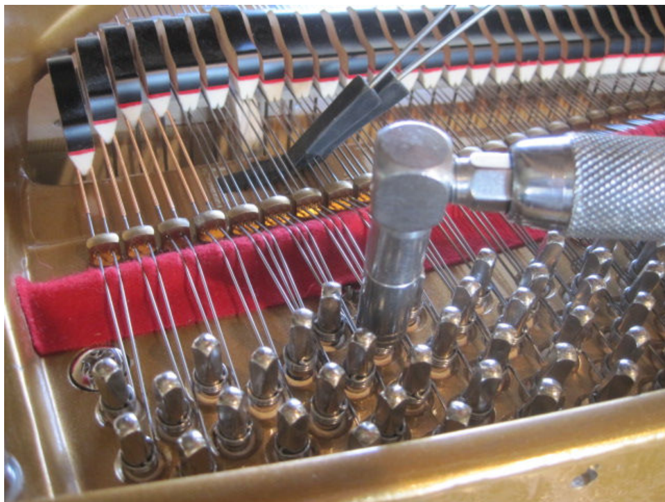
Photo 125: The initial tuning is begun. New piano string stretches, so the first several tuning will not be particularly stable.
