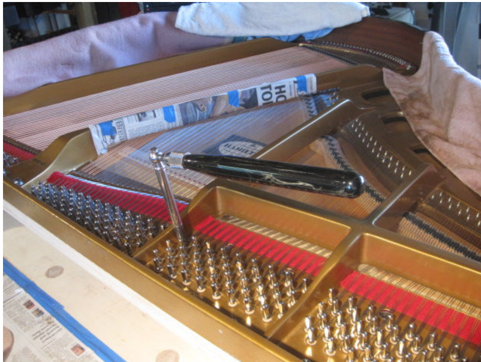
Photo 120: The piano is chipped up to approximate pitch.
