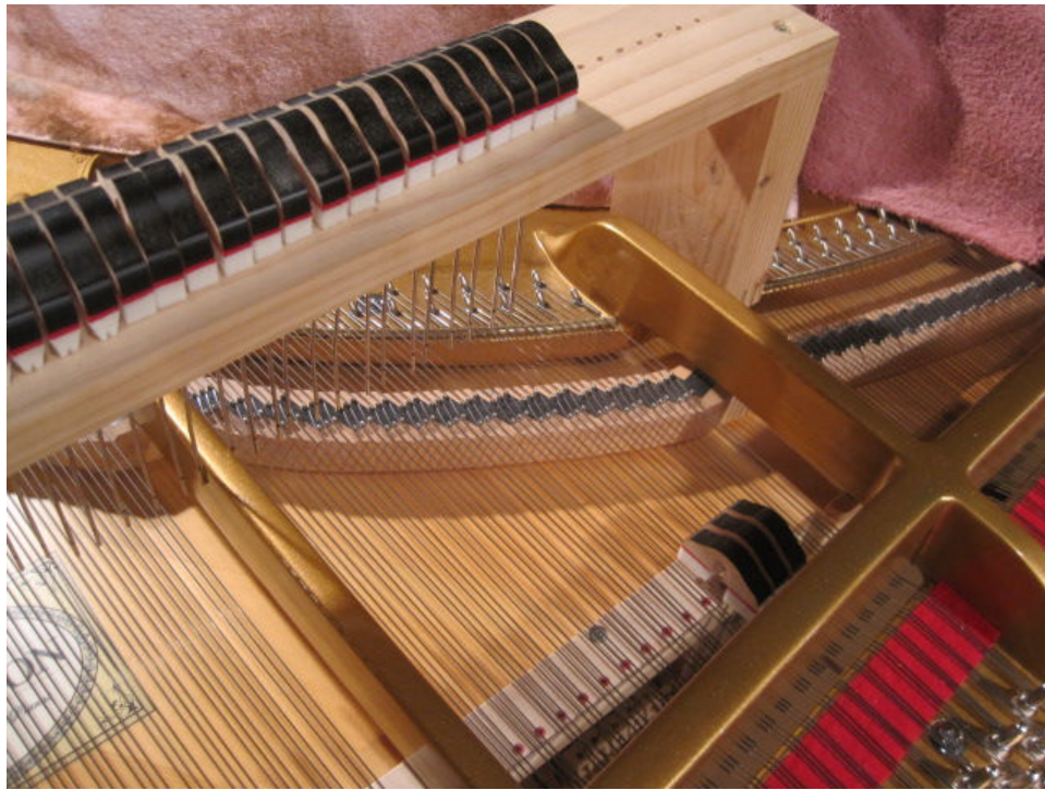
Photo 121: With the tension on the strings, the dampers are now brought out of storage for installation.
