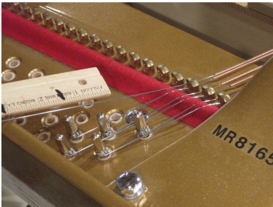
Photo 114: The end of the ruler is held exactly above the center of the pin hole. The leader on the string is cut at 3 1/8" .
