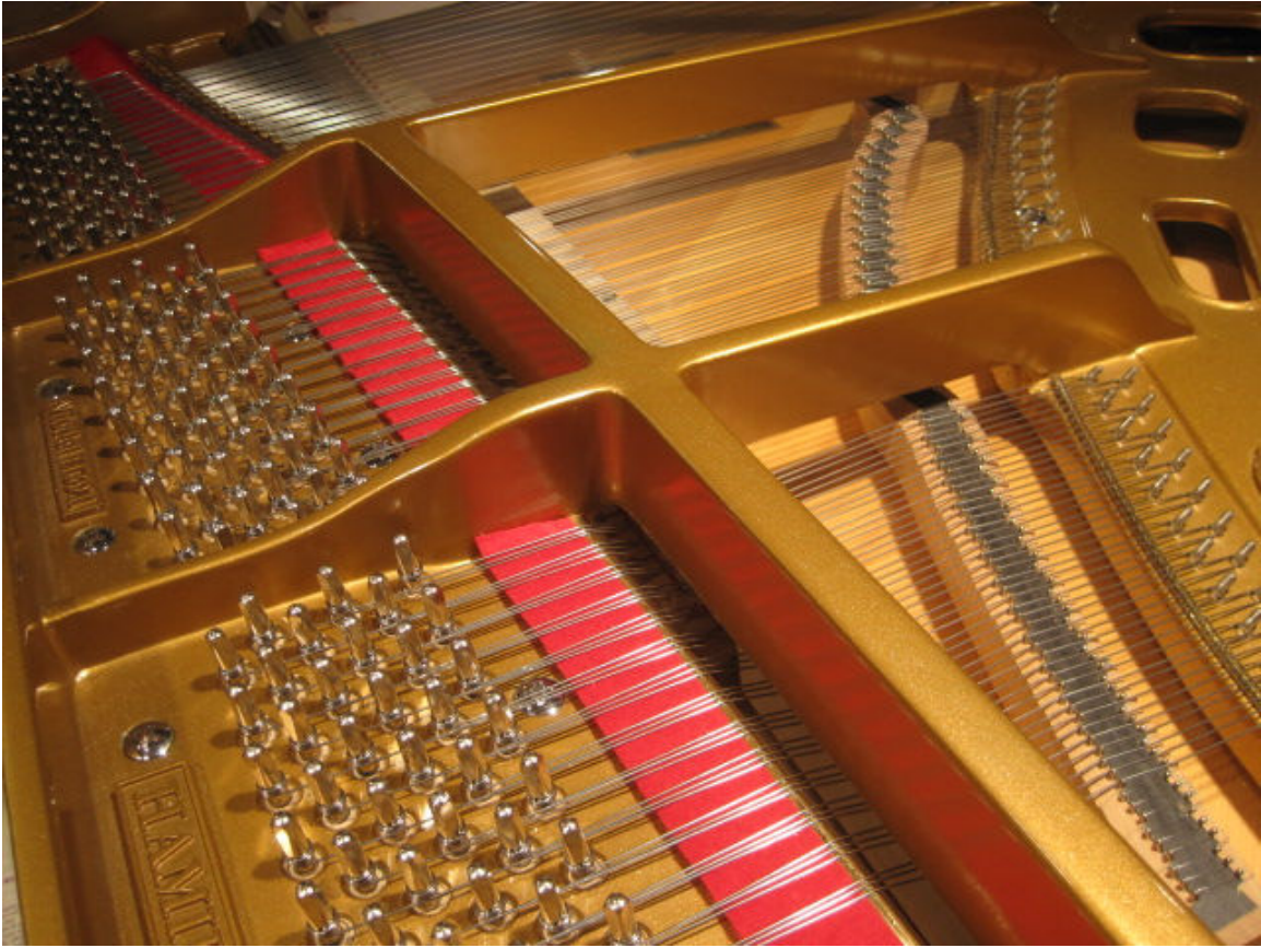
Photo 108: The finished treble stringing.
