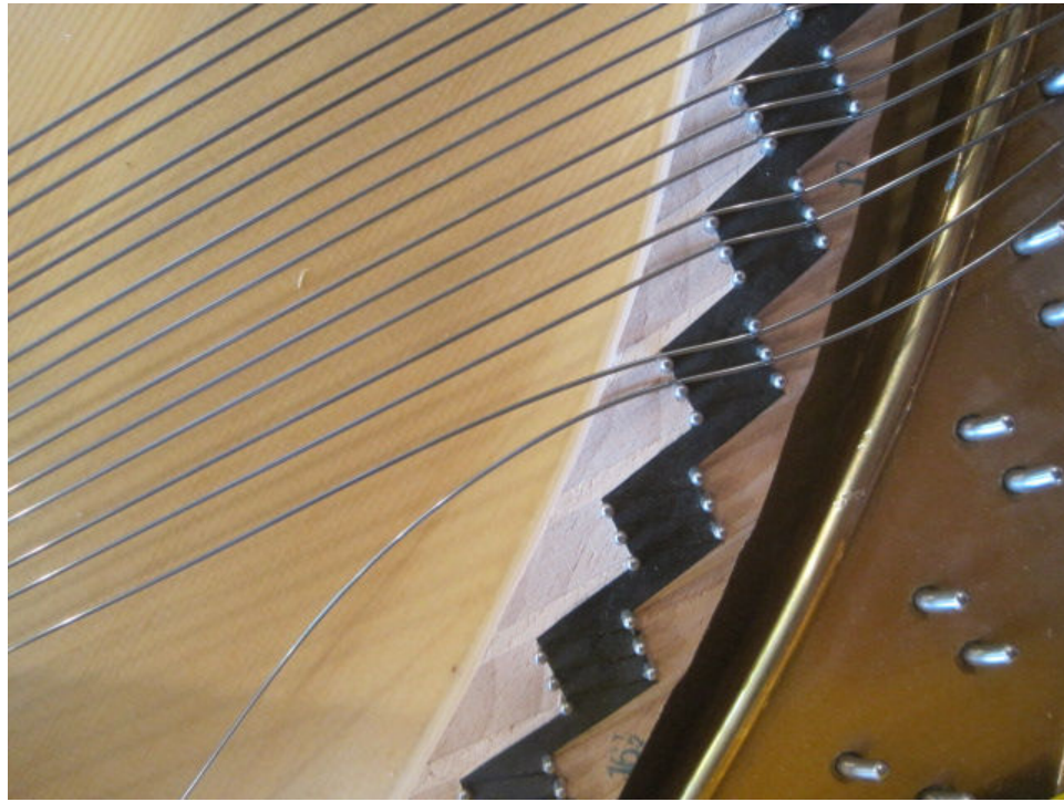
Photo 100: . . .then threaded past the bridge pins.
