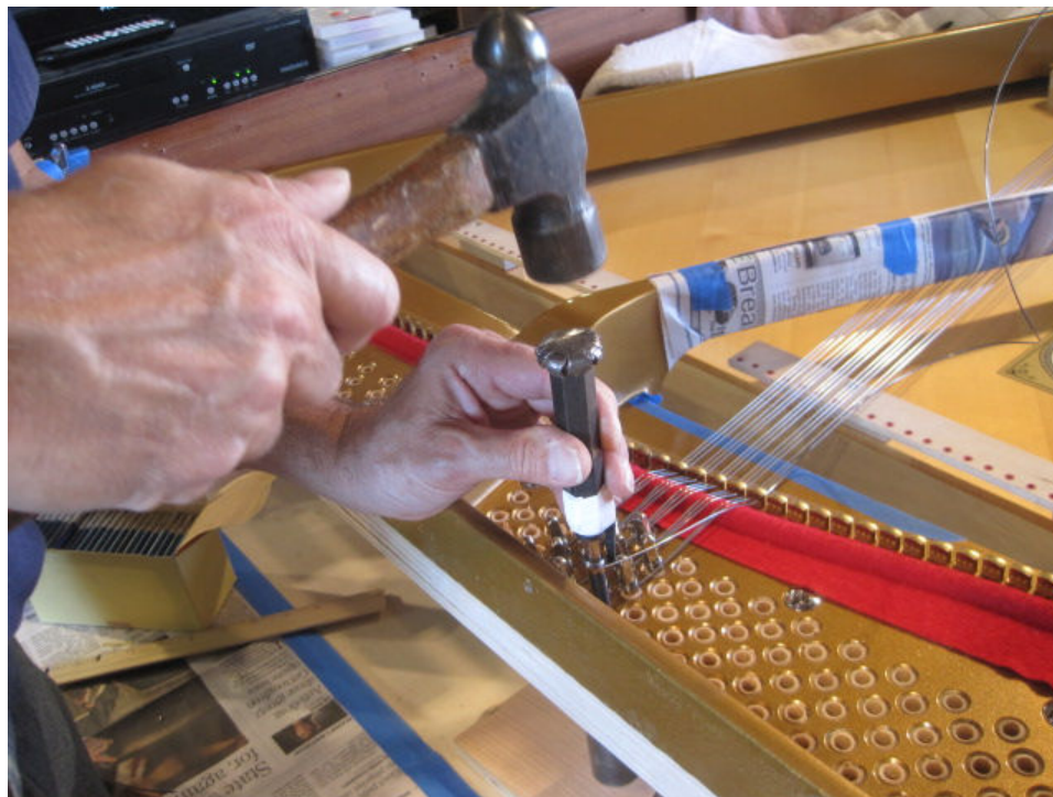
Photo 97: Using a pin punch and a ball peen hammer, the pin is driven into the pin block to a exact depth.
