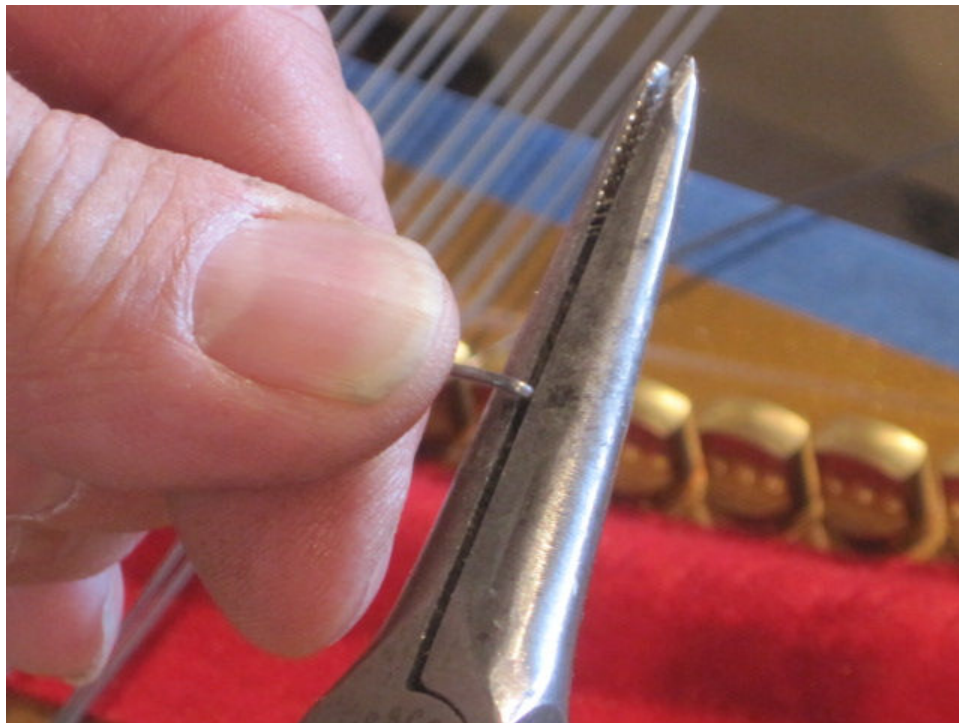
Photo 95: The bend, (referred to as the 'beckett') is formed using a pair of needle-nose pliers.
