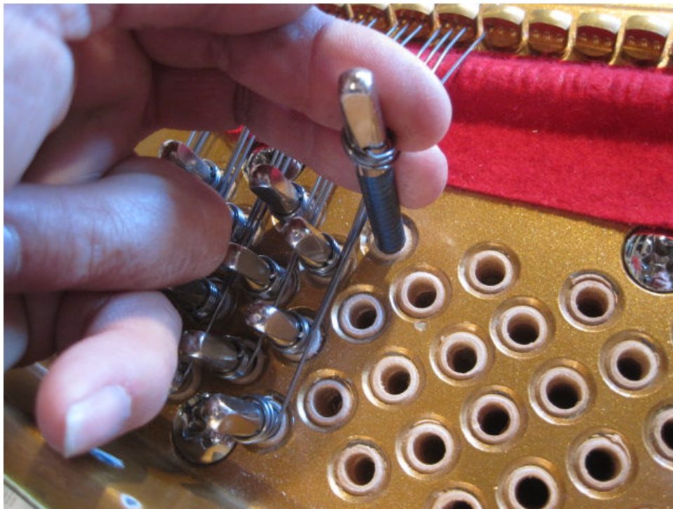
Photo 104: A second beckett and coil are made, and the pin is lined up with the hole.
