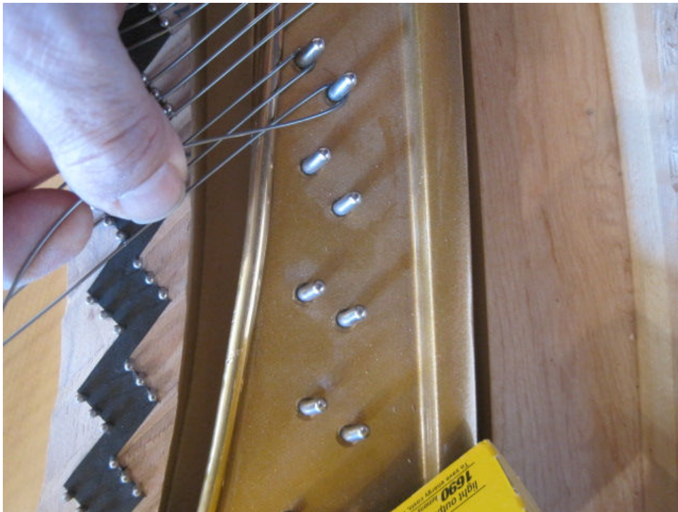
Photo 99: The wire is pulled around the plate pin. . .
