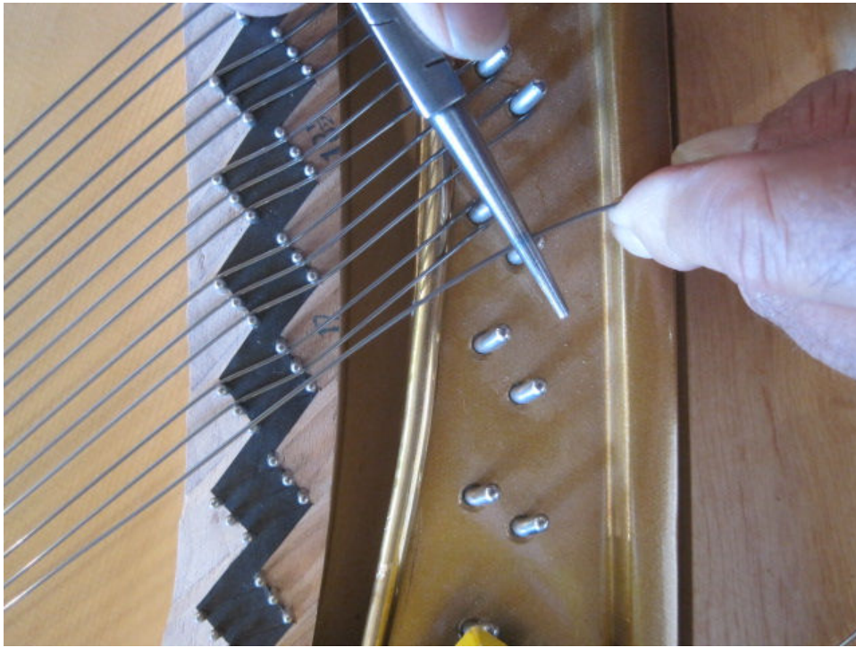
Photo 98: Each treble string goes from a tuning pin, around a plate pin at the back of the piano, then returns to the front of the piano to be attached on the other end to another tuning pin. Here, the bend is put in the wire at the plate pin, using a pair of round nose pliers.
