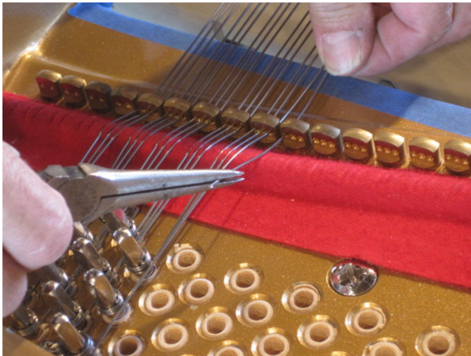
Photo 102: The cut end is brought underneath a strut in the cast iron plate, then threaded through the agraffe on the other end. Notice that the beginning of this wire went through the far right hand hole in one agraffe, and returns through the far left hand hole in the next, meaning that the wire is divided between two separate notes.
