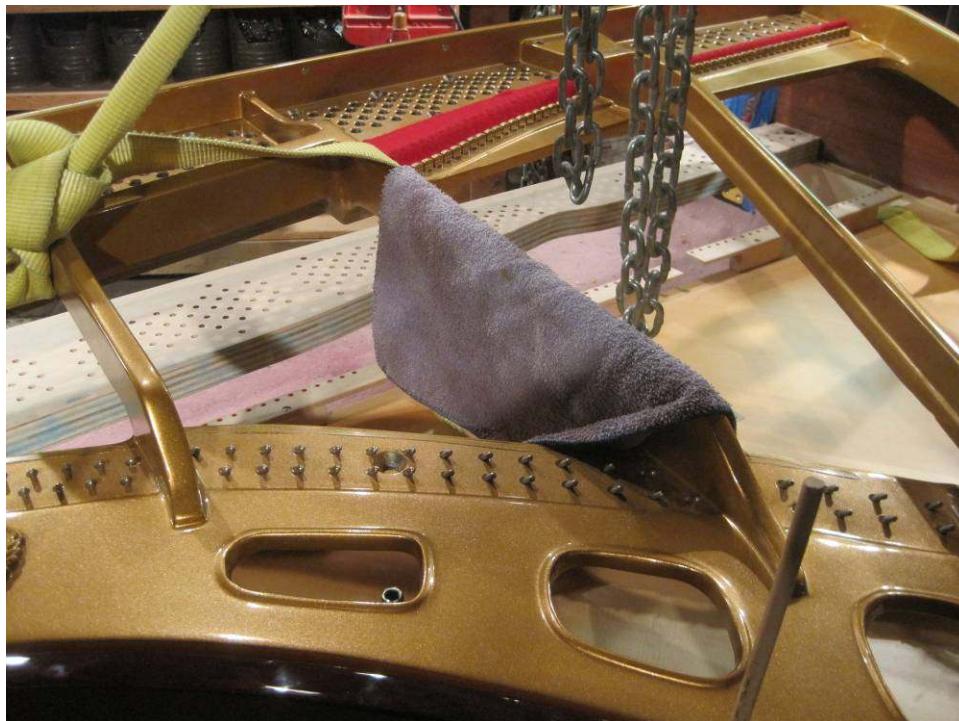
Photo 85: With the pinblock in the piano this time, the plate is carefully lowered down one last time. If everything was done correctly, all screw holes and pin holes should line up exactly.
