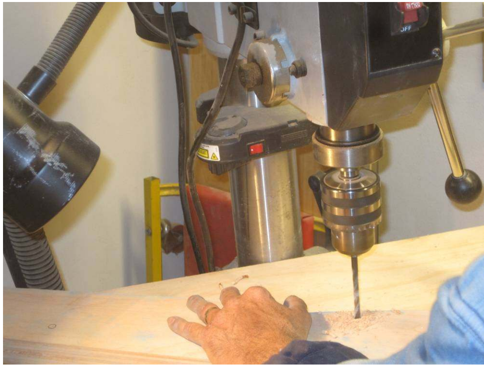
Photo 66: Several of the screw holes are drilled, so that the pinblock may be positioned securely to the plate before the pinblock holes are drilled.
