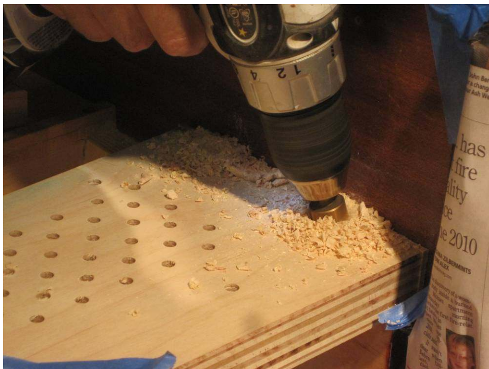
Photo 82: The screw holes are countersunk.
