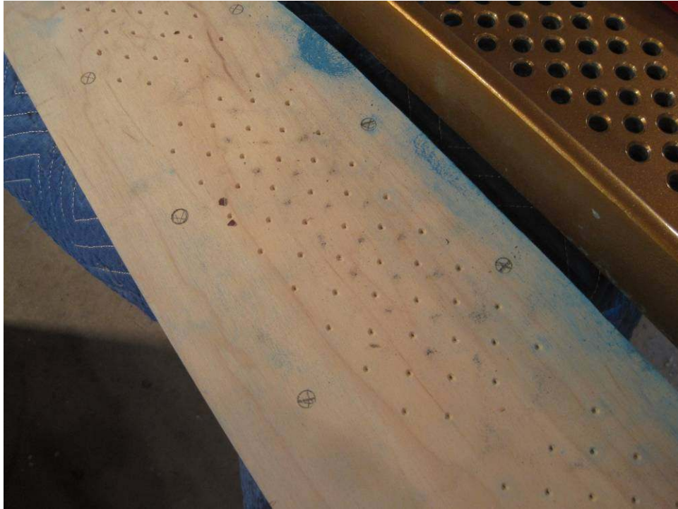
Photo 74: Once the tuning pin holes, and the rest of the plate screw holes are marked, the pinblock is removed from the plate for drilling.
