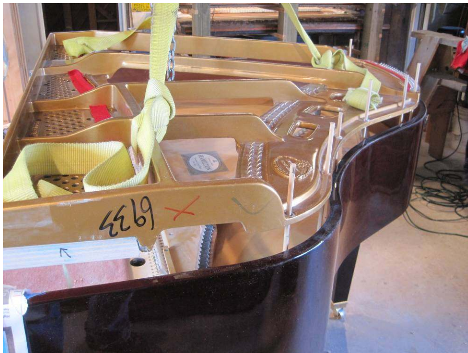
Photo 79: The plate with attached pinblock is carefully lowered for the first of several times into the piano. The dowels line up the screw holes in the plate with the hole along the outer edge of the soundboard. The helps the plate smoothly lower into position without making unwanted contact with the inner rim.
