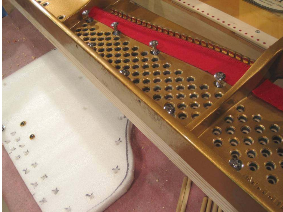
Photo 86: Screws are taken from the foam board where they have been stored, and put back into the correct holes and turned down.
