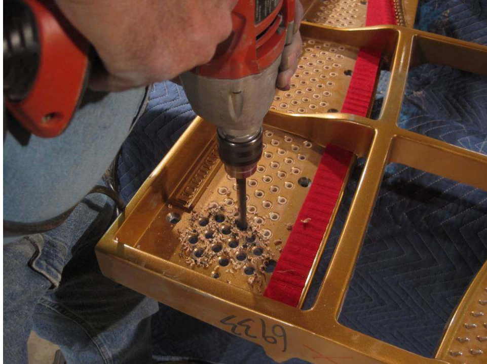
Photo 67: The plate is now turned right side up. Before marking the tuning pin holes, however, the original tuning pin bushings must be removed. Ordinarily, these are punched out, but for some reason the factory glued these bushings in place, so they must be drilled out.
