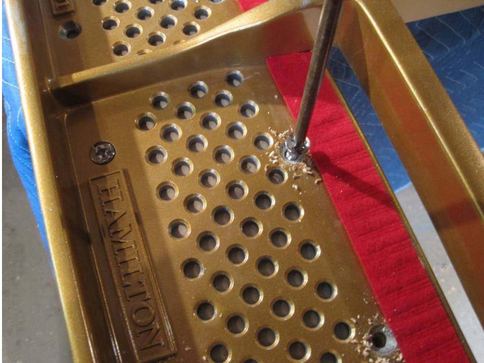
Photo 70: Screws on either end of the plate and in the center are tightly screwed down.
