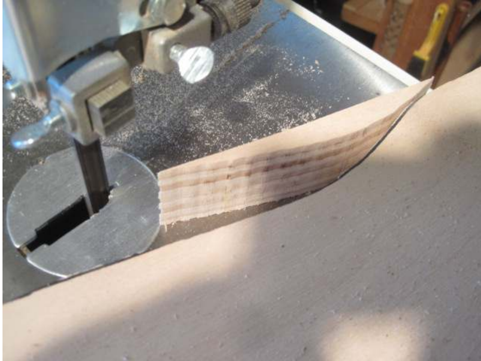
Photo 52: With the narrow blade, the cut is easily finished.
