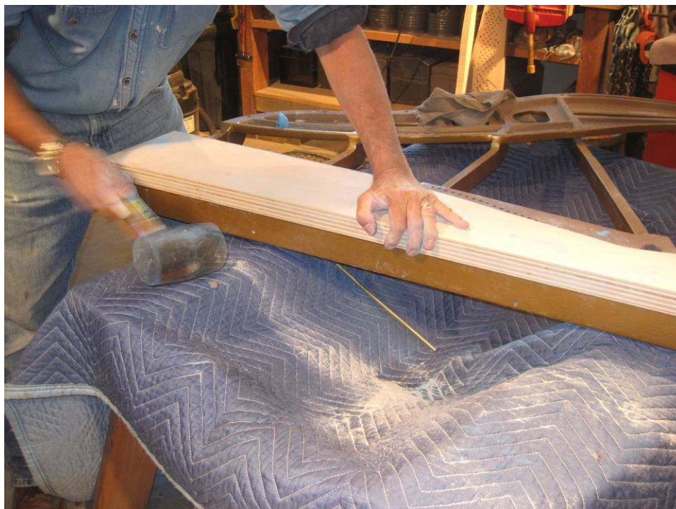
Photo 57: Placing the pinblock back on the plate, I knock it in several places with a heavy rubber mallet. This will show me the high spots, where wood is touching metal.
