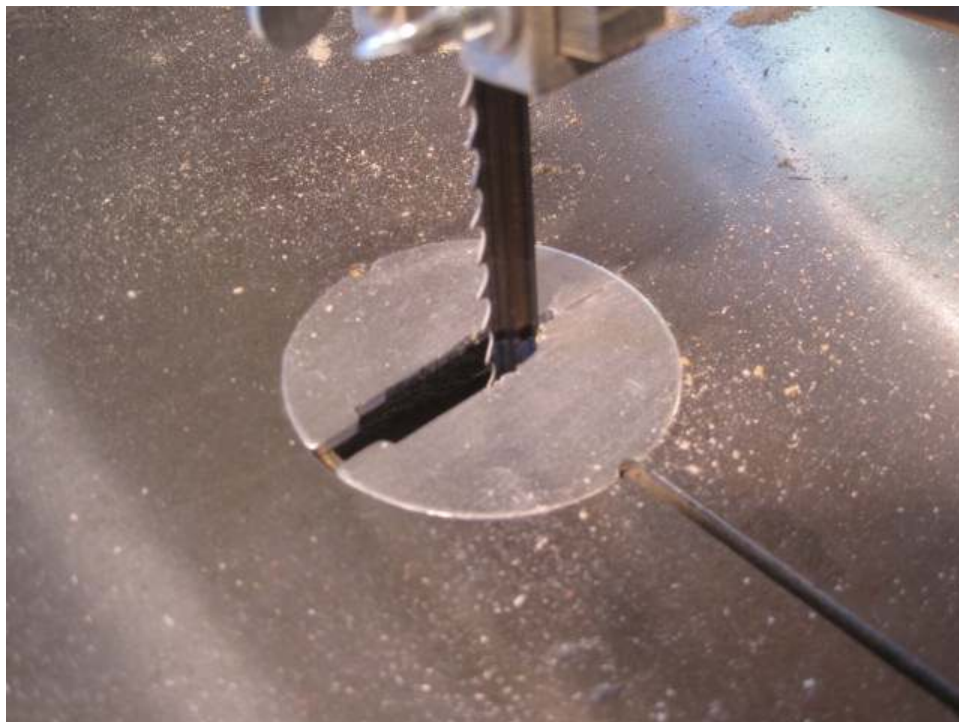
Photo 51: A \frac{1}{4} " blade is substituted. The wider blade gives a steadier cut on the overall line, and so it's worth the time to make the switch to get the best of both blades.
