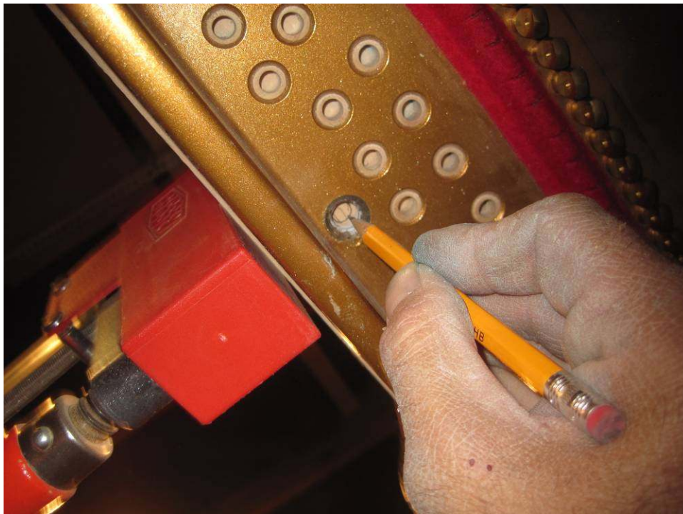
Photo 65: Looking up from underneath, I mark the screw holes, but not the tuning pin holes.
