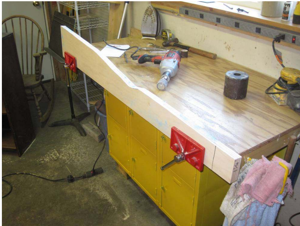
Photo 59: I next carry the pinblock to another room of the shop (not enough free space here for the cast iron plate, unfortunately), where a special bench with a pair of vise is used to steady the work piece.
