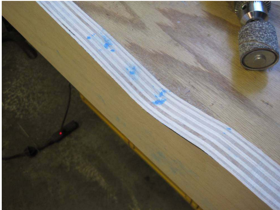
Photo 61: After a dozen or so trips back and forth, progress is being made. The idea is to have continuous chalk spots showing up from one end of the pinblock to the other.
