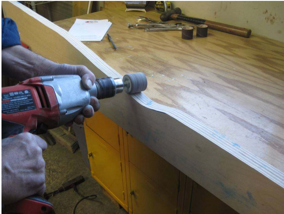
Photo 60: Using a grinding drum mounted on a heavy-duty drill, the chalked spots are ground down. The process, once begun, repeats itself over and over.
