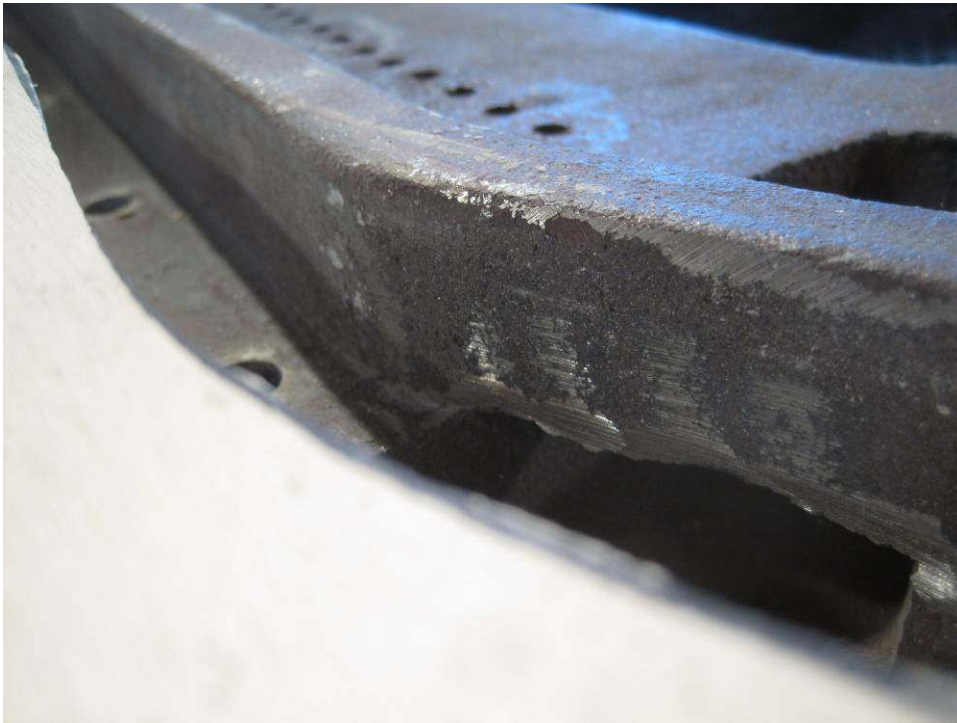
Photo 54: The pinblock should butt up firmly against the corresponding flange on the underside of the plate. With a good fitting job, the wood / cast iron connection will be snug from one end of the pinblock to the other. An absolutely tight fit will dramatically affect the stability of the tuning, as the strings, when brought up to tension, exert approximately 20 tons of tension pulling the pins, and the pinblock, backwards towards the rear of the piano.
