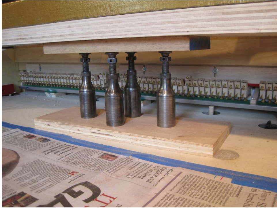
Photo 90: The underside of the pinblock is supported where the first pins will be installed in the tenor section of the piano.
