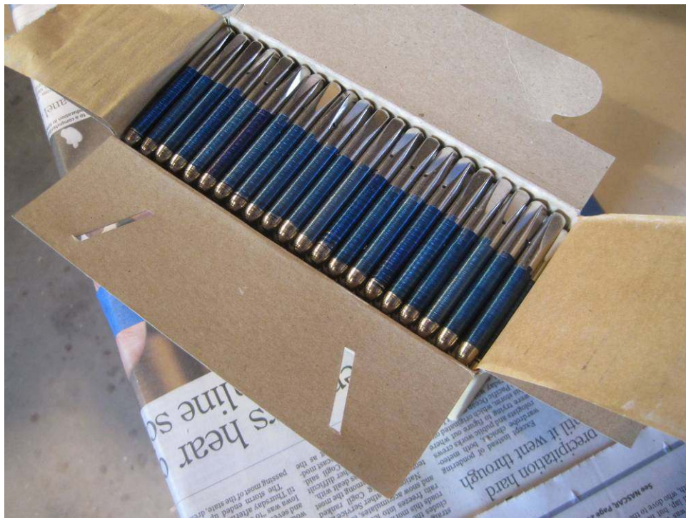
Photo 91: Size 2/0 (factory size) of nickel plated, blued pins.
