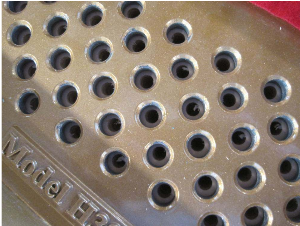
Photo 78: With the pinblock again temporarily screwed to the plate, the pin holes line up perfectly. The appearance of off-center screws is an illusion caused by the position of the camera relative to each hole.
