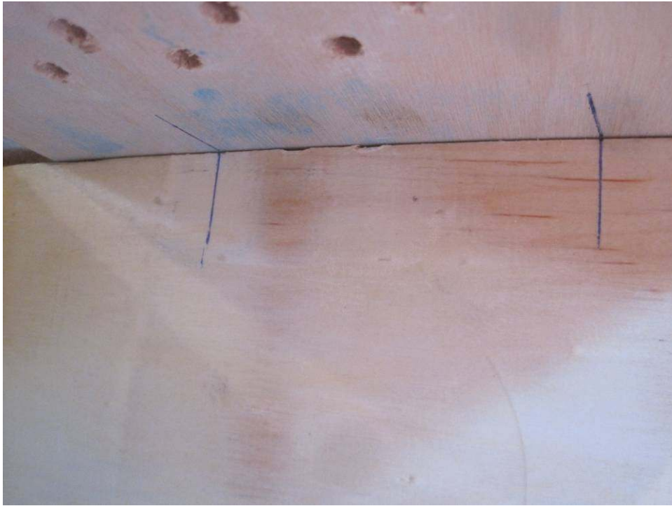
Photo 80: Once the exact positioning of the pinblock and plate are determined, matching lines are drawn where the underside of the pinblock rests on the ledges inside of the rim.
