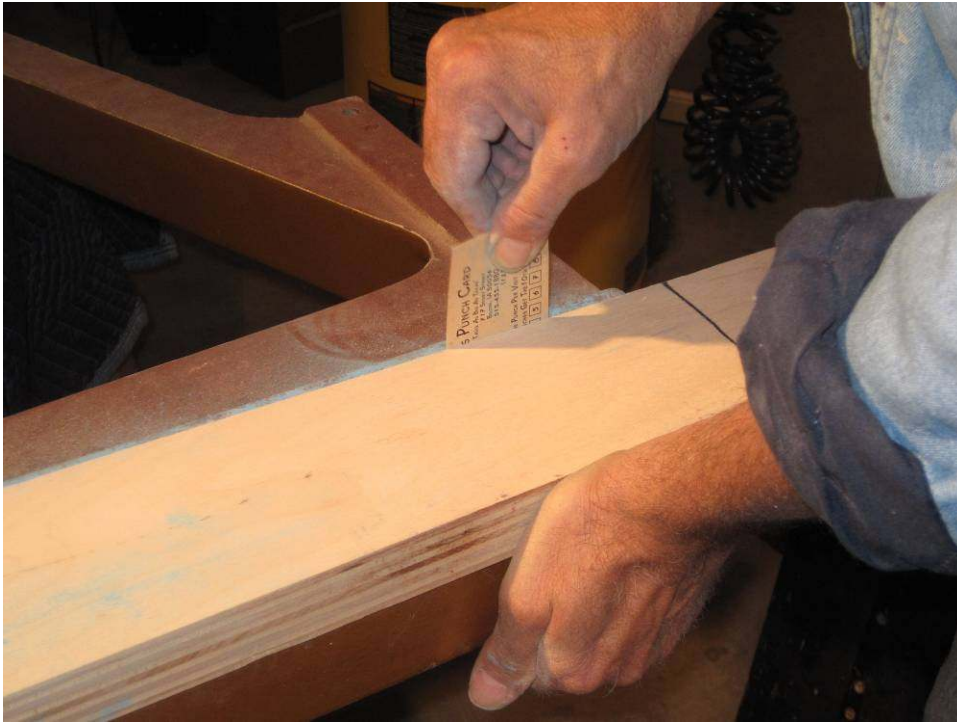
Photo 62: After 78 trips back and forth (anywhere between 50 and 100 is typical), the pinblock passes the “business card” test. A business card, placed anywhere along the pinblock between the wood and the metal flange, will be grabbed tightly when the pinblock is pressed forward.
