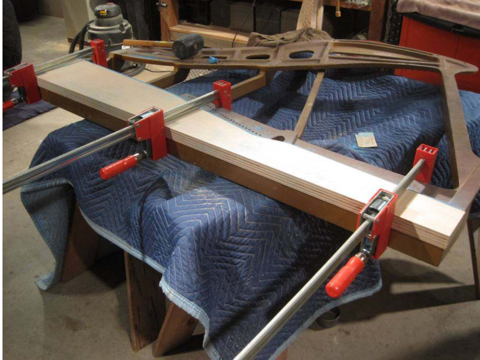
Photo 64: Before flipping the plate, the pinblock is clamped into place for the purpose of marking the holes for the plate screws.
