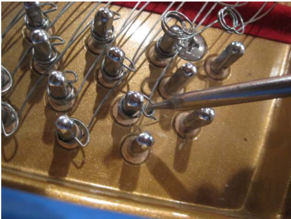
Photo 18: Coils are pulled loose from pins with a string hook.
