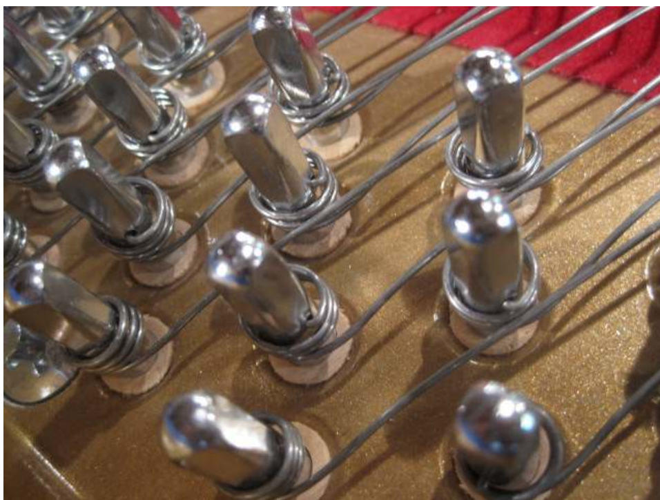
Photo 16: Tension Coils are loose with tension released.
