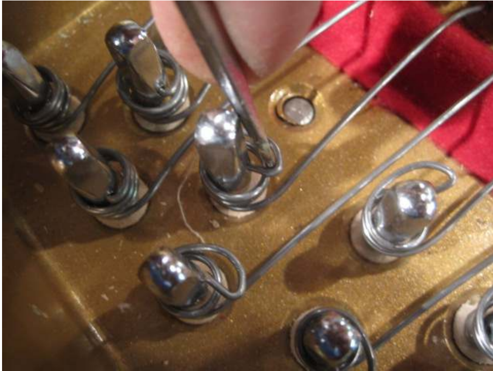
Photo 17: Beckett in each string is pulled from its pin.
