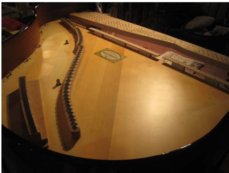
Photo 30: Soundboard and bridges seen from back end of piano. Pinblock is screwed down to ledges inside the rim.
