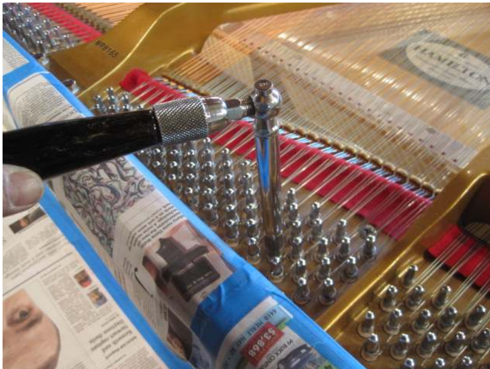
Photo 15: Tension on strings needs to be reduced from approximately 18 tons to zero before strings may be safely removed.
