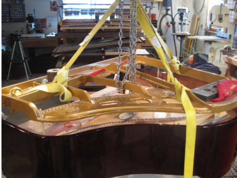
Photo 28: Plate is lifted with hoist. Hoist is rated for 2000 lbs. Plate weighs approximately 300 lbs.
