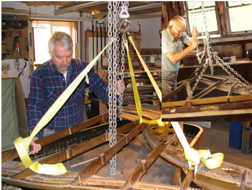
Photo 1: Now and then – The author removes plate from a Weber grand (circa 1880). Inset – Paul Behm trying out new hoist in 1976.
