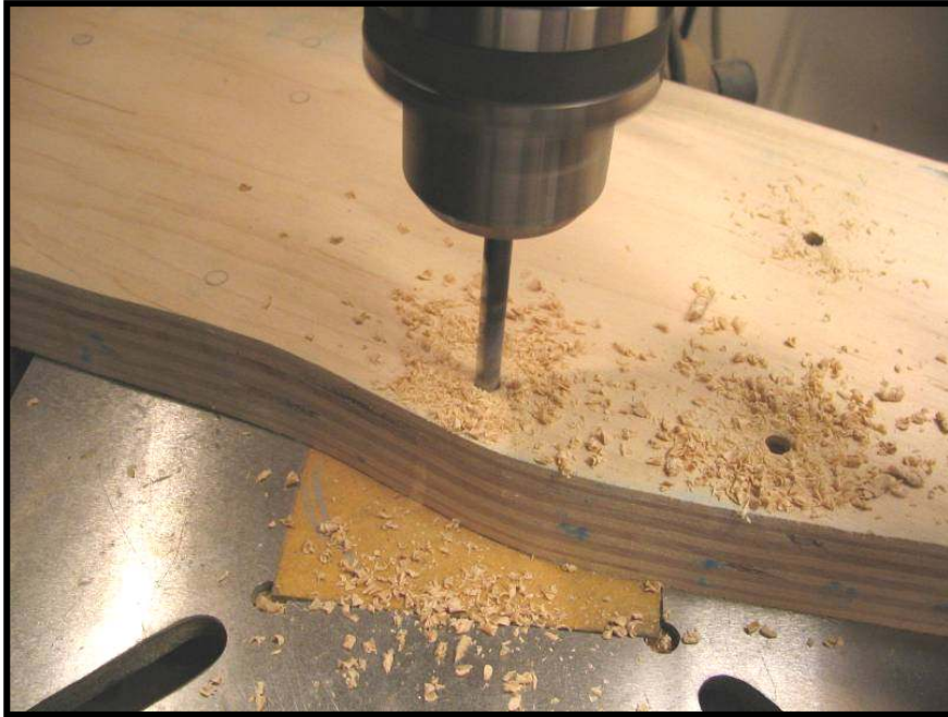
Photo #3: Drilling the pilot holes for the plate screws.
