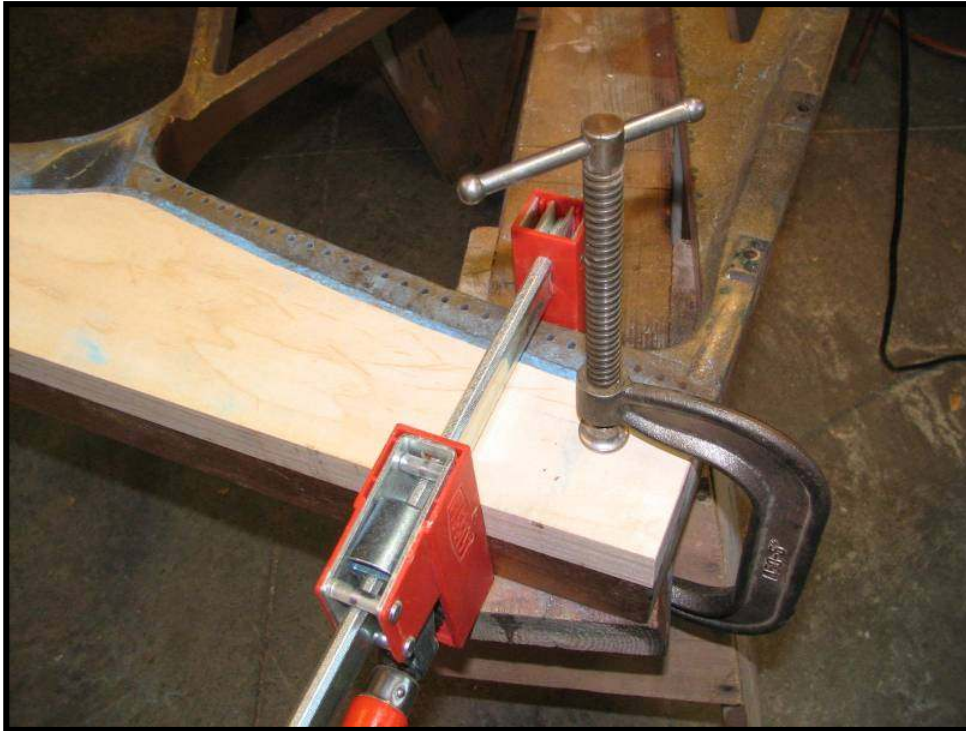
Photo #1: Pinblock clamped firmly in place.
