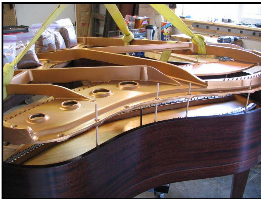
Photo #11: Guide dowels help lower the plate safely
