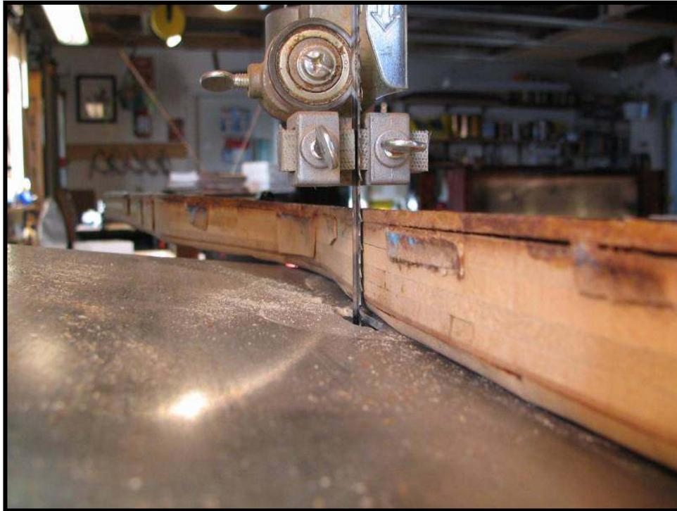
*Photo #2: Matching the blade to the bevel*
