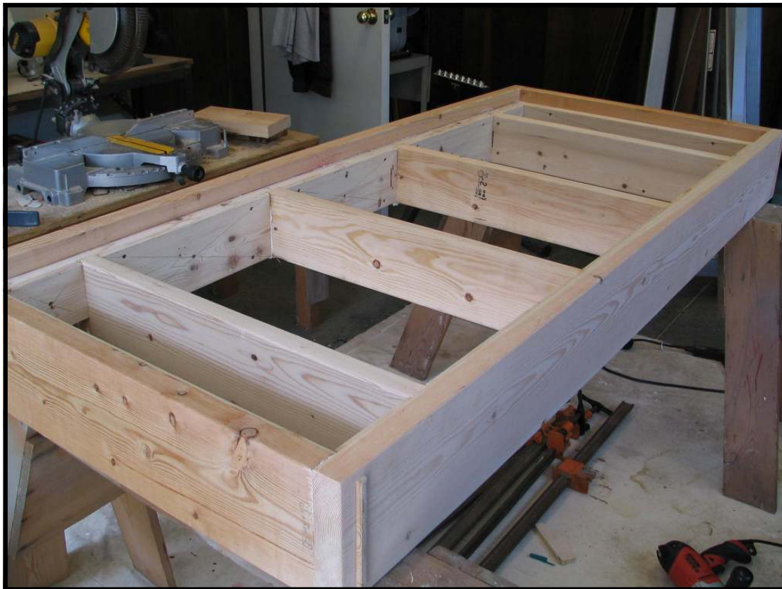
Completed framework assembly with mortise and tenon joints.
