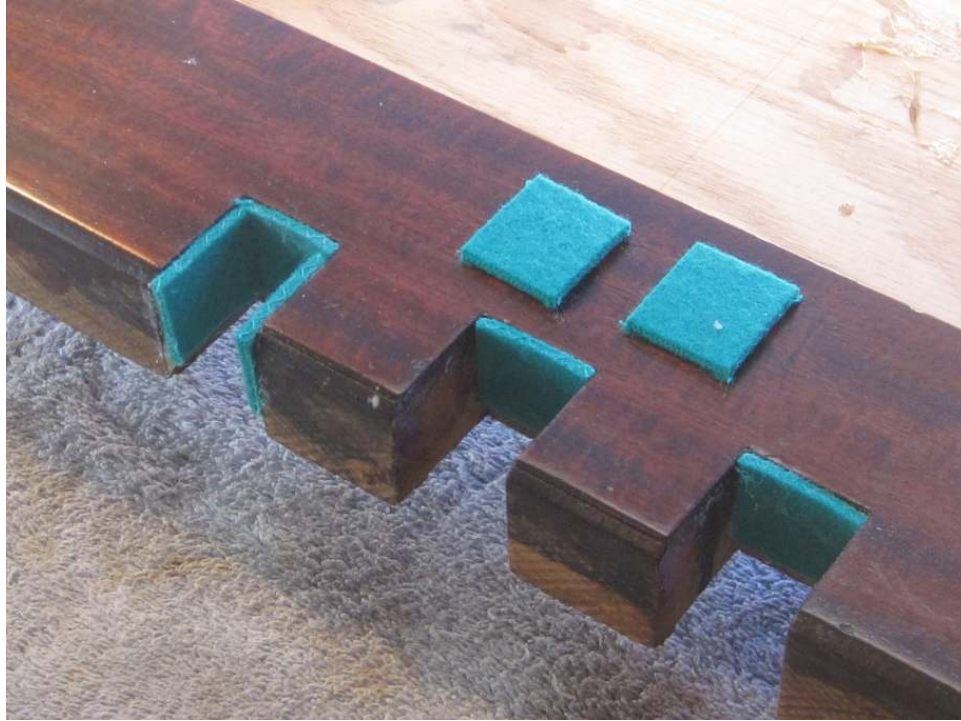
Photo 46: The felts are glued in place with Titebond. The top square goes in first, with the side felts put in to support the top.
