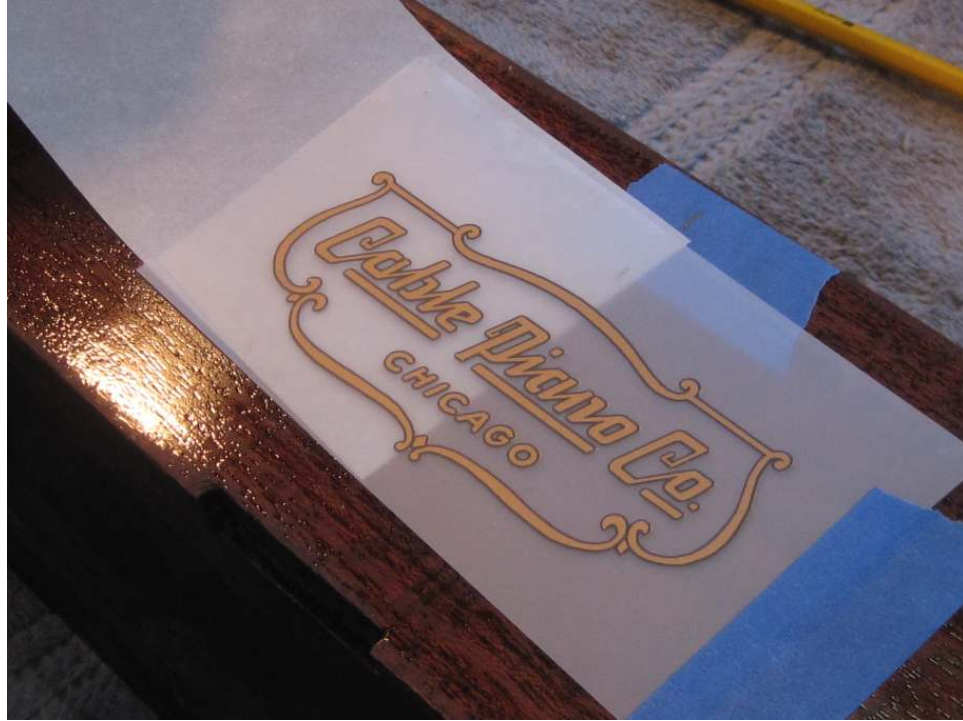
Photo 38: Once the decal is taped on the right hand side, the protective tissue is slid out. Only once have we actually burnished the decal to the tissue.
