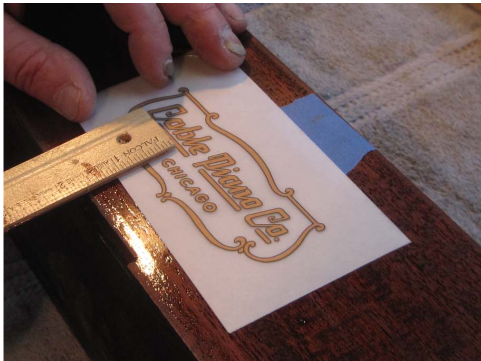
Photo 37: The decal is applied in between finish coats. Two coats of polyurethane have already been brushed on to the fallboard. After the decal is burnished in place, two more coats will be brushed over it. Here Dave locates the decal at the center of the fallboard. The pencil line on the blue masking tape marks the center of the fallboard from side-to-side.
