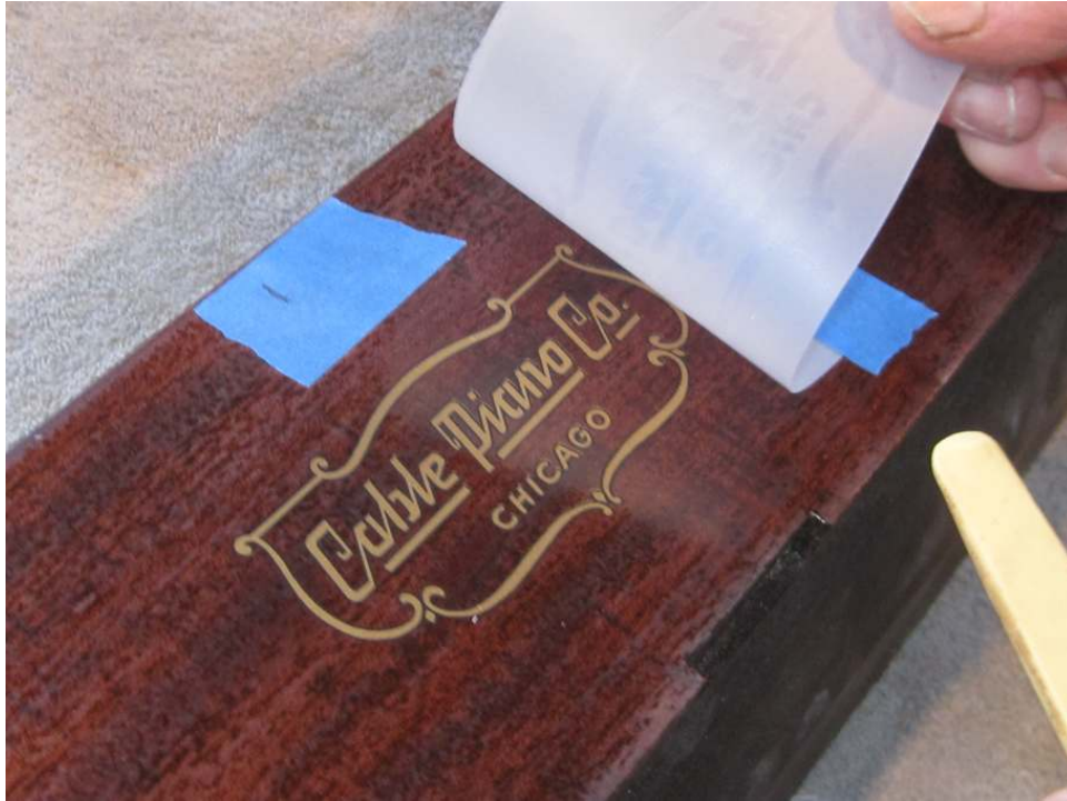
Photo 40: Dave lifts of the plastic sheet revealing the decal in place. (The slightly scuffed condition of the finish between coats improves adhesion.) Another coat of finish will be immediately applied to protect the new decal.
