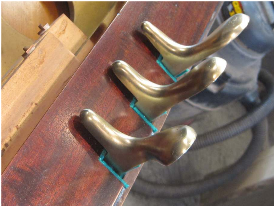
Photo 49: Pedals have been polished and lacquered. The floor of the piano and trapwork (after cleaning) has been reinstalled, along with the pedal rail with new felt. Things are starting to go back together.
