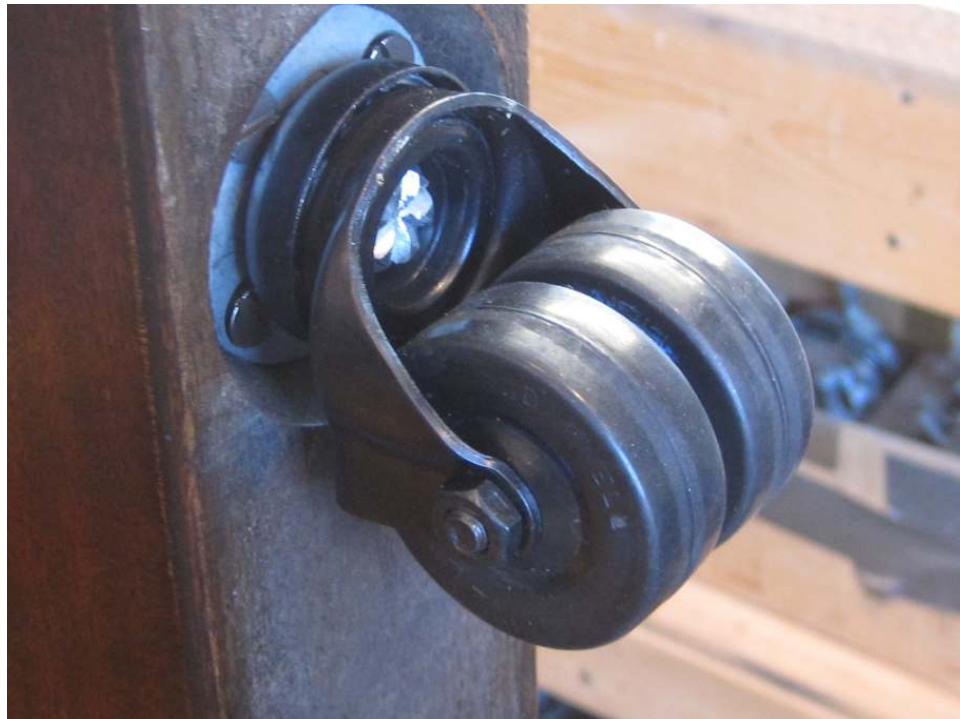
Photo 43: Time for new casters - top-of-the-line cast metal sockets and twin, rubber-fiber wheels are installed. These things are great – practically every upright that comes into our shop get a set. Rolling the piano around in the shop with these on is a breeze. Plus, these are just the thing for pianos going into homes with any kind of laminate flooring.
