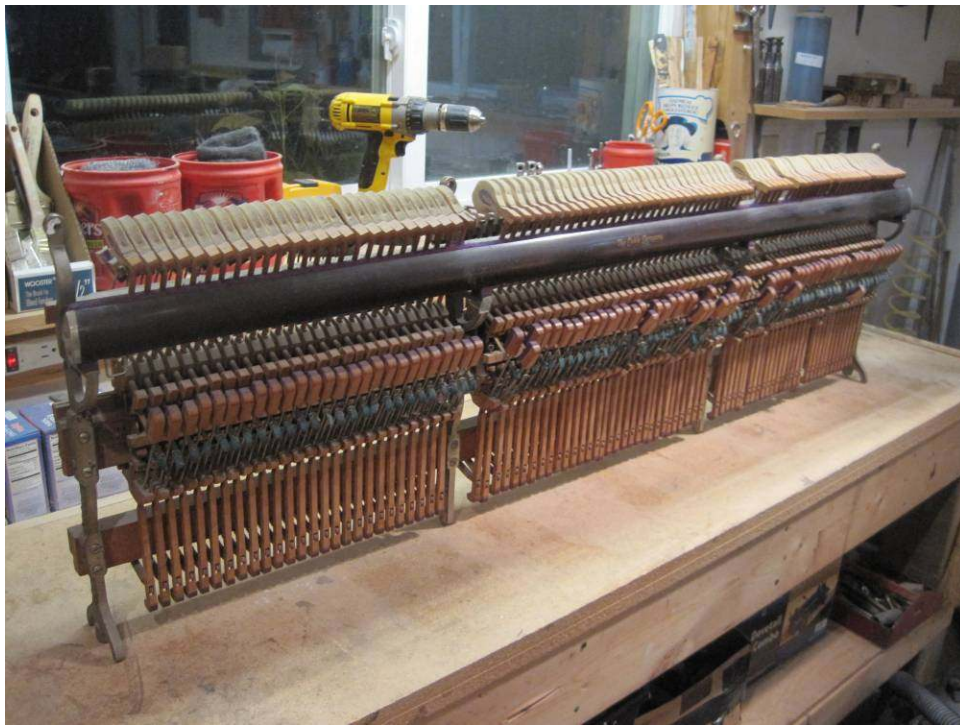
Photo 5: Piano action remove to bench for servicing
