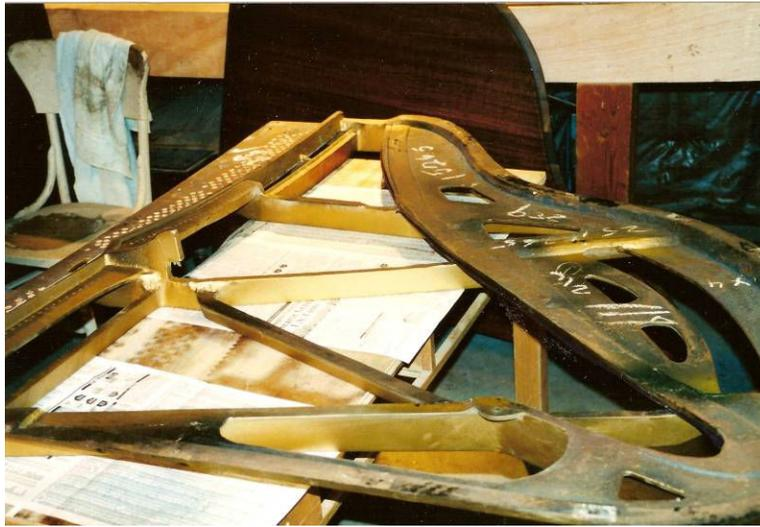
*Photo #4: Plate upside down for fitting the pinblock*
