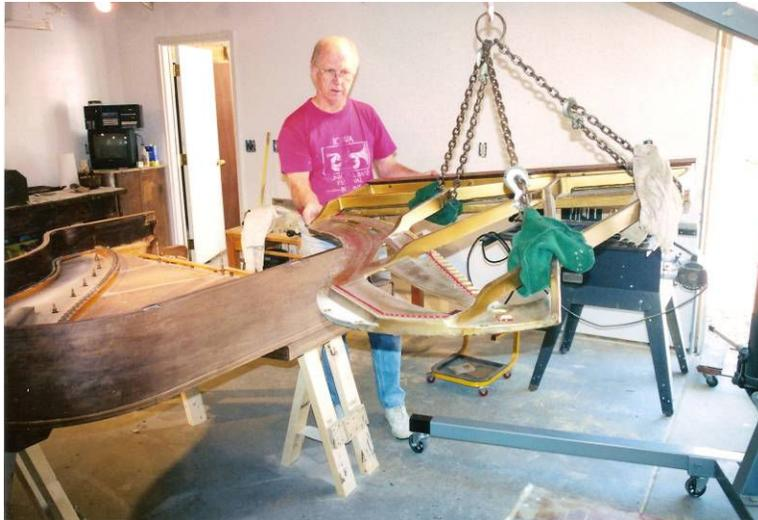
*Photo #6: Removing a plate with the engine puller*
