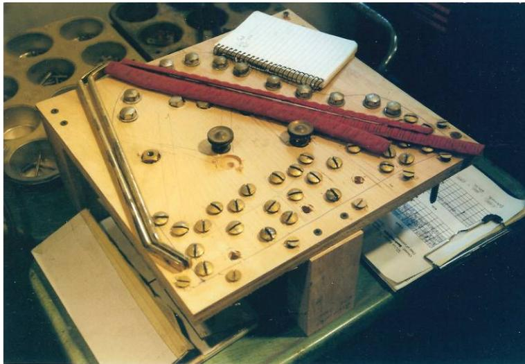
*Photo #2: Screw holder for a typical grand*
