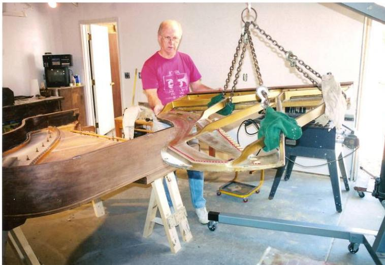
*Photo #6: Removing a plate with the engine puller*
