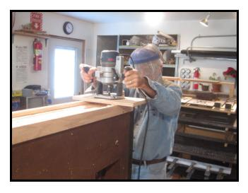
right) in order to give access to the back framework and pinblock. Once repairs have been accomplished, a new hardwood cap may be produced and installed—preferably with countersunk screws to allow access in the future.
