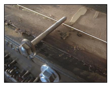
The photo left (taken during the repair of a separated back / pinblock assembly) illustrates the problem. The original lag screws (one of which is shown resting on top of the plate and pinblock) weren't able to hold things together once the glue joint failed. The white line shows where the pinblock ends and the back bracing begins. Obviously, the screws didn't
