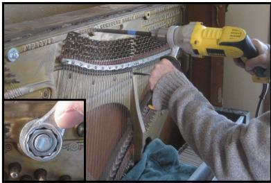
into the extended holes and the nuts are tightened down to apply permanent compression on the joint (inset).
