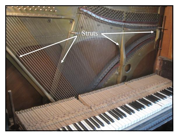
The cast iron plate revealed.
