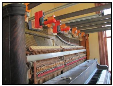
With this system the plate may be gently eased back into position. The crank on each clamp can be turned a fraction of a rotation at a time if necessary to apply pressure evenly from side to side. Once the gap has been closed sufficiently, the clamps may need to be left in place overnight (depending upon the adhesive used) to allow the glue to cure before proceeding.
