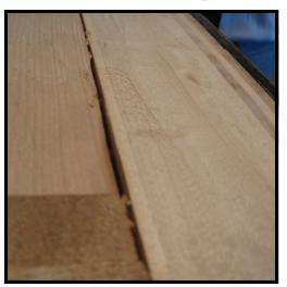
problem may begin. For anything greater than a simple hairline crack, the first step is to clean any debris out of the crack, block it open, then take the stress off the assembly by letting most of the tension off the strings. With the tension released, an adhesive is worked down into the crack. Finally, the gap is closed by using clamps to squeeze the assembly together.
