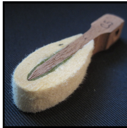
Same hammer after reshaping.
