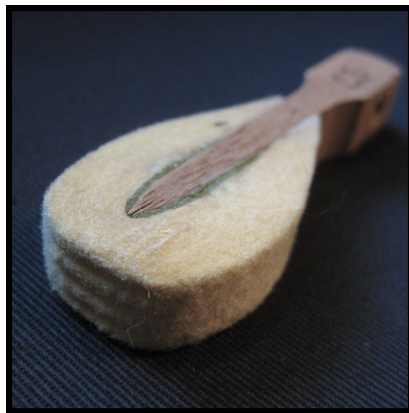
Hammer with significant wear.
