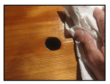
In addition to the soundboard, bridges are refinished as well (photo below). The sides and notches of the bridges are stripped and sanded, then shellacked. The top surface of the bridges (which must be slippery for strings to slide over easily) is coated with DAG, a product specifically designed for surfaces which must be friction-free.
