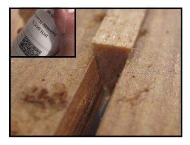
After the shims have been fitted, they are glued in place with a special glue with necessary acoustic properties (insert above). The shims are then weighted down and the glue is allowed to cure overnight.
