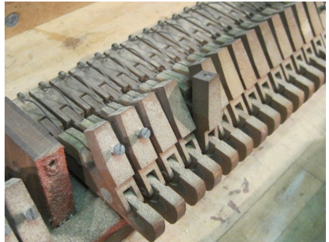
Photo 2: Added-on set screws.
