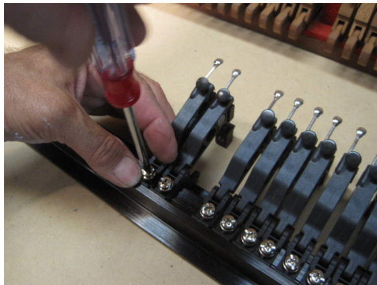
Photo 7: Screwing the damper levers down.
