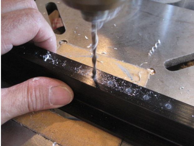
Photo 5: Drilling the flange screw holes
