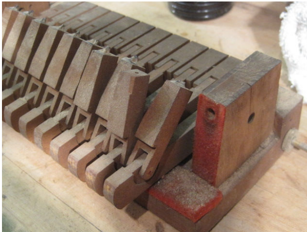
Photo 1: Epoxy collars on the tops of the damper blocks.
