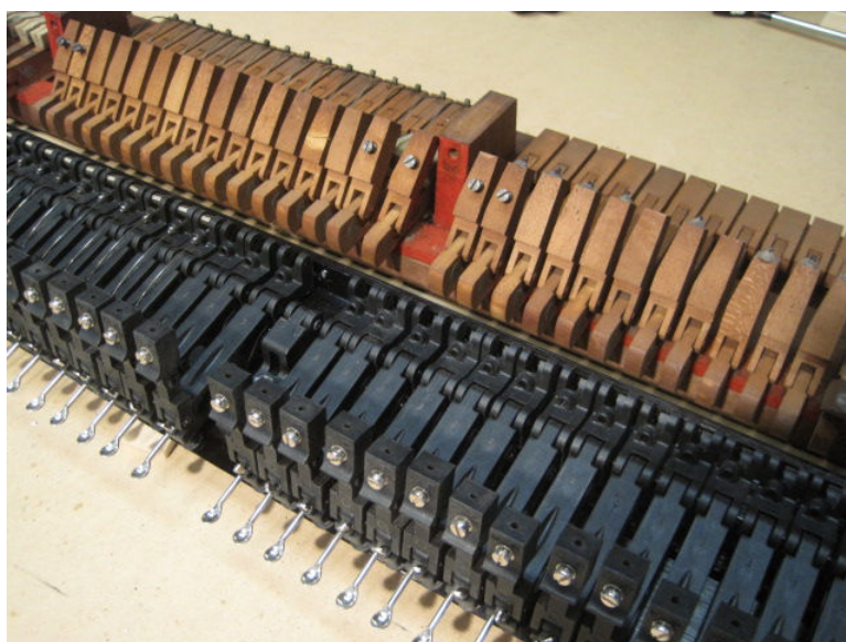
Photo 8: New back action compared to old.
