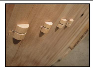
As the wires are tightened, glue will squeeze out from the areas being joined (below photo), indicating that the fit is tight and the bond will be secure. The excess glue is carefully cleaned from the edges before it dries.
