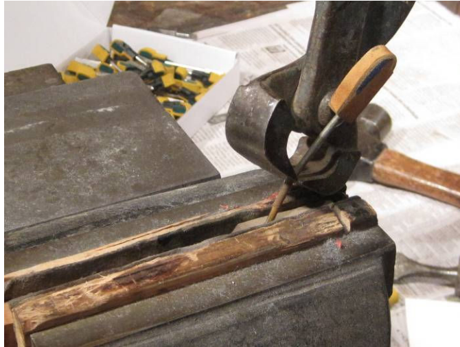
Photo 9: Removing the old wires.
