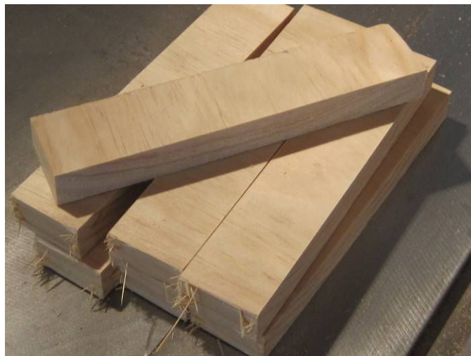
Photo 10: Material for risers, planed to thickness.
