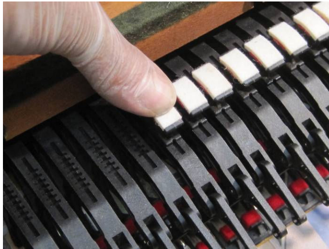
Photo 3: Gluing the heels.
