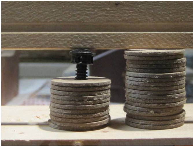
Photo 8: The stack of punchings with and without capstan.
