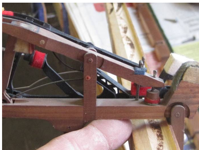
Photo 6: Much better alignment after trimming the rail.
