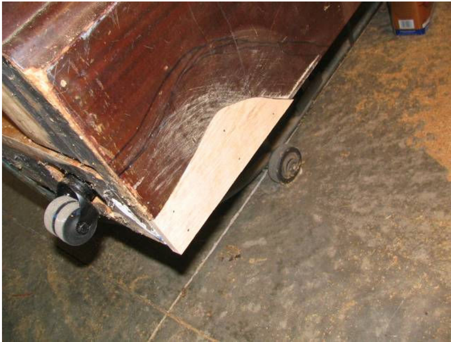
Photo 2: Glued in place, with finishing nails in lieu of clamps
