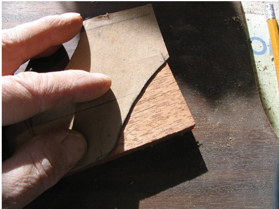
Photo 5: Transfer the shape to the new stock
