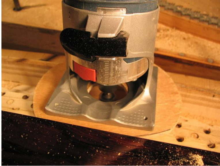
Photo 6: Small Bosch router with added base plate.
