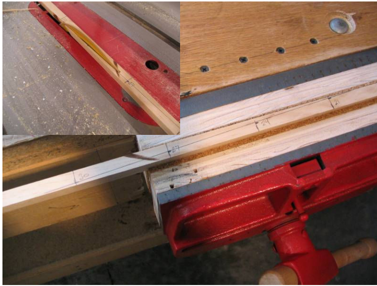
Photo 2: Adjustment strip marked for cutting.
