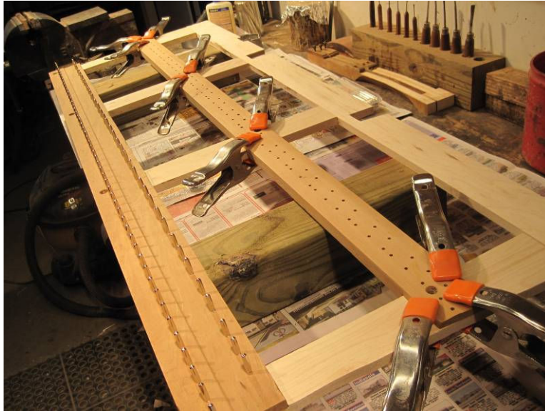
Photo 2: Balance rail is clamped into place.
