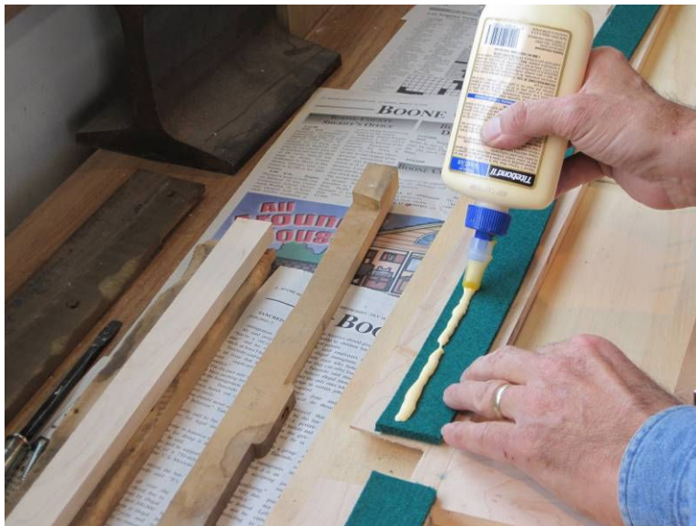
Photo 7: Gluing the back rail cloth.
