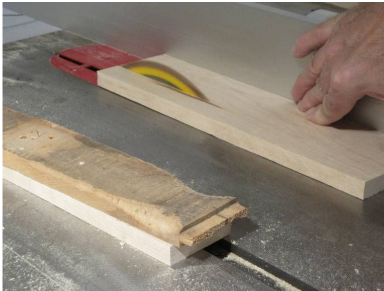
Photo 9: Ripping to width.
