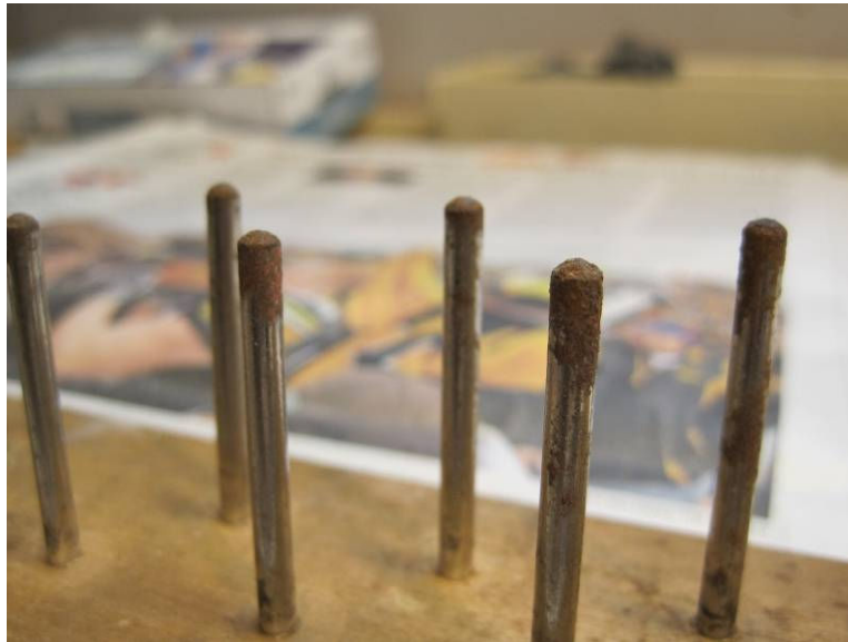
Photo 1: Corrosion which was more than skin-deep.
