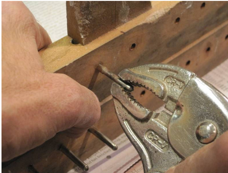
Photo 6: Pulling out the front rail pins.
