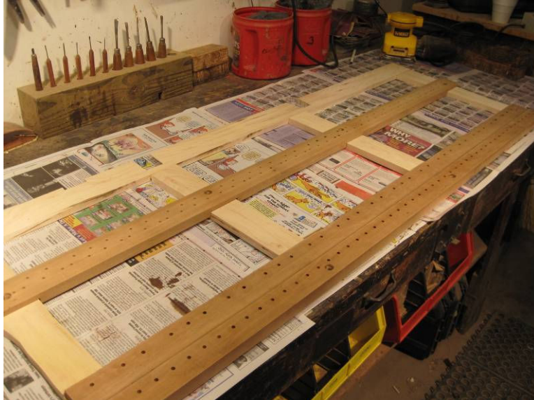
Photo 13: Balance rail is installed.
