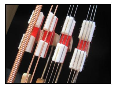
The four most commonly used upright dampers are shown in the photo above. The powerful vibration of the longest of the copper wound bass strings (far left in photo) are quieted by single wedge dampers. For the lighter pairs of wound bass strings found further up on the scale, double wedge dampers are used. Plain steel treble strings are either dampened with trichord dampers or flat dampers.
