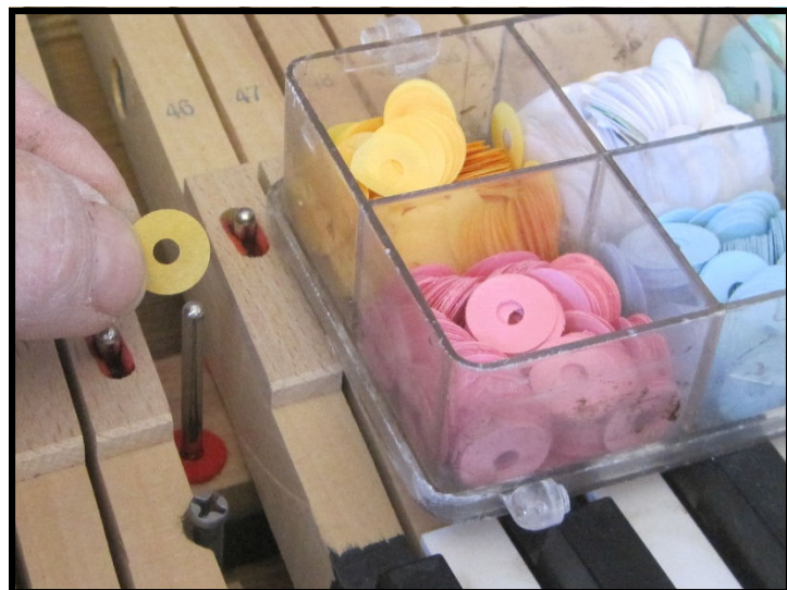
.002" paper punching being installed
